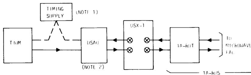
A. TERMINATING ARRANGEMENT WITH 1A-RDT IN HUB OFFICE
