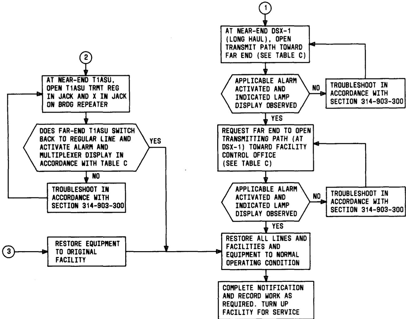
Fig. 4—Facility Alarm Verification Test (Sheet 2 of 2)
