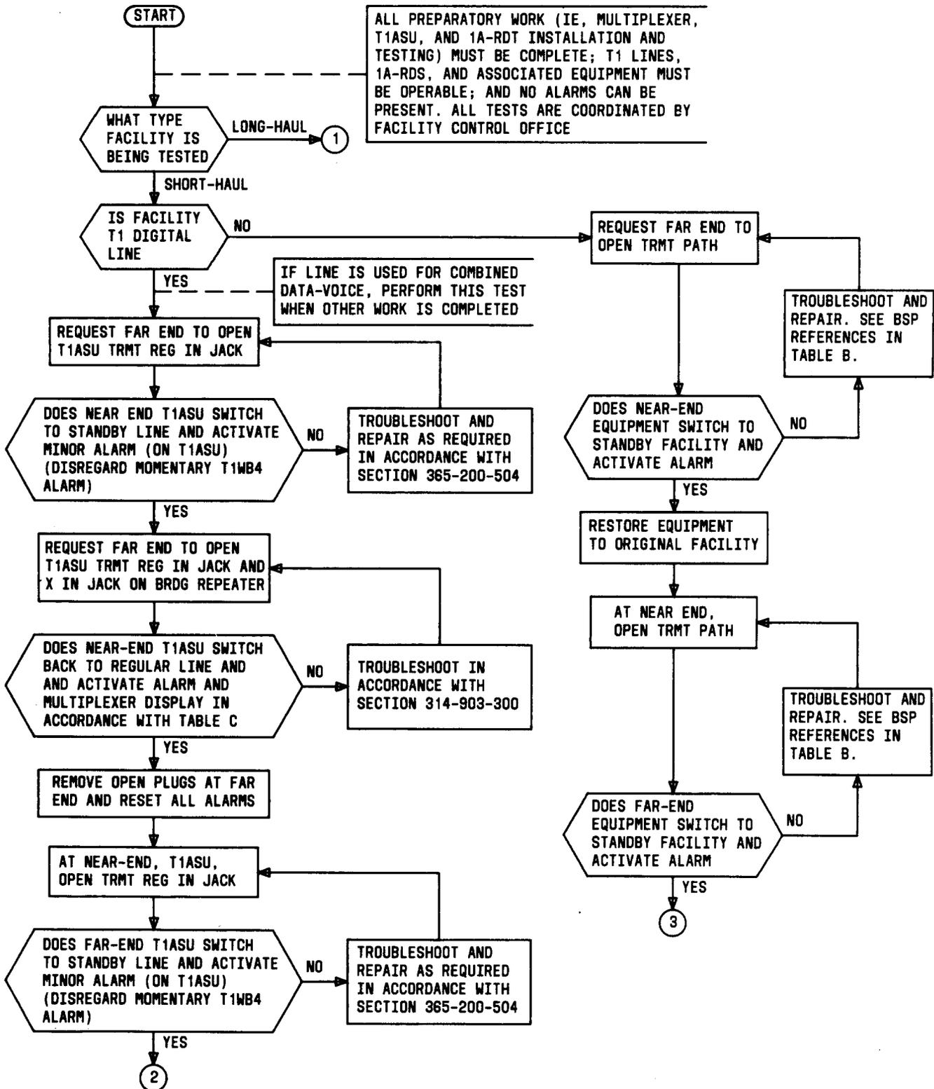
Fig. 4—Facility Alarm Verification Test (Sheet 1 of 2)
