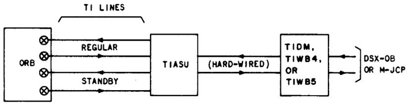
A. TYPICAL CROSS-CONNECTION FOR TI LINE WITHOUT DSX-1
