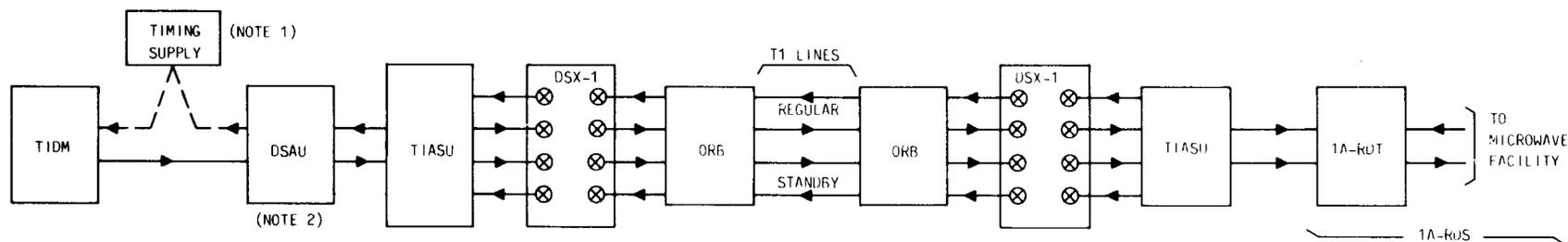
B. TERMINATING ARRANGEMENT WHEN T1 LINE IS USED FOR CONNECTING HUB OFFICE WITH 1A-RDS TERMINAL IN ANOTHER OFFICE.
