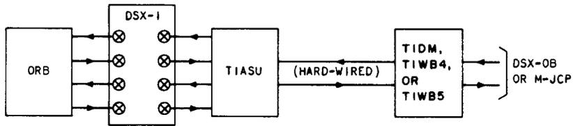
B. TYPICAL CROSS-CONNECTION FOR TI LINE WITH DSX-1
