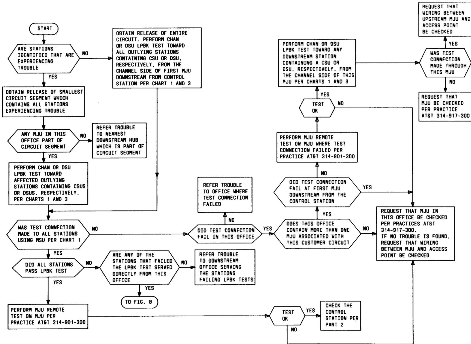
Fig. 7—Hub Trouble Isolation Procedures for a Multipoint Circuit (Sheet 1 of 2)
