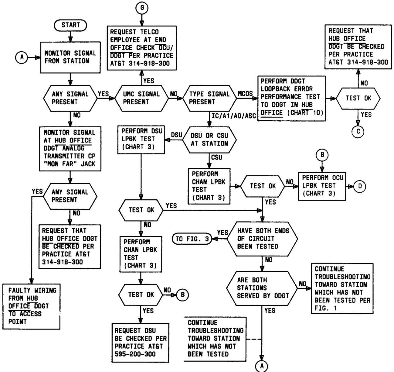
Fig. 5—Trouble Isolation Procedures for Stations Served by DDGT (Sheet 1 of 2)
