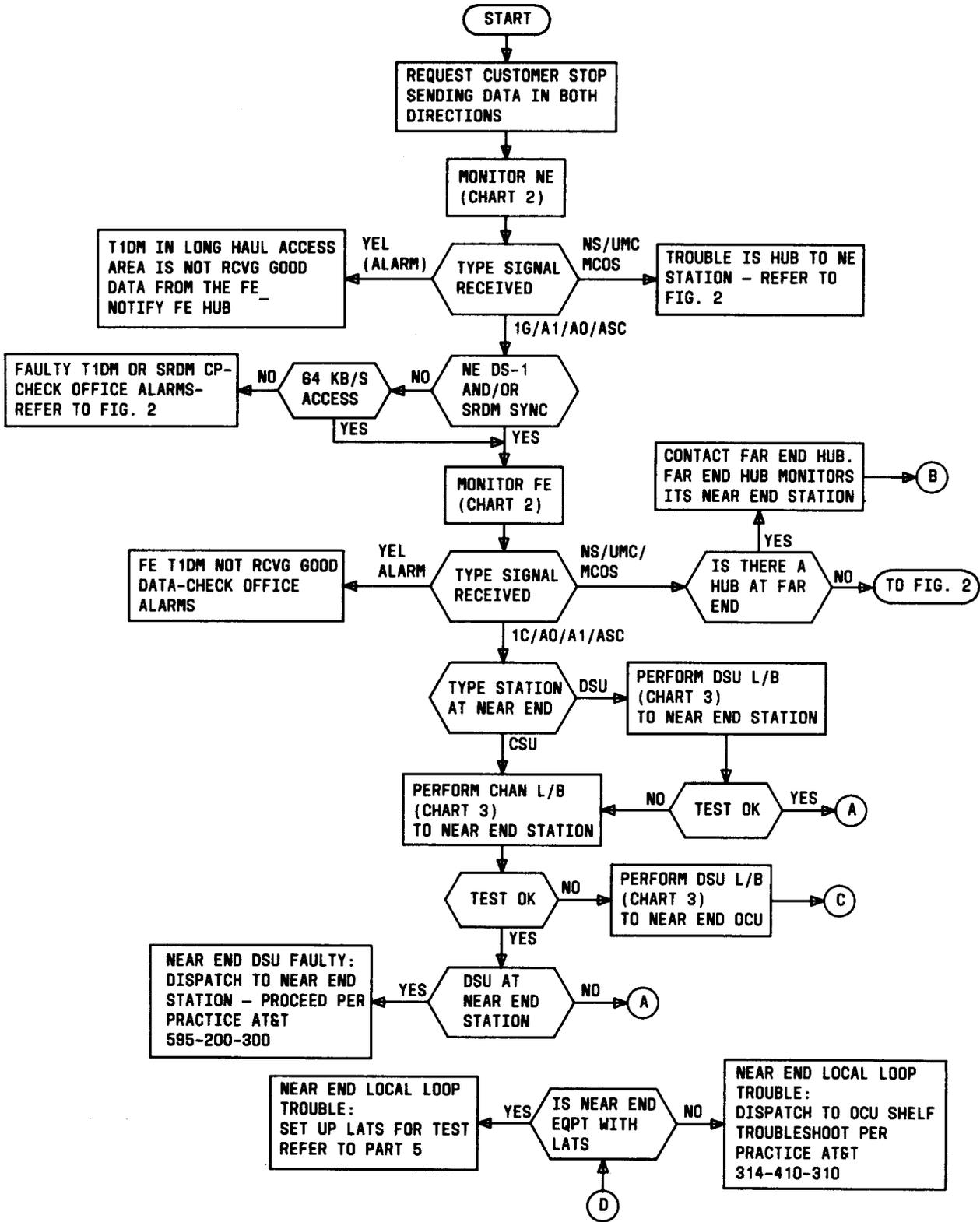
Fig. 1—Preliminary Hub Trouble Isolation Procedures (Sheet 1 of 3)
