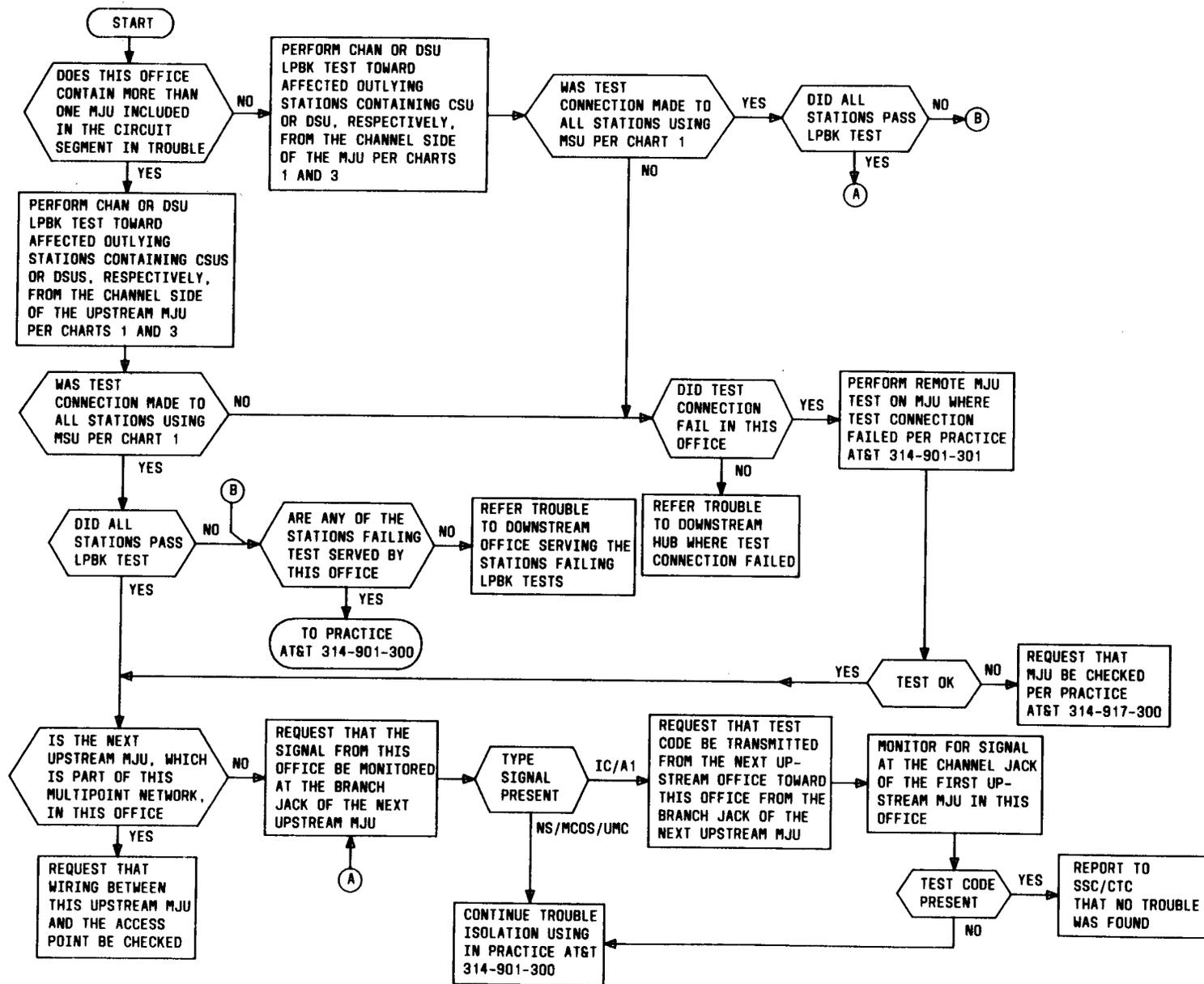
Fig. 7—Hub Trouble Isolation Procedures for a Multipoint Circuit (Sheet 2 of 2)
