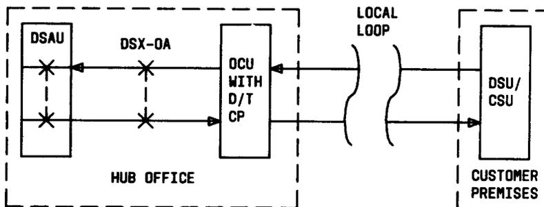
Fig. 2—Hub to OCU Circuit Analysis
