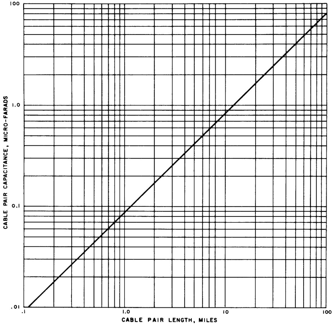
Fig. 12—Capacitance/Mileage Nemograph
