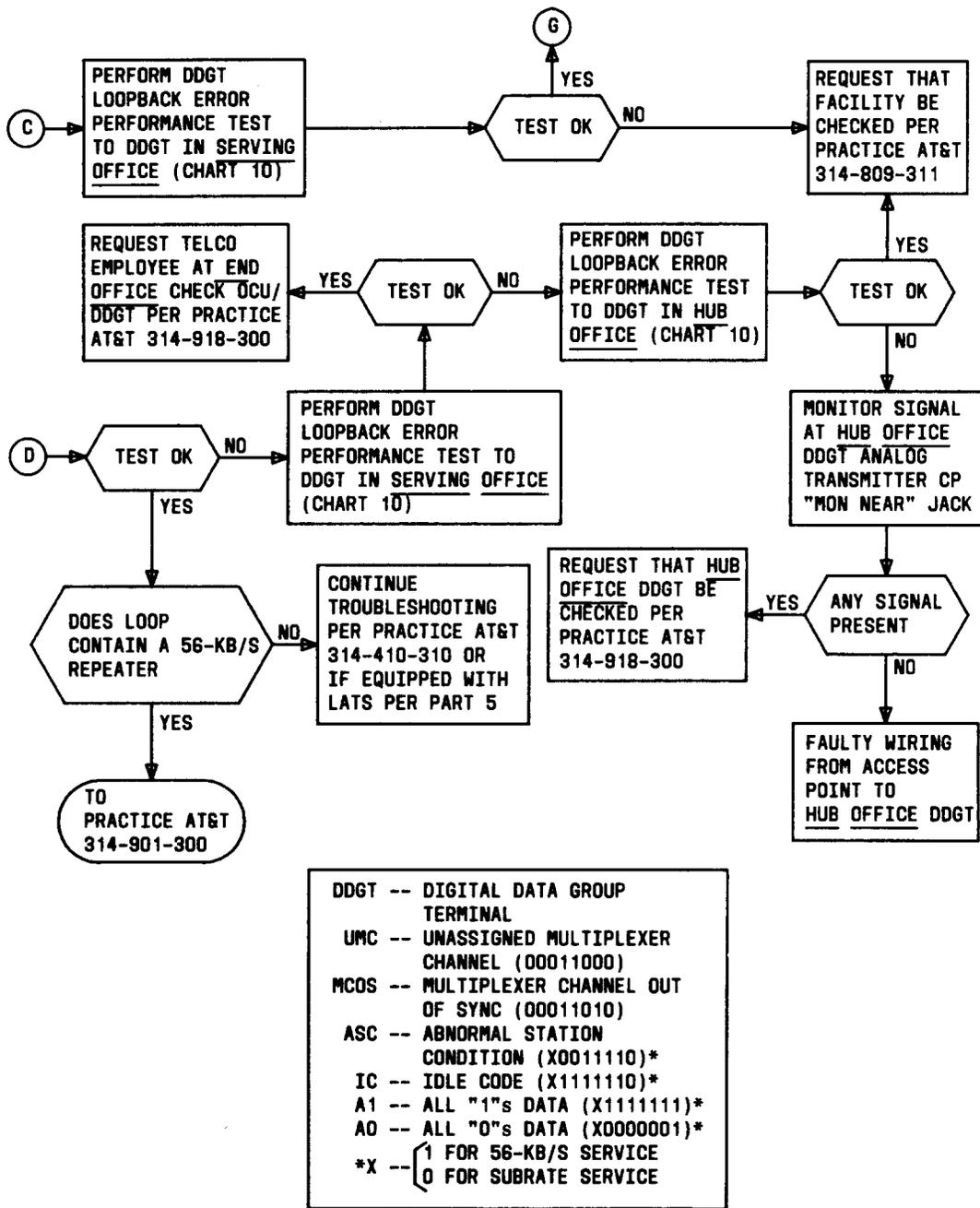
Fig. 5—Trouble Isolation Procedures for Stations Served by DDGT (Sheet 2 of 2)
