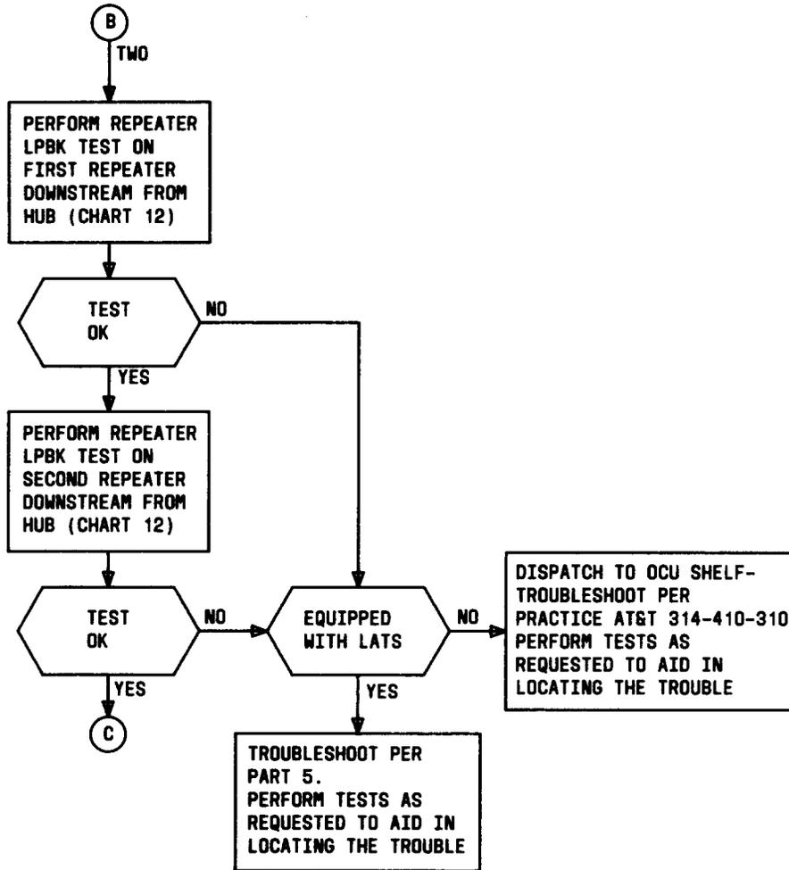
Fig. 4—Trouble Isolation Procedures for Loop Containing 56-kb/s Repeater (Sheet 2 of 2)
