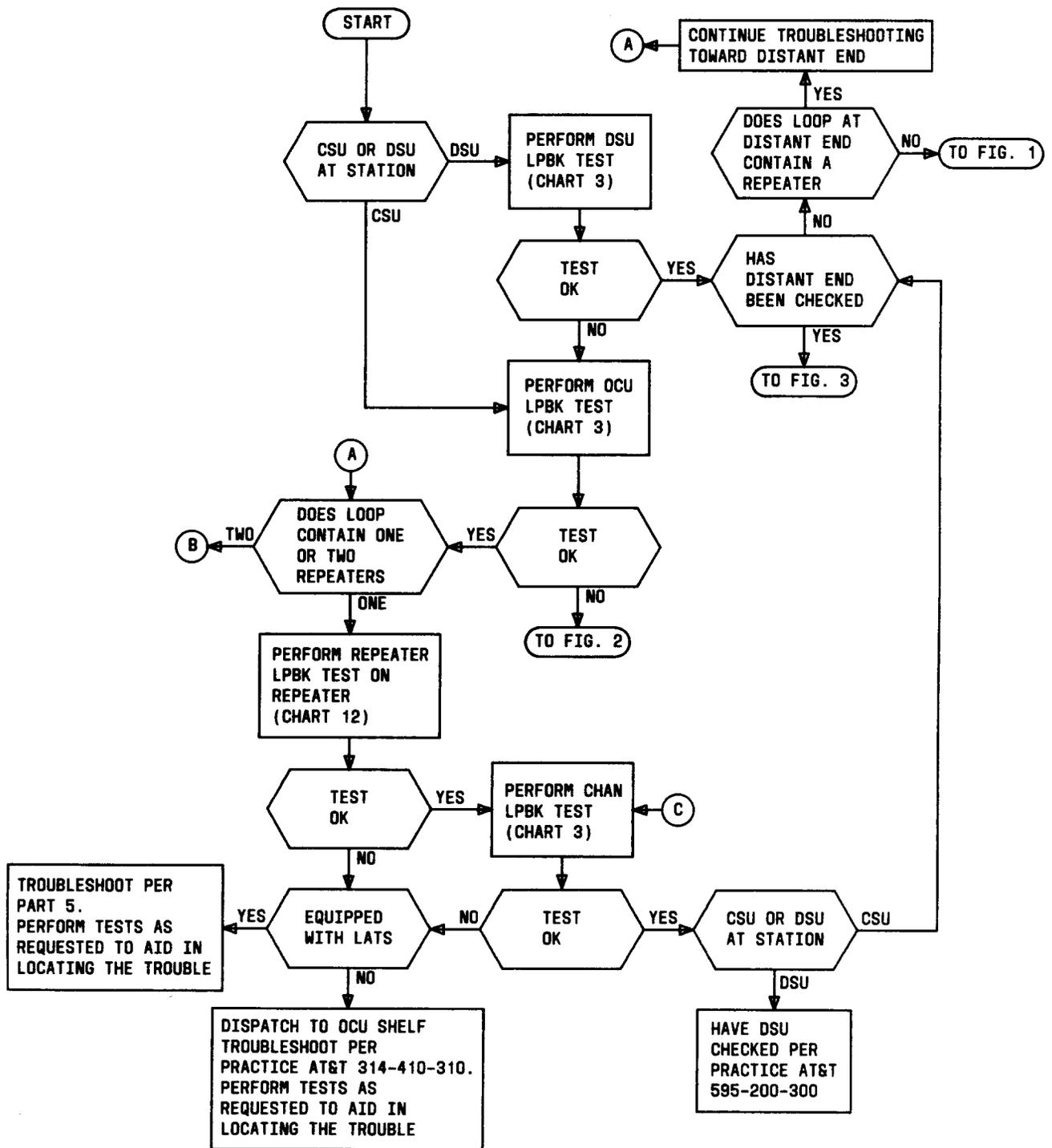
Fig. 4—Trouble Isolation Procedures for Loop Containing 56-kb/s Repeater (Sheet 1 of 2)
