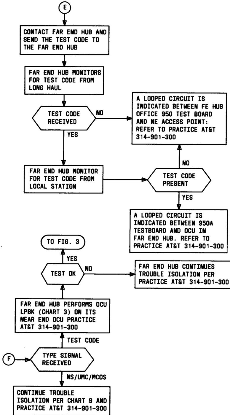
Fig. 1—Preliminary Hub Trouble Isolation Procedures (Sheet 3 of 3)
