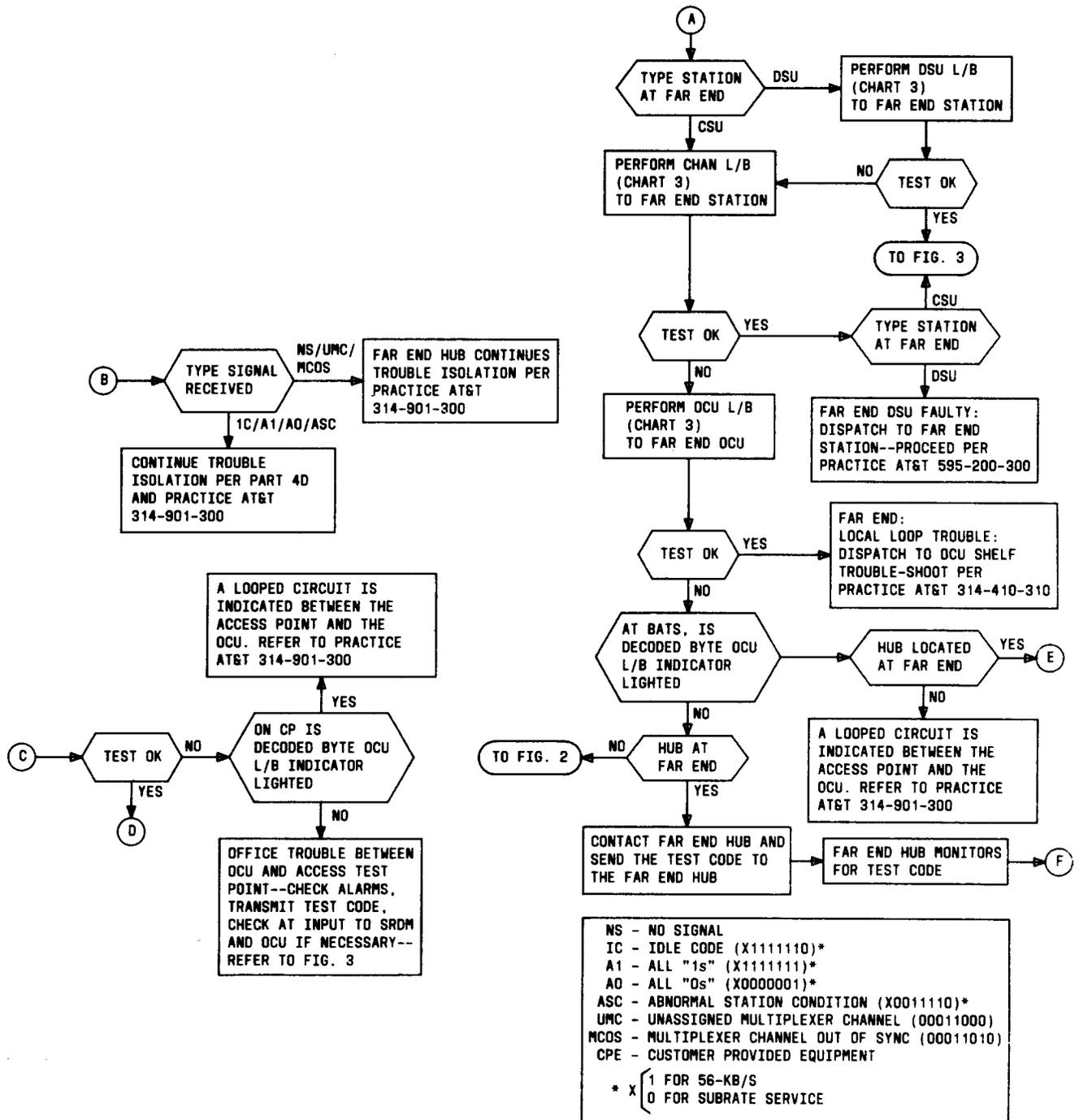
Fig. 1—Preliminary Hub Trouble Isolation Procedures (Sheet 2 of 3)
