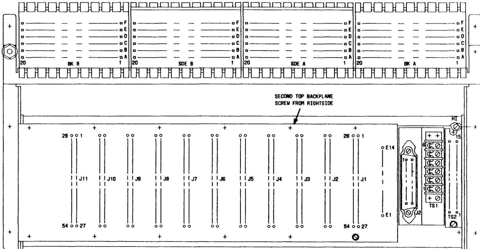
Fig. 2 - Rear View of Clock Distribution Unit (J98726Z-1)
