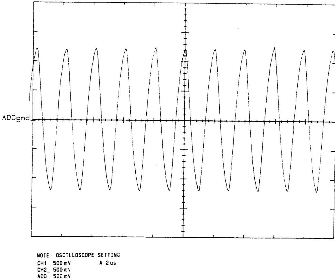
Fig. 17b - 512-kHz AHG4 Output Waveform
