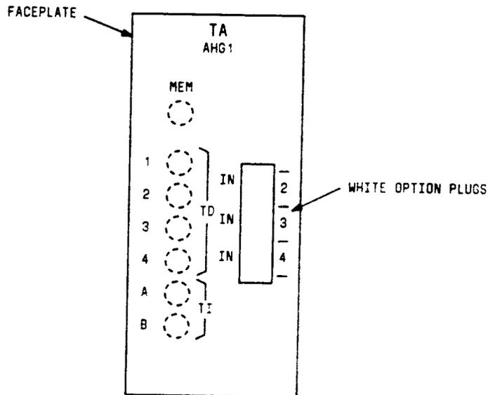
Fig. 23 - Location of Options for the AHG1 Timing Alarm
