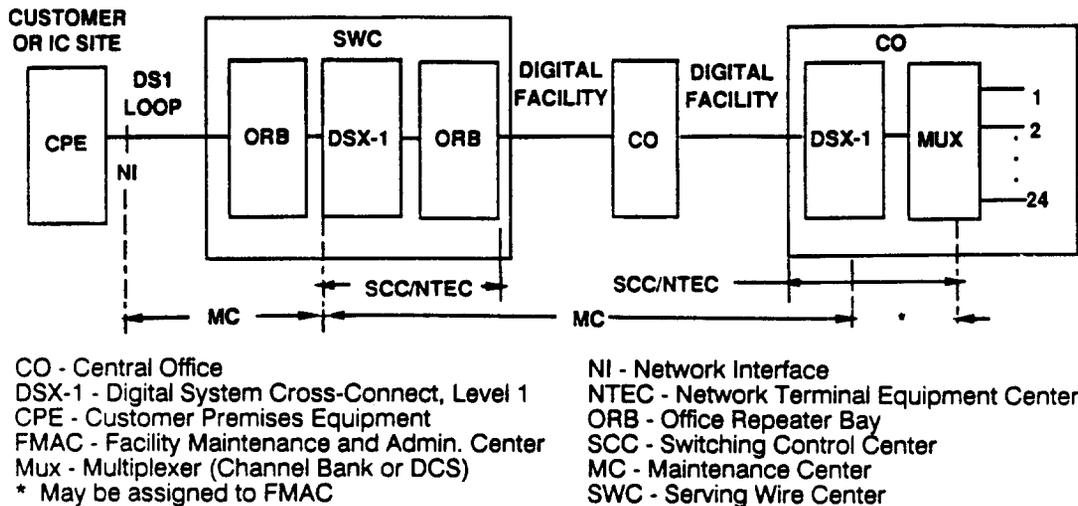
Fig. 2 - CO Multiplexer and Operations-Center Repair Responsibilities
