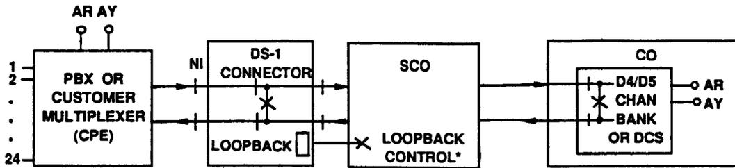
\*Loopback controlled from office that has circuit control.
