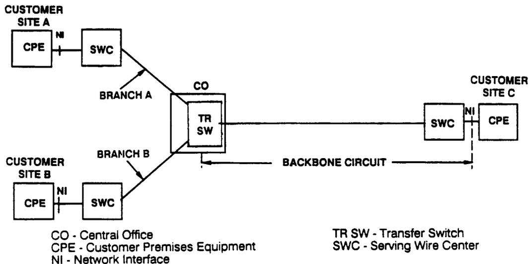
Fig. 3 - Transfer Arrangement
