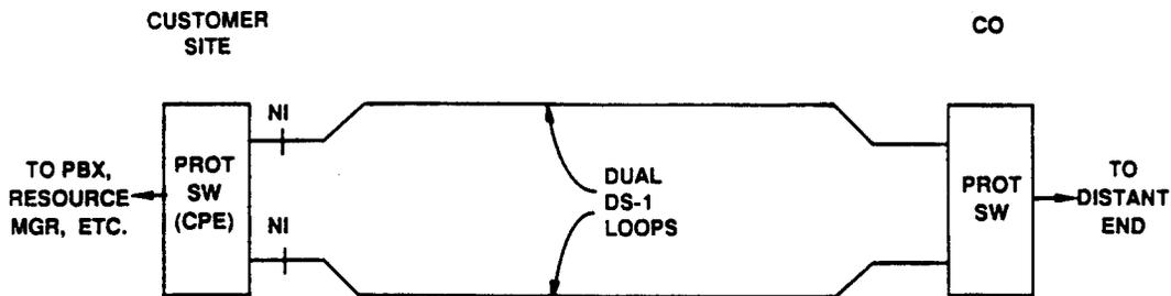
Fig. 4 - DS-1 Service with Automatic Protection Switching
