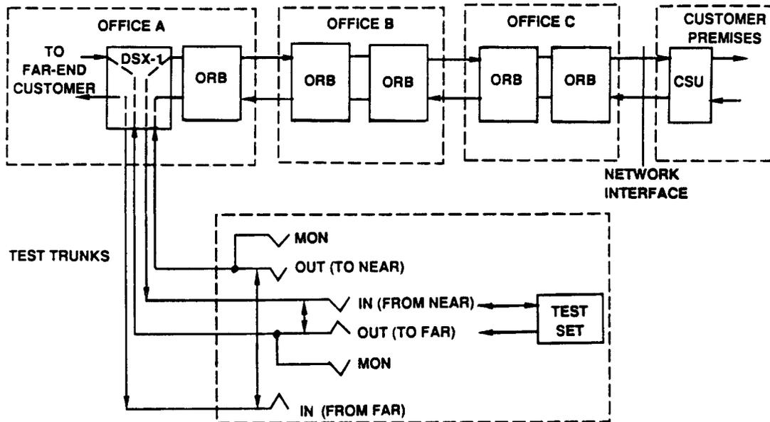
Fig. 7 - DS-1 Circuit, Patched for Testing
