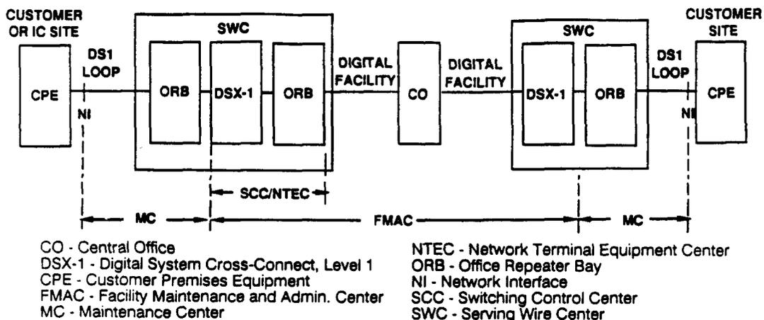
Fig. 1 - Circuit Routing and Operations-Center Repair Responsibilities
