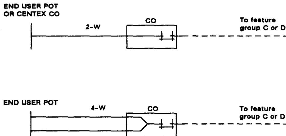
Fig. 16 - Typical WATS Access Line Configuration
