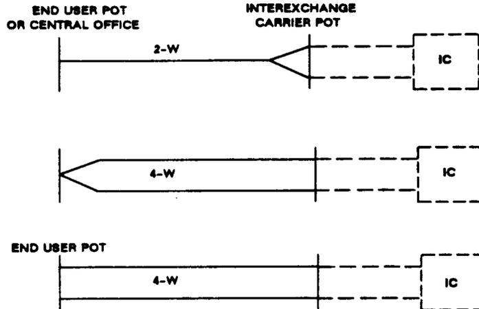
Fig. 4 - Typical Voice-Grade 2 Channel Configurations
