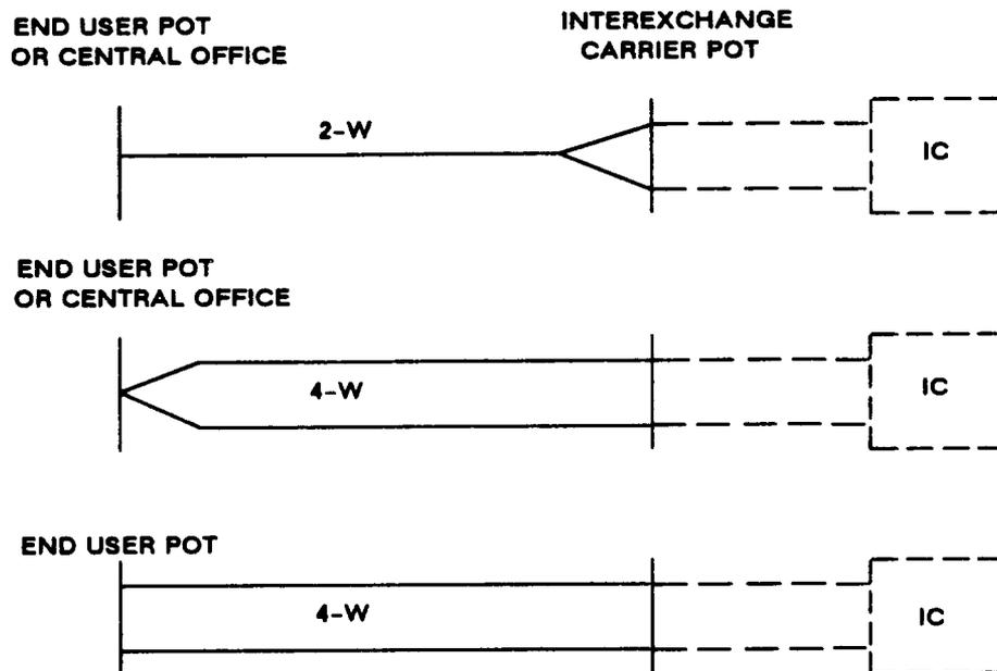
Fig. 5 - Typical Voice Grade 3 Channel Configurations
