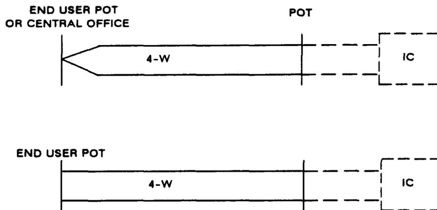
Fig. 10 - Typical Voice-Grade 8 Channel Configurations
