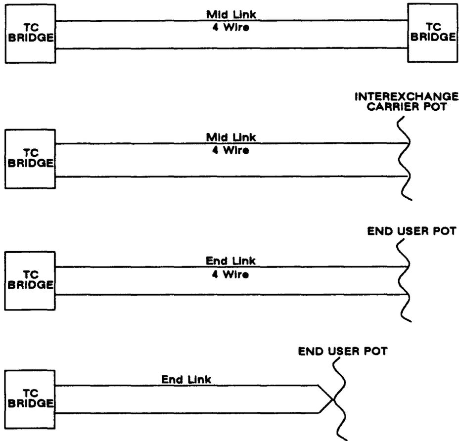
Fig. 2A - Typical Effective 4-Wire Multipoint Configurations
