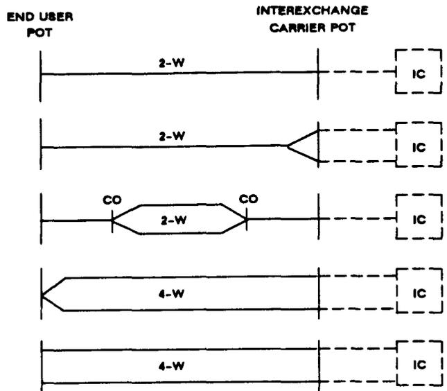
Fig. 3 - Typical Voice-Grade 1 Channel Configurations
