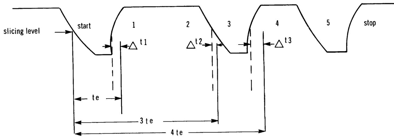
Fig. 2—Distorted Five Level Telegraph Start-Stop Signal
