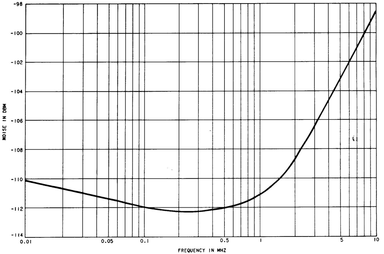
Fig. 8—3A/4A FM Terminal Pair Fluctuation Noise (Without Pre-Emphasis)
