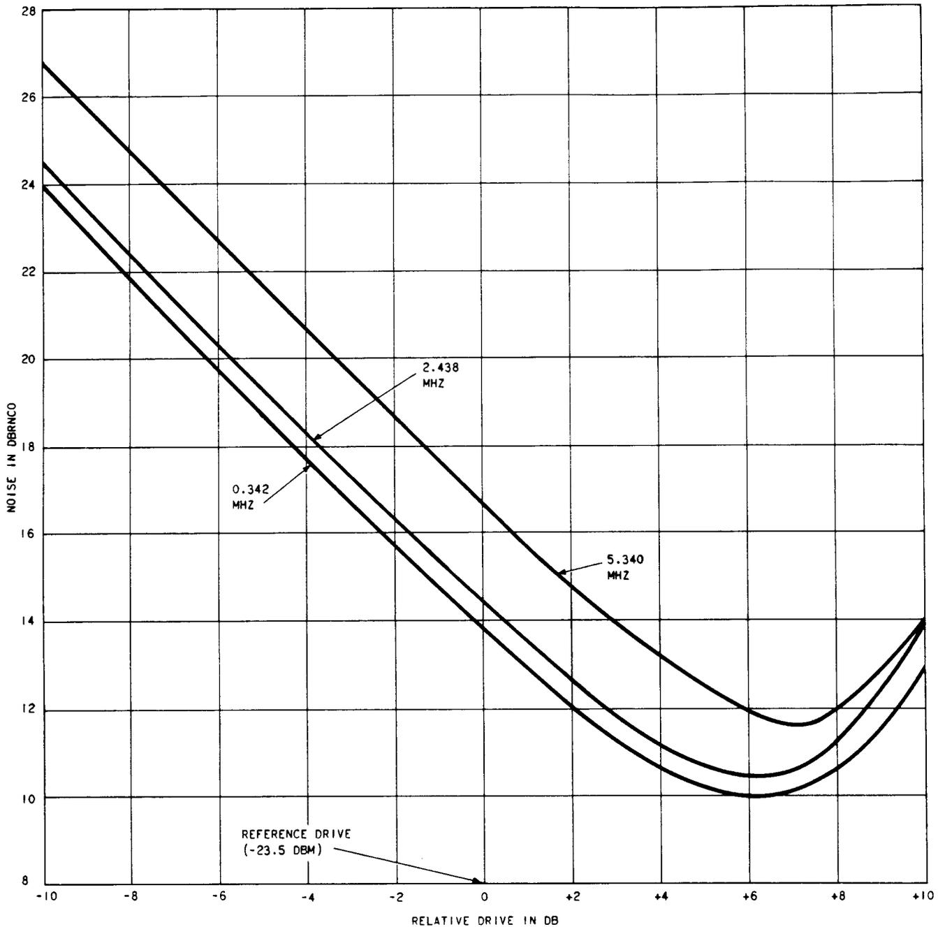
Fig. 4—Typical 3A/4A FM Terminal Pair 1200-Circuit Noise Load Curves (With 457D and 457E Networks)
