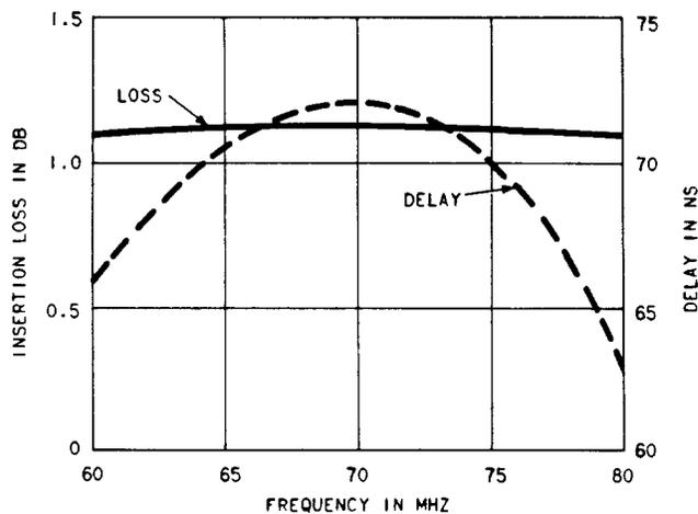
Fig. 3—4167A Network Delay and Insertion Loss
