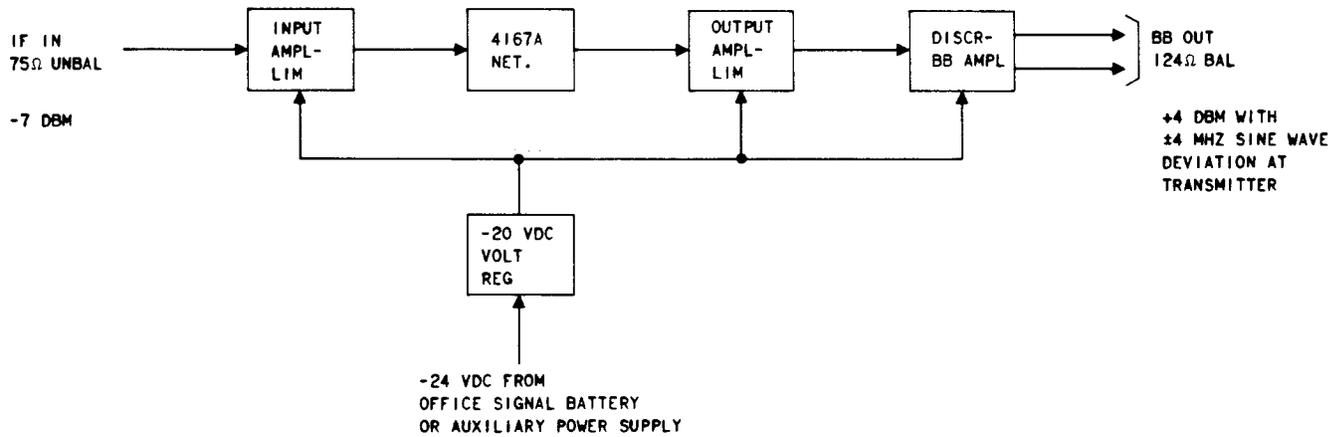
Fig. 2—4A FM Terminal Receiver Block Diagram
