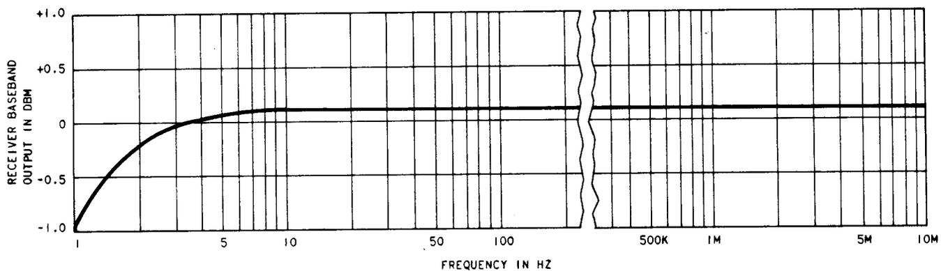
Fig. 7—3A/4A FM Terminal Pair Baseband Response
