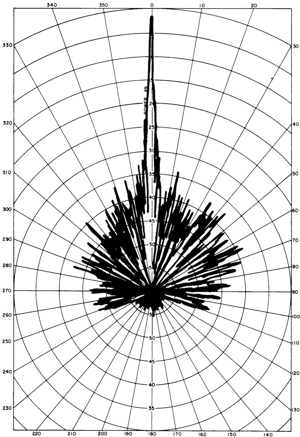
Fig. 5—Radiation Pattern for Horizontally Polarized 11.2 GHz Signal
