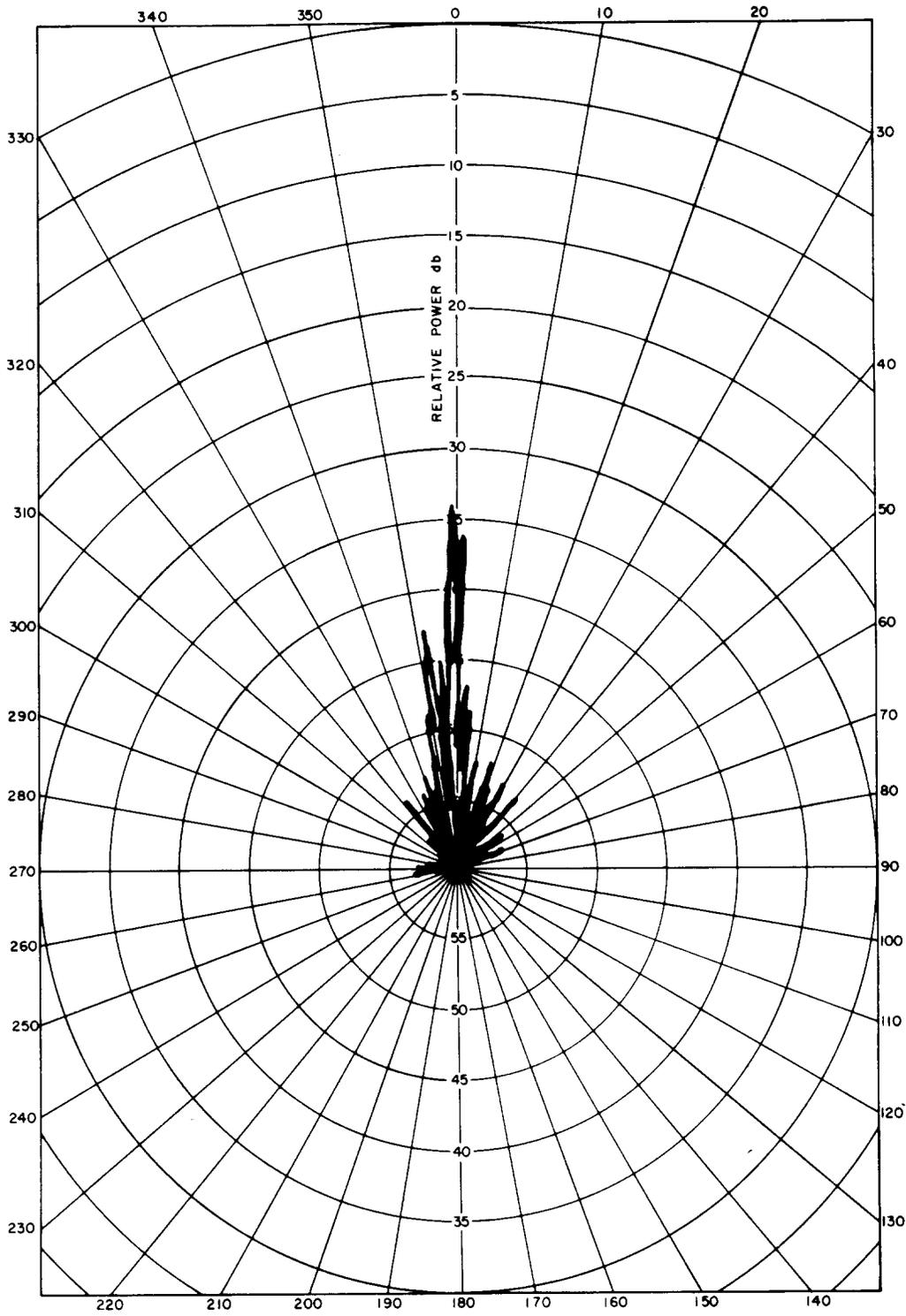
Fig. 8—Response to a Cross-Polarized 11.2 GHz Signal
