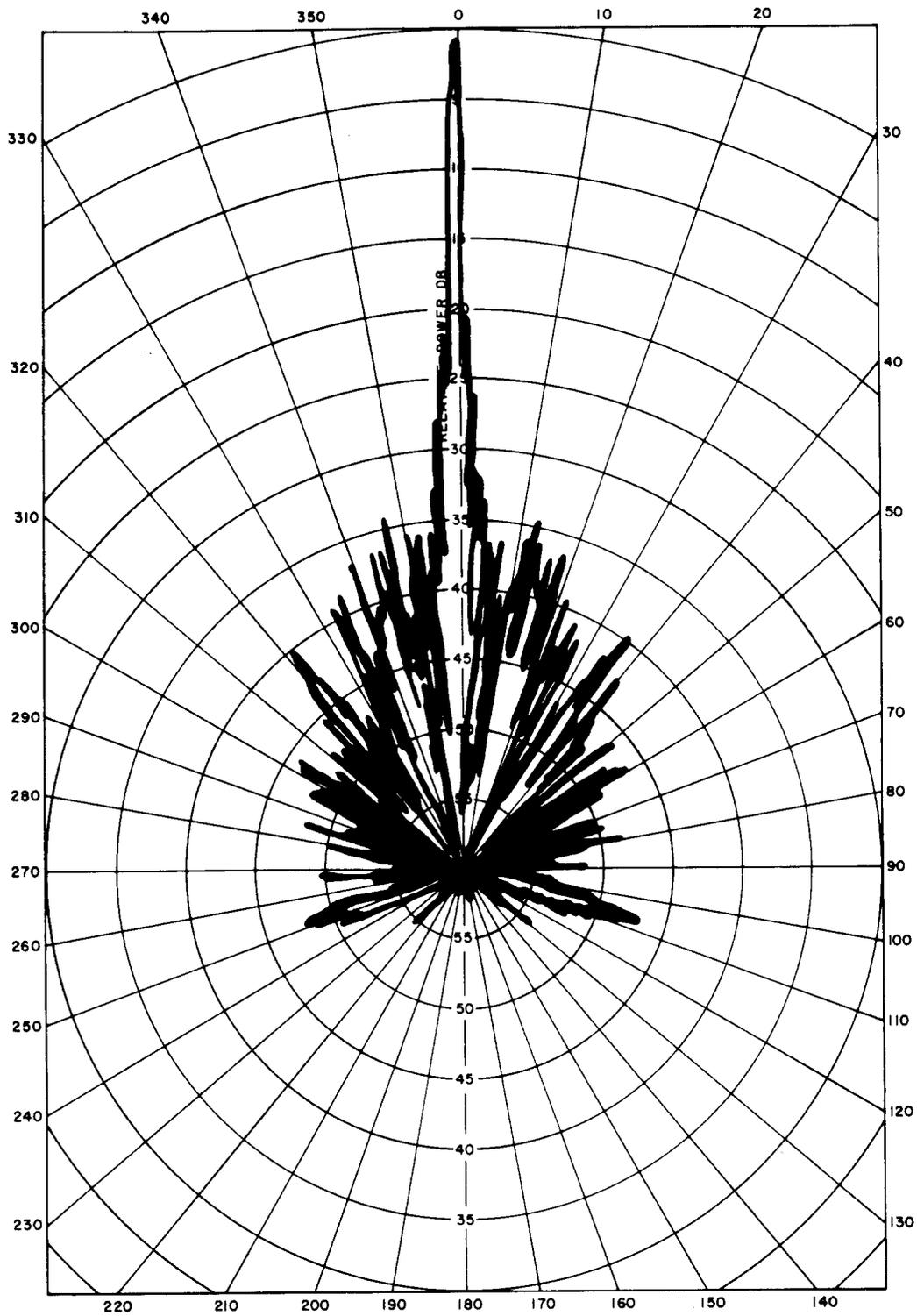
Fig. 6—Radiation Pattern for Vertically Polarized 11.2 GHz Signal
