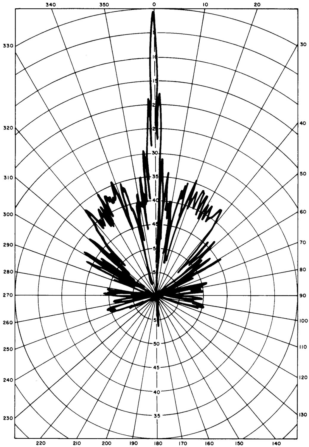
Fig. 3—Radiation Pattern for Horizontally Polarized 6.175 GHz Signal
