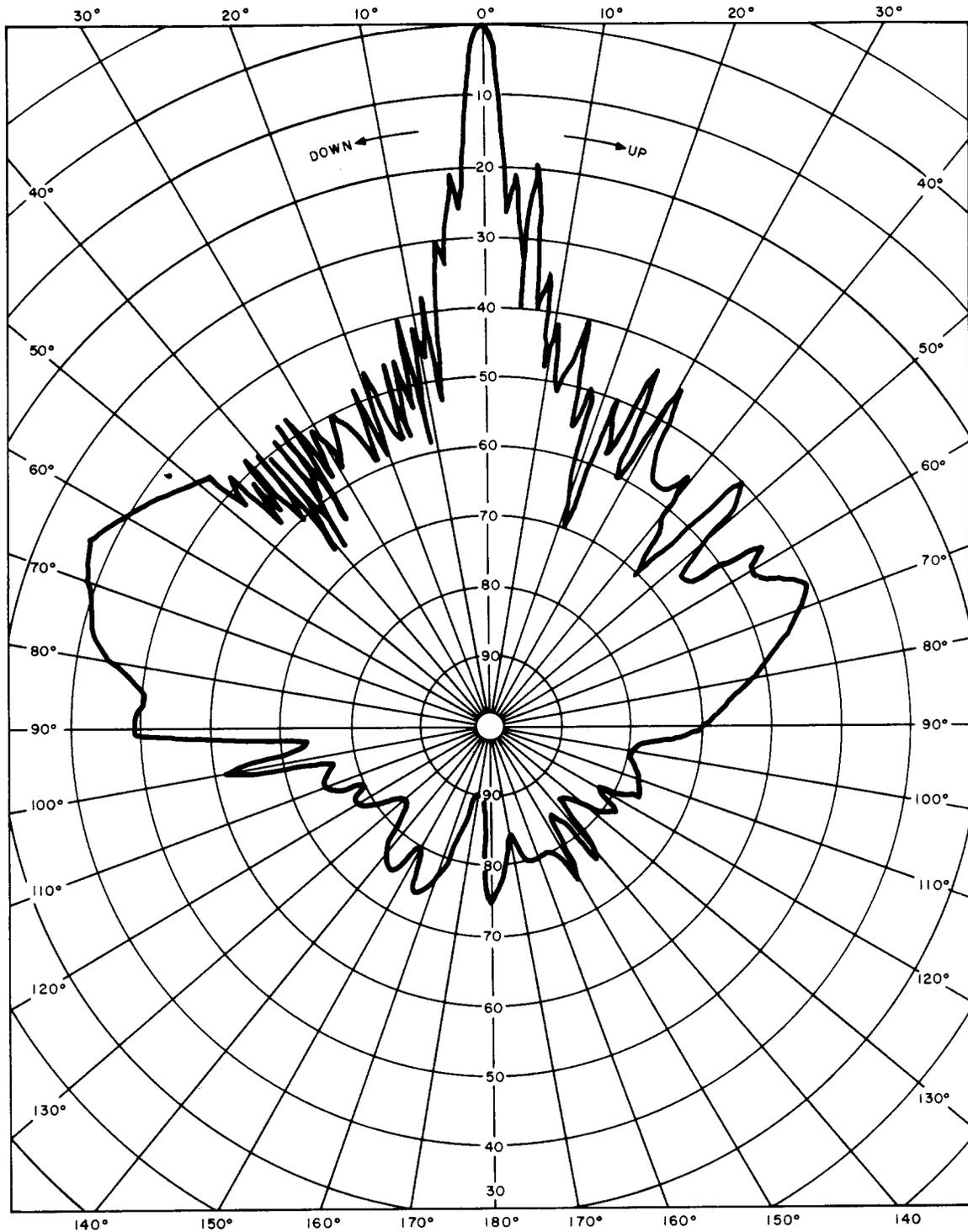
Fig. 14—Vertical Directivity—Horizontal Polarization—3740 MHz (360 Degrees)
