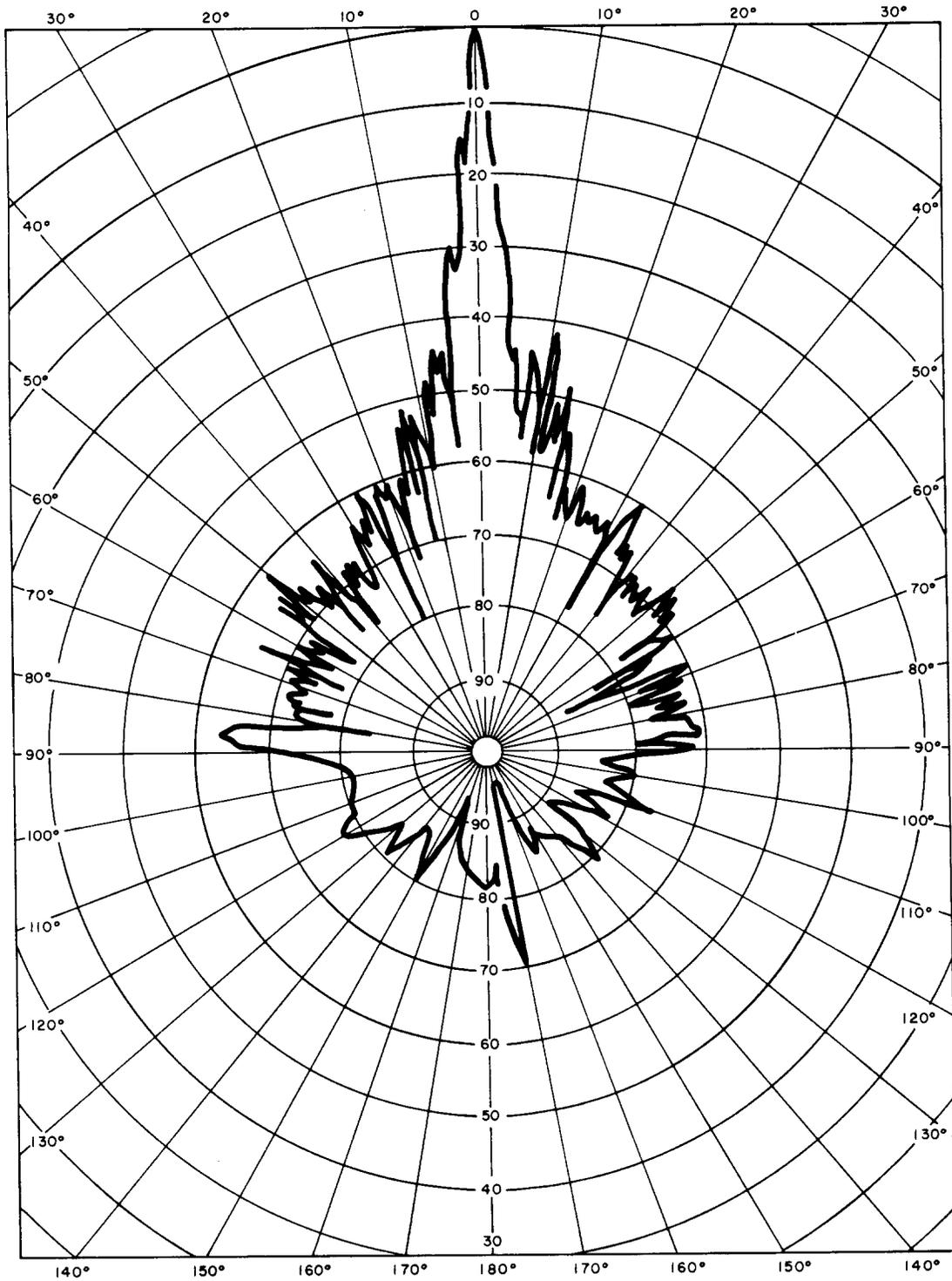
Fig. 12—Horizontal Directivity—Horizontal Polarization—10,960 MHz (360 Degrees)
