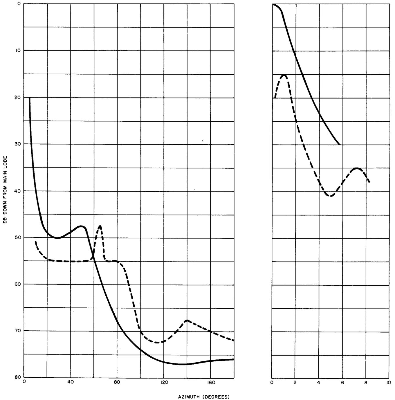
Fig. 22—Smoothed Horizontal Directivity—Vertical Polarization—6 GHz
