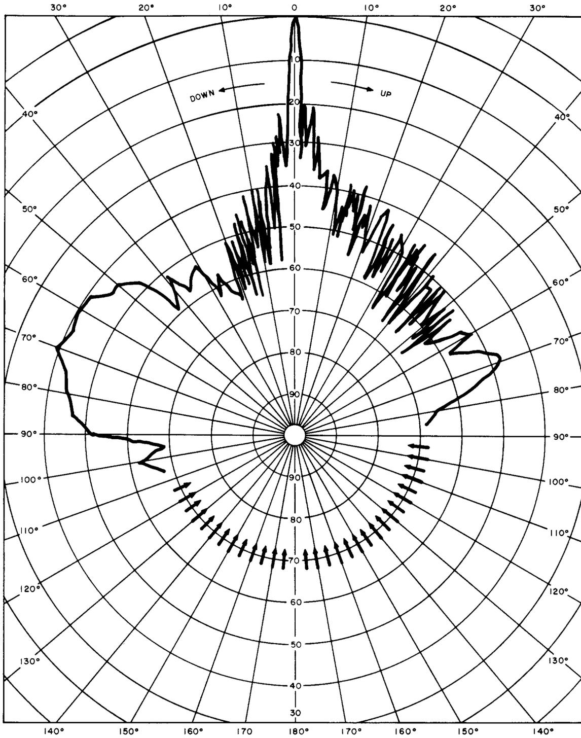
Fig. 16—Vertical Directivity—Vertical Polarization—10,960 MHz (360 Degrees)
