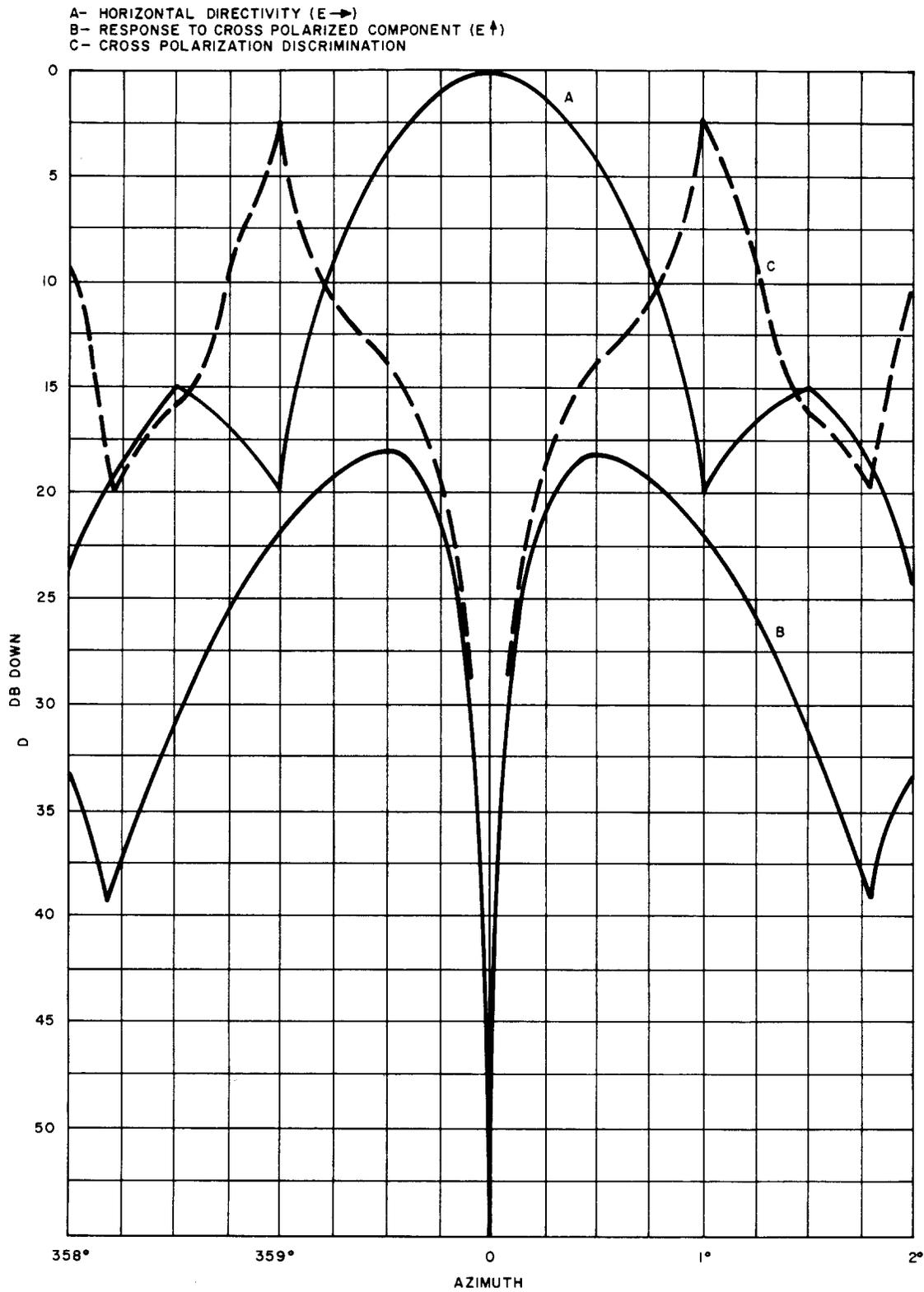
Fig. 5—Horizontal Polarization—Cross-Polarization Discrimination with Azimuth ( $\pm 2$  degrees)—10.960 MHz
