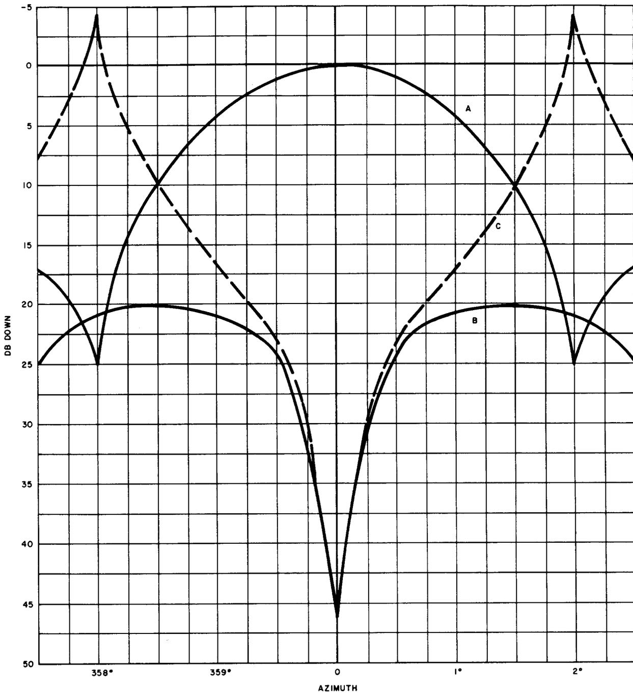
Fig. 3—Horizontal Polarization—Cross-Polarization Discrimination with Azimuth ( $\pm 2.5$  Degrees)—3740 MHz
