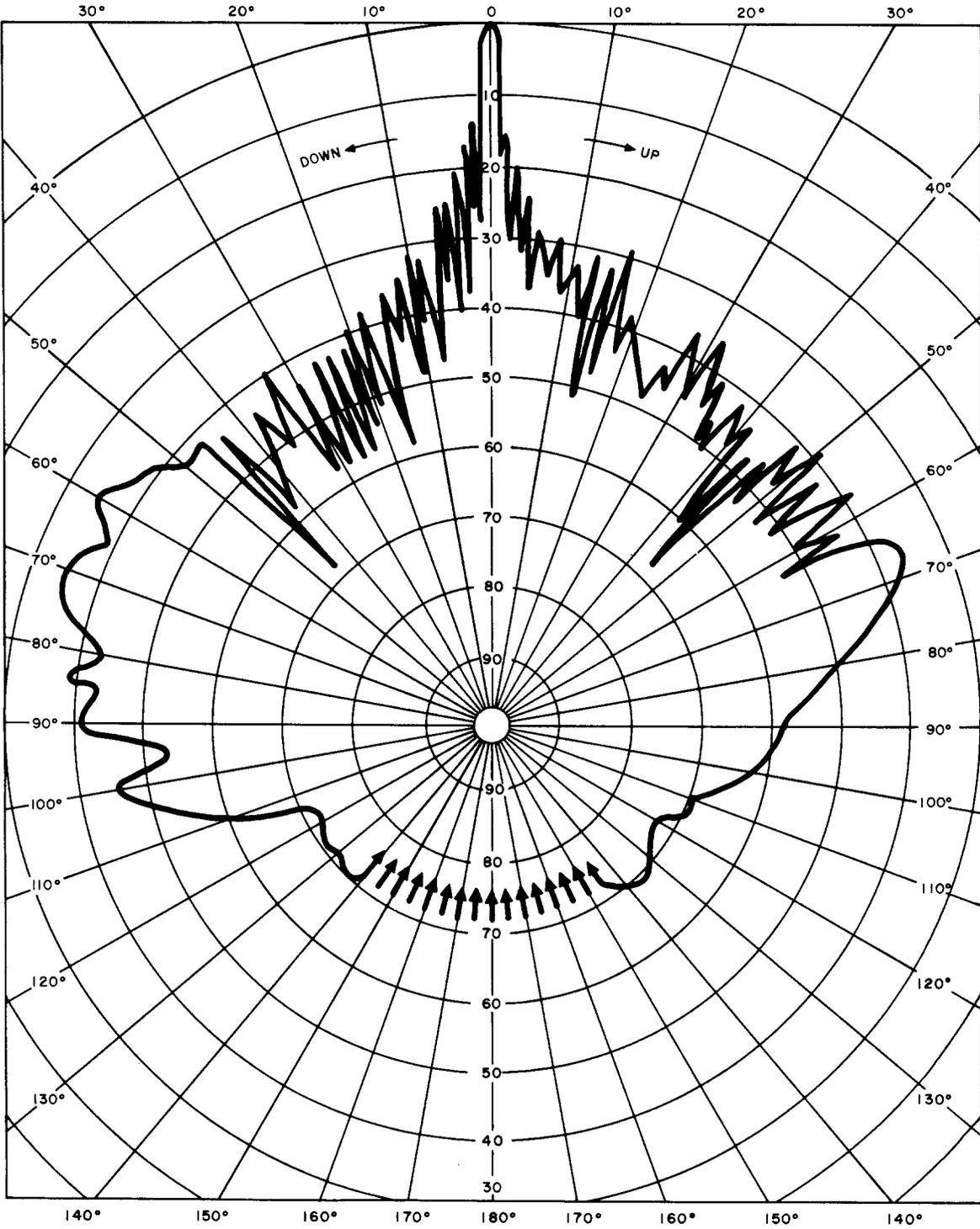
Fig. 15—Vertical Directivity—Vertical Polarization—6325 MHz (360 Degrees)
