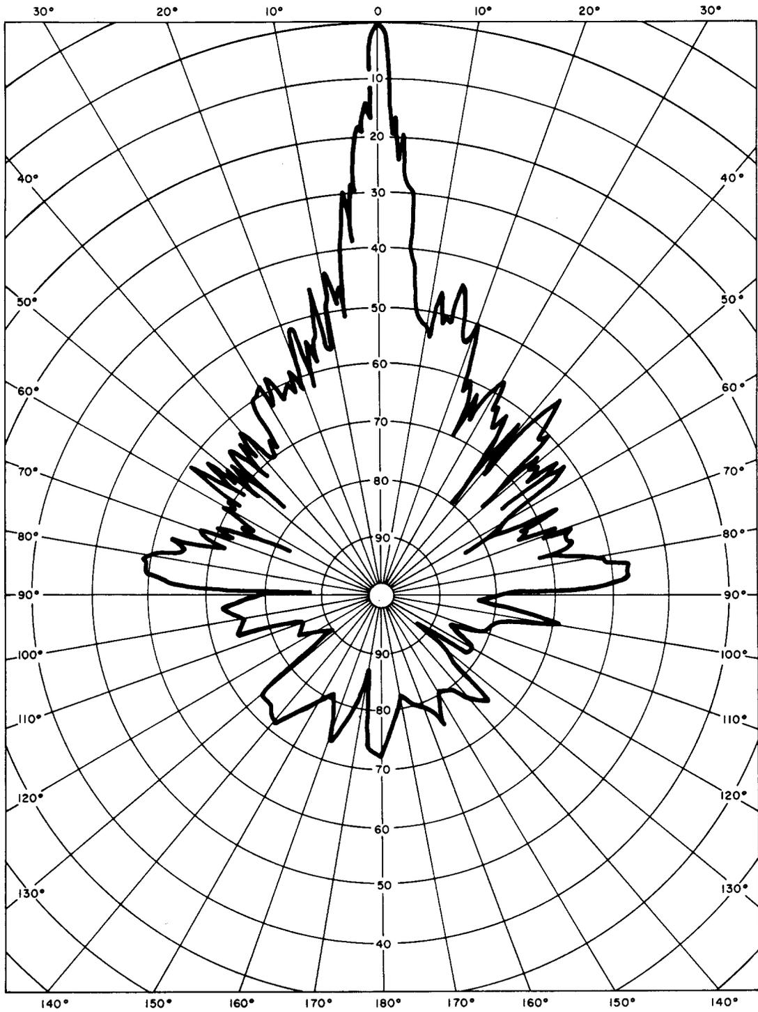
Fig. 10—Horizontal Directivity—Horizontal Polarization—6325 MHz (360 Degrees)
