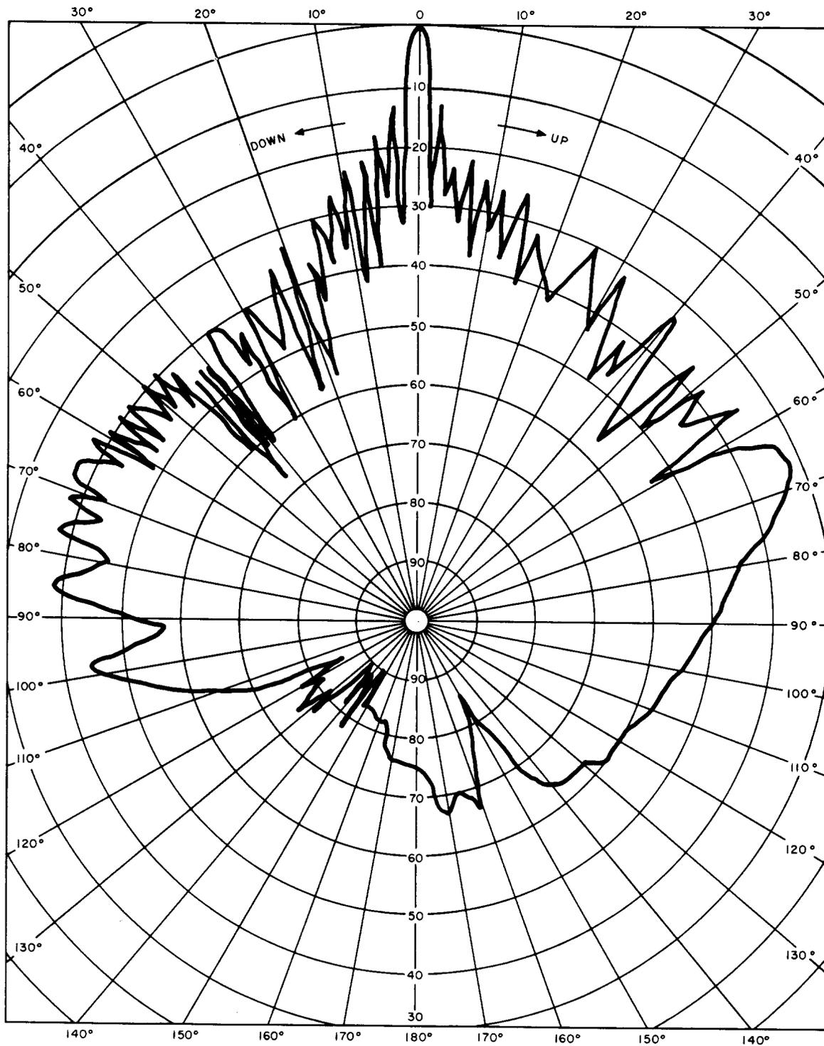
Fig. 13—Vertical Directivity—Vertical Polarization—3740 MHz (360 Degrees)
