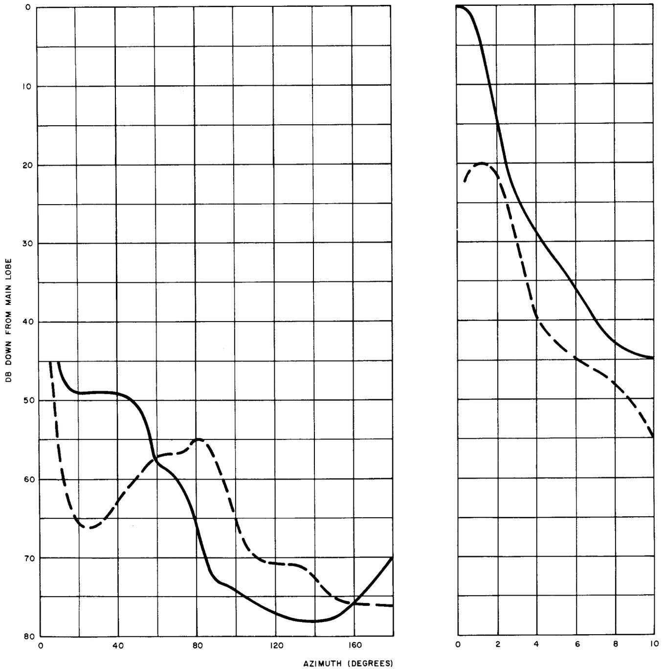
Fig. 20—Smoothed Horizontal Directivity—Vertical Polarization—4 GHz
