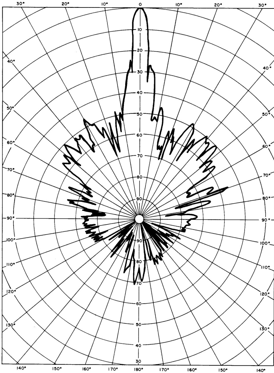
Fig. 7—Horizontal Directivity—Vertical Polarization—3740 MHz (360 Degrees)
