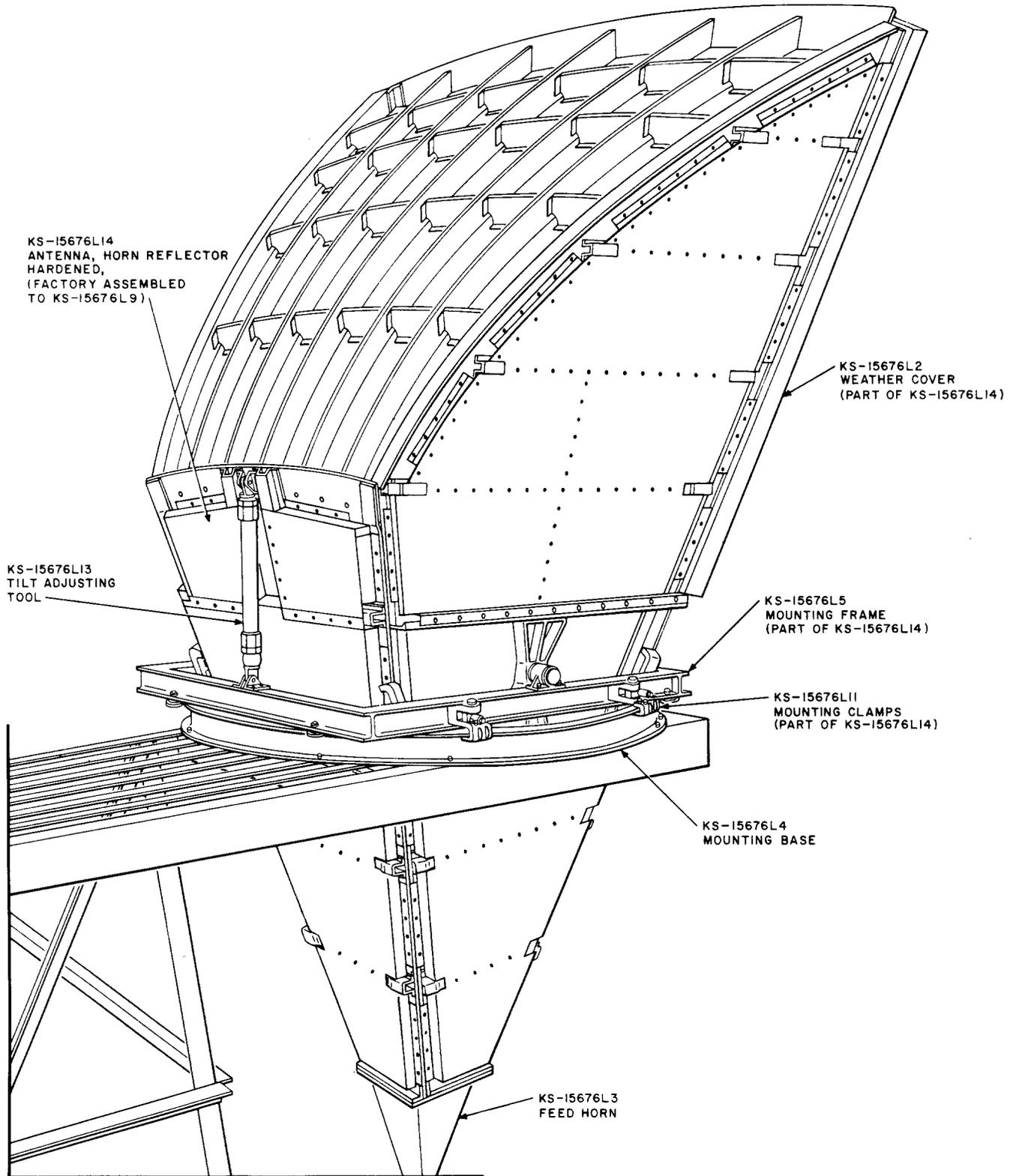
Fig. 2—KS-15676 L14 Hardened Horn Reflector Antenna
