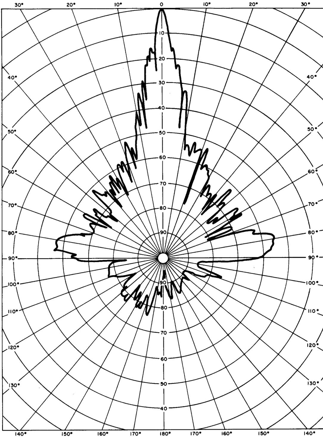
Fig. 8—Horizontal Directivity—Horizontal Polarization—3740 MHz (360 Degrees)
