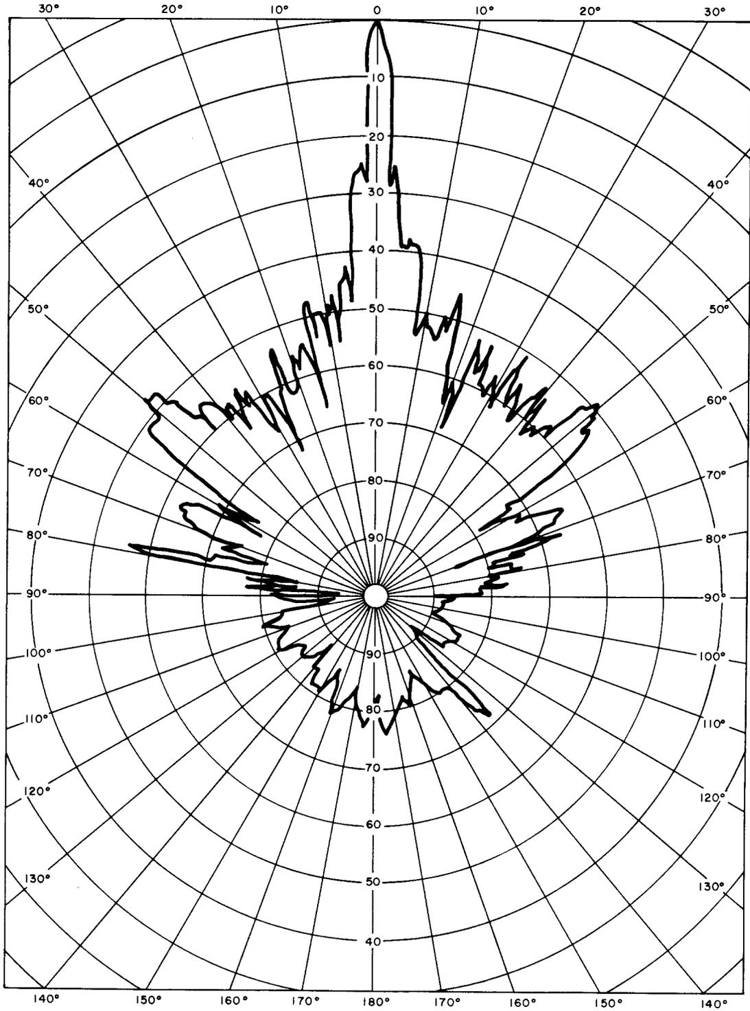
Fig. 9—Horizontal Directivity—Vertical Polarization—6325 MHz (360 Degrees)
