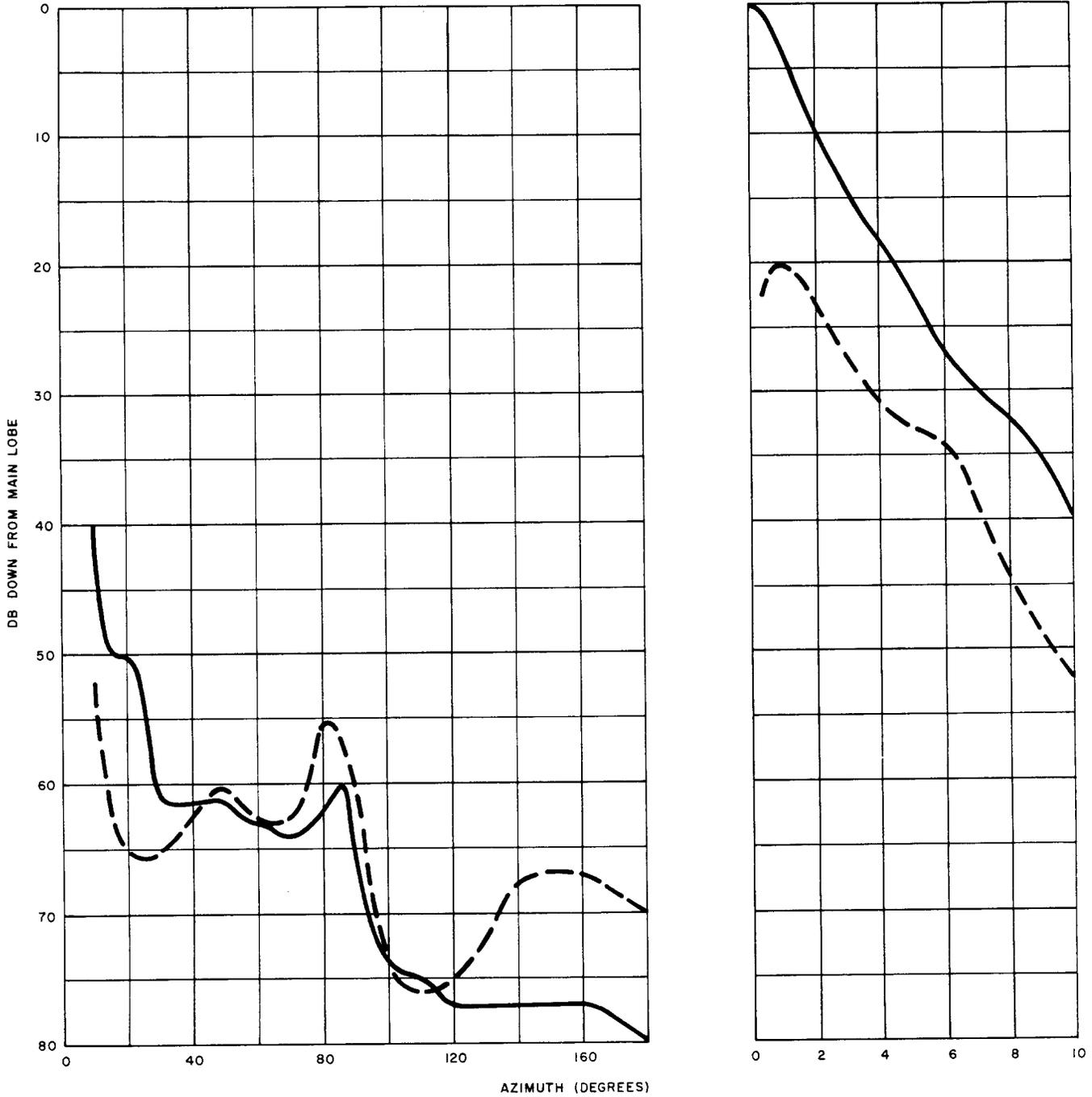
Fig. 21—Smoothed Horizontal Directivity—Horizontal Polarization—4 GHz
