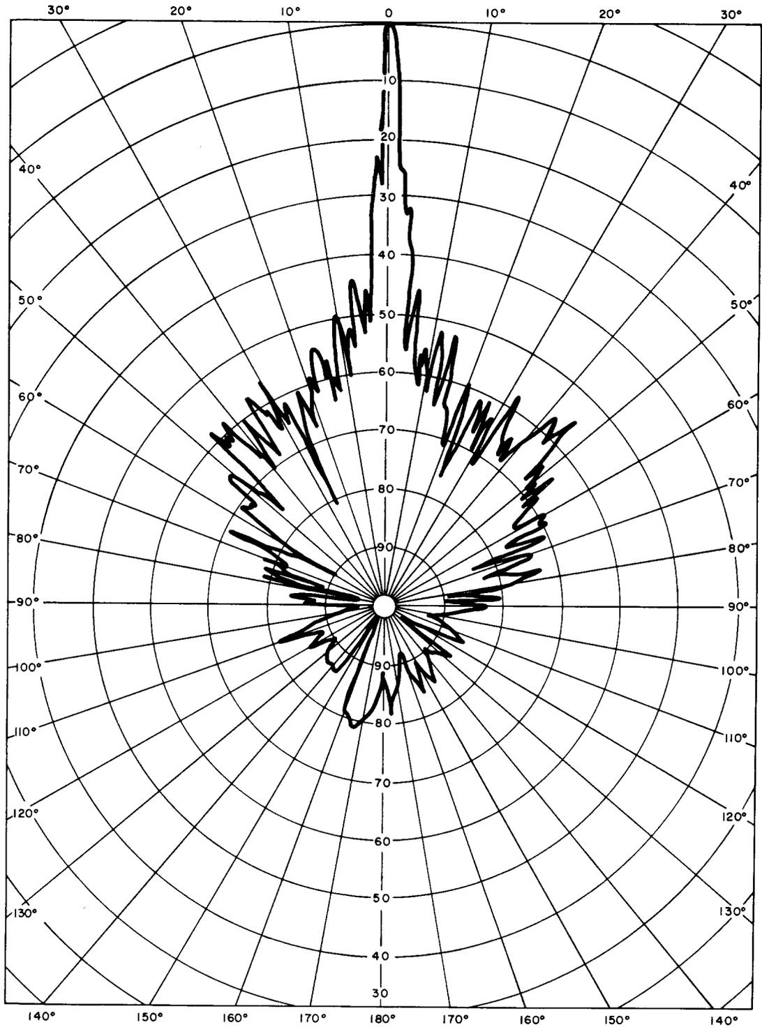
Fig. 11—Horizontal Directivity—Vertical Polarization—10,960 MHz (360 Degrees)
