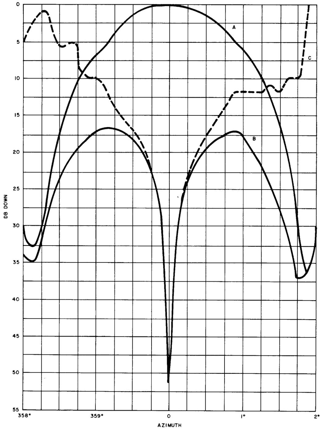
Fig. 4—Horizontal Polarization—Cross-Polarization Discrimination with Azimuth ( $\pm 2.5$  Degrees)—6325 MHz
