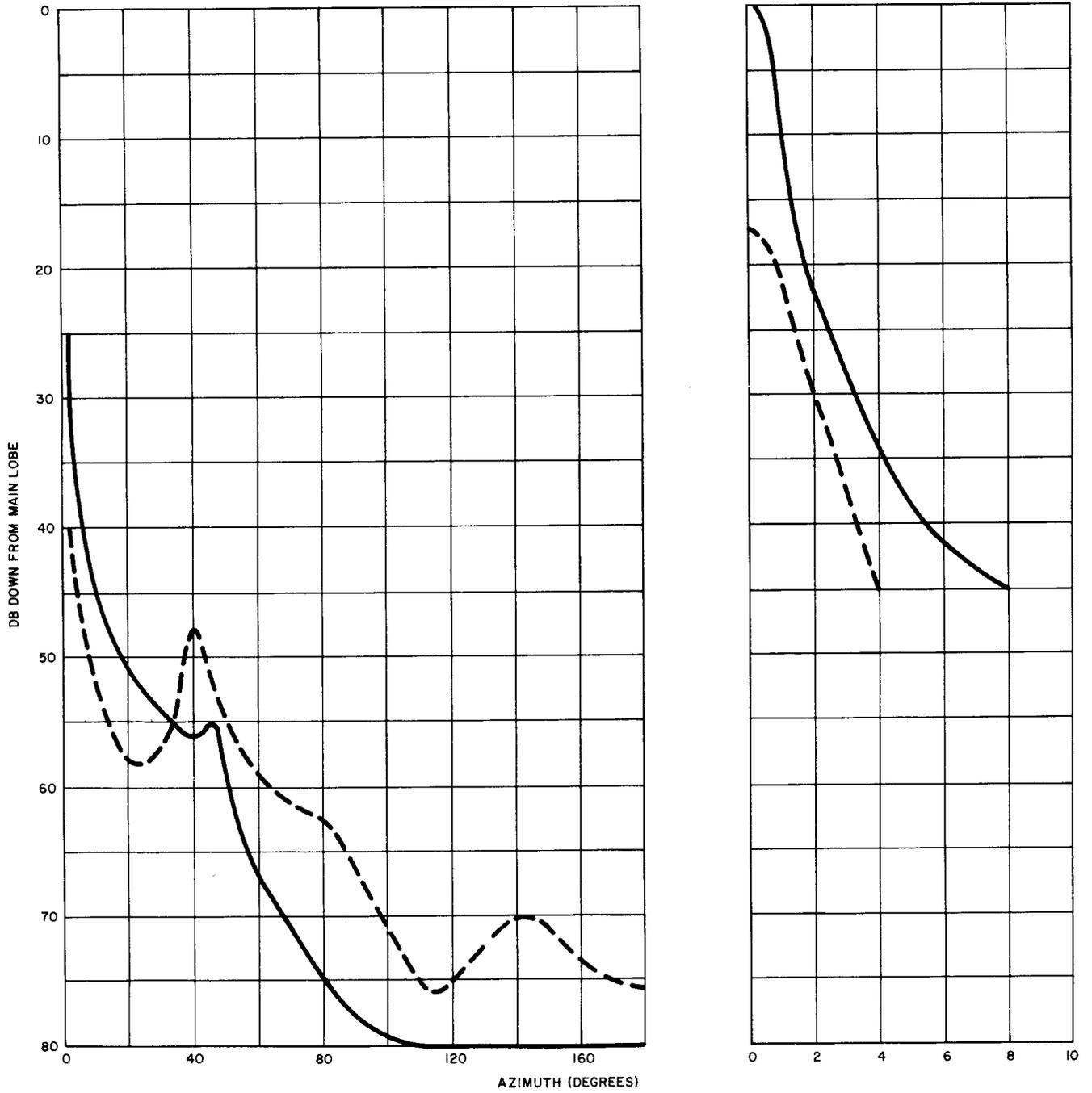
Fig. 24—Smoothed Horizontal Directivity—Vertical Polarization—11 GHz
