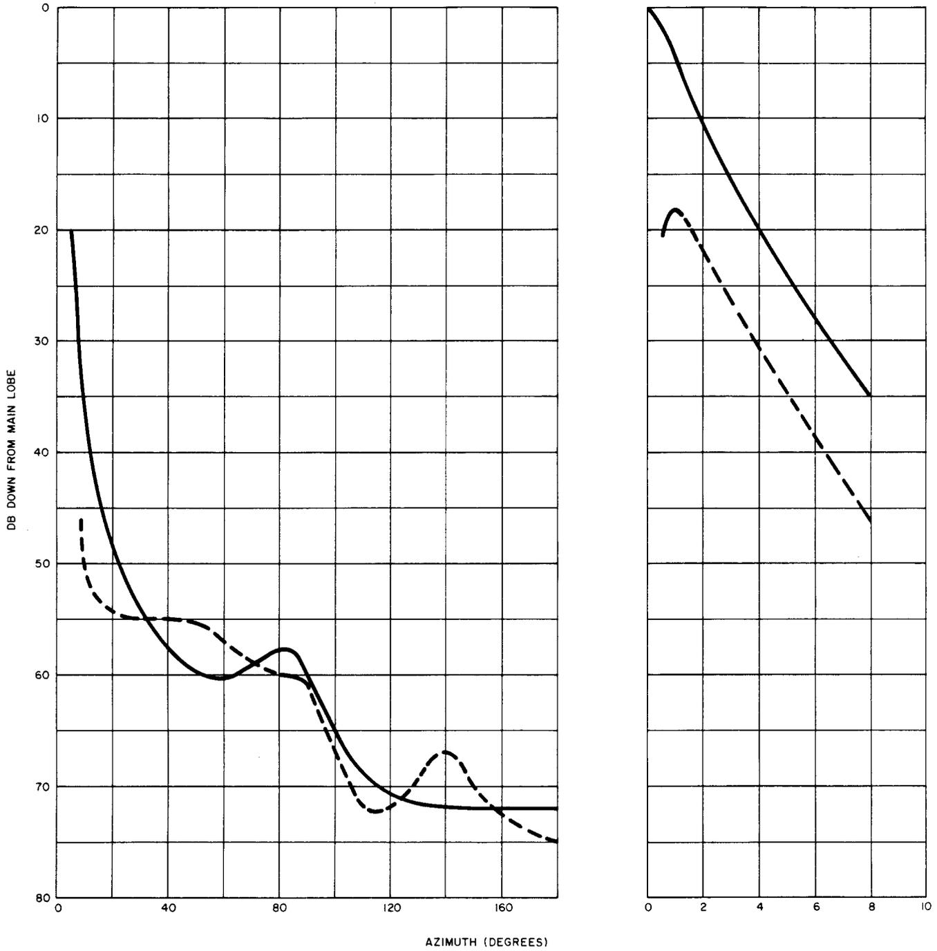
Fig. 23—Smoothed Horizontal Directivity—Horizontal Polarization—6 GHz
