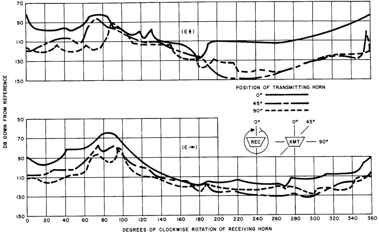
Fig. 17—Coupling—3740 MHz
