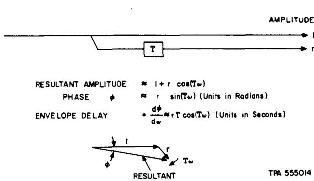
Fig. 9—Approximate Delay Characteristic
