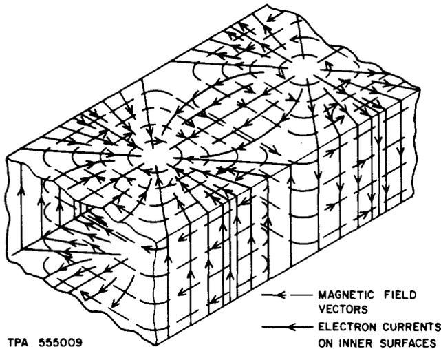
Fig. 4—Surface Current in Rectangular Waveguide
