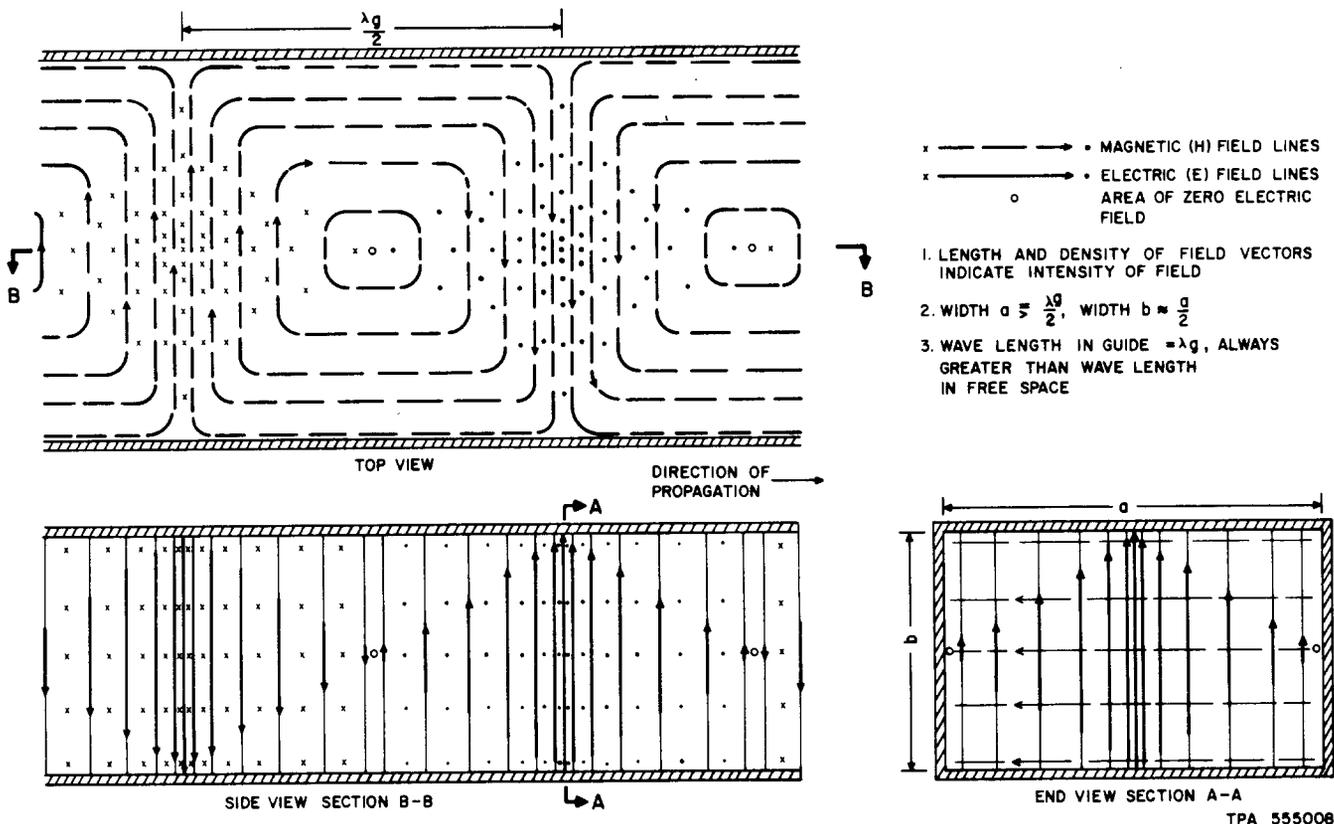
Fig. 3—Relative Fields in Dominant Mode Rectangular Waveguide
