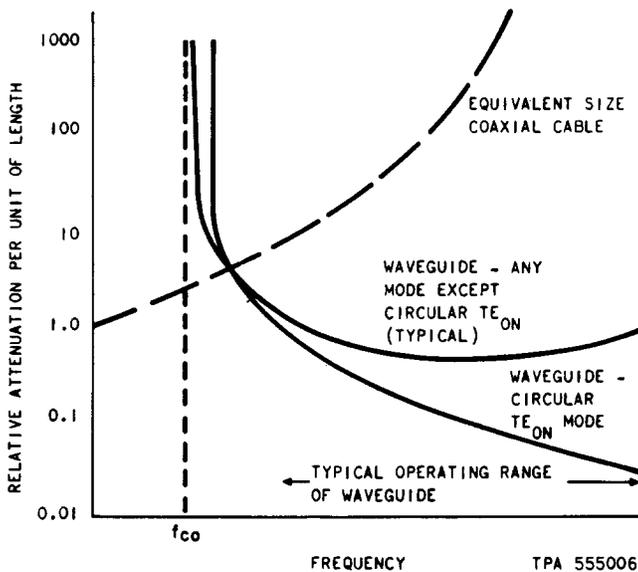
**Fig. 1—Relative Attenuation vs Frequency Characteristics of Comparable Size Waveguide and Coaxial Cable**
