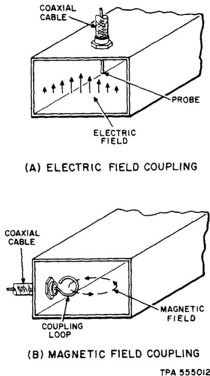
Fig. 7—Coupling Into or Out of Waveguide
