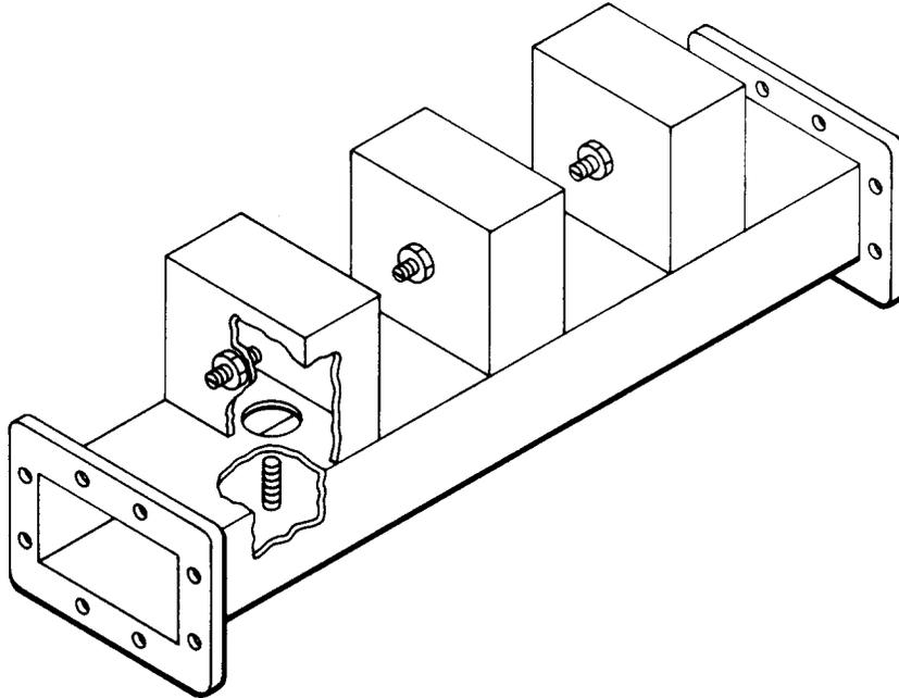
(A) 4-GHZ BAND-REJECT FILTER
