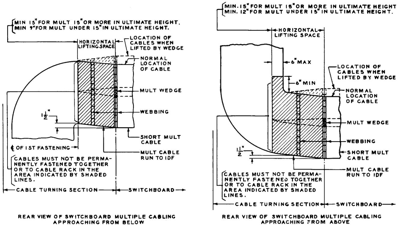
Fig. 5 – Cabling In Switchboard Cable Turning Sections
