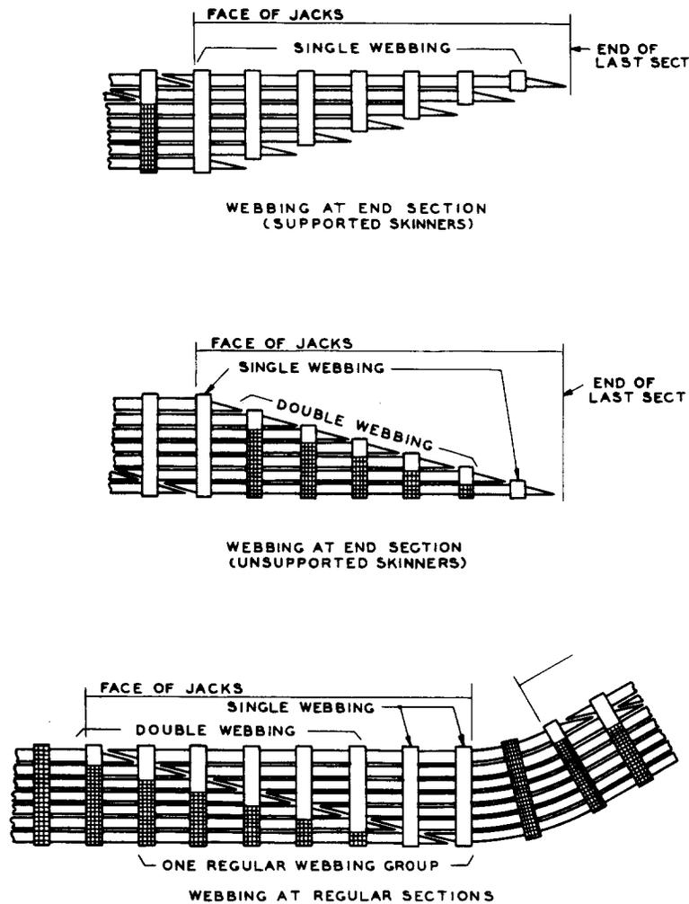
NOTE: THE SHADED PORTIONS OF THE WEBS INDICATE THE CABLES OVER WHICH THE DOUBLE OR FOLDED PORTION EXTENDS.
