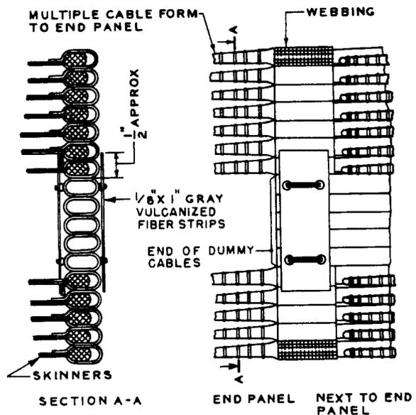
Fig. 4 - Fastening Dummy Cables In End Panels Of Switchboards
