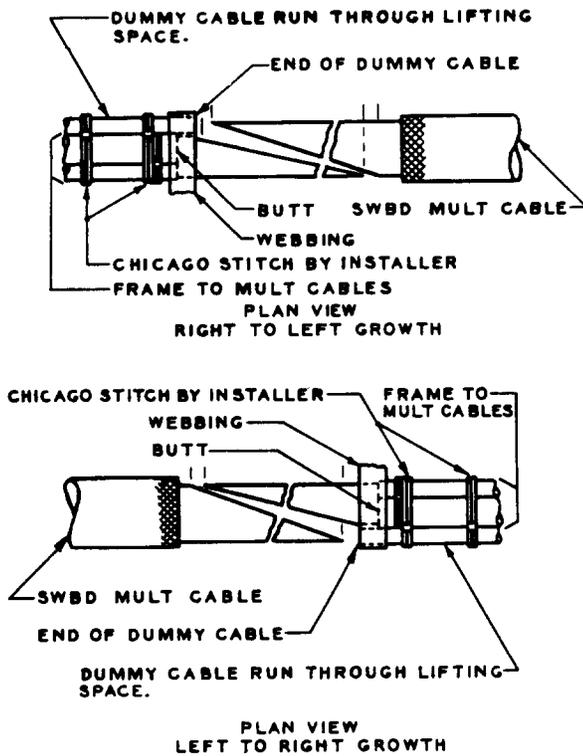
Fig. 3 - Method of Adding Dummy Cables To Frame-to-Multiple Cables
