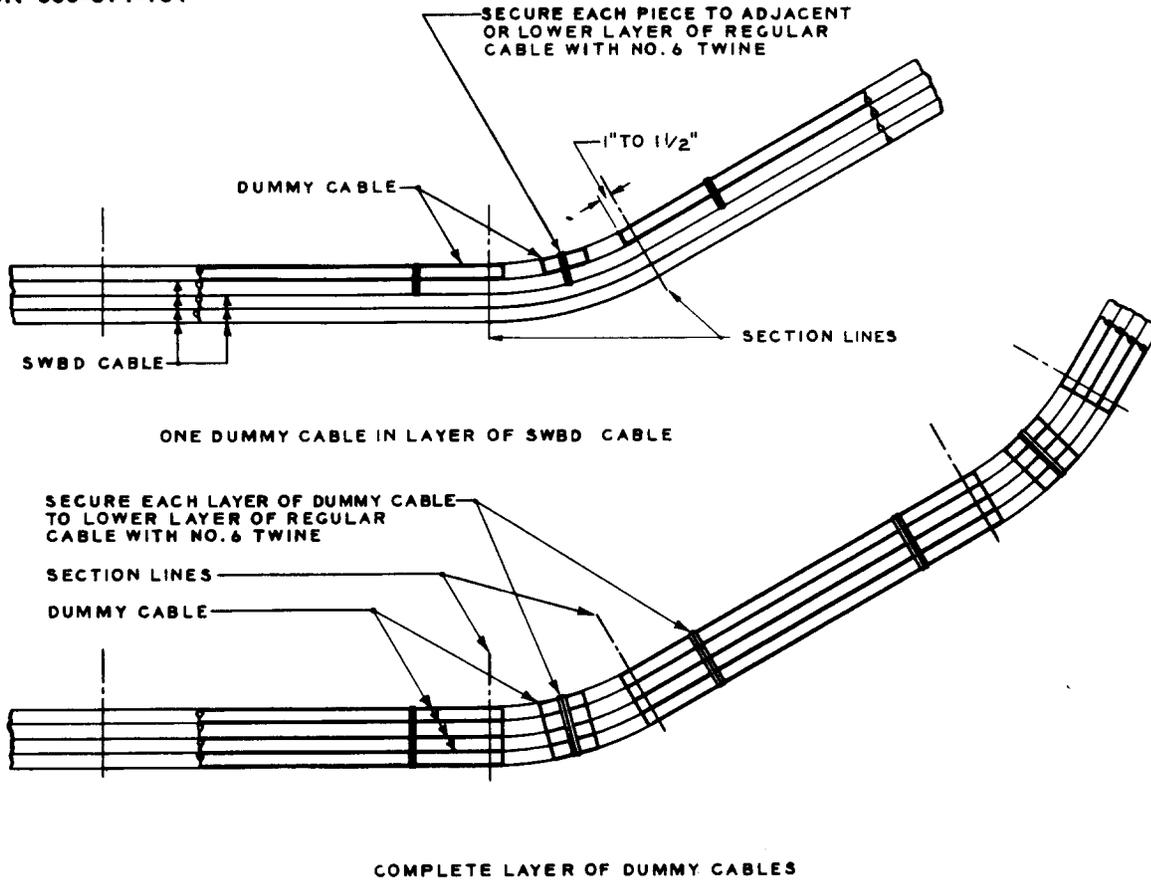
Fig. 2 - Method of Using Flat-type Nonmetallic Dummy Cables in Angle Sections
