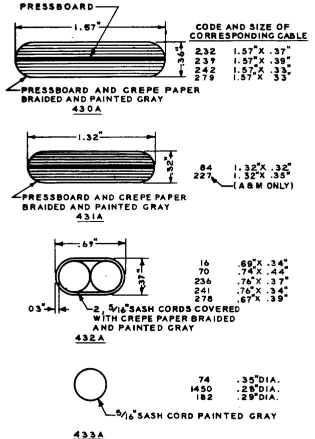
Fig. 1 — Nonmetallic Dummy Cables
