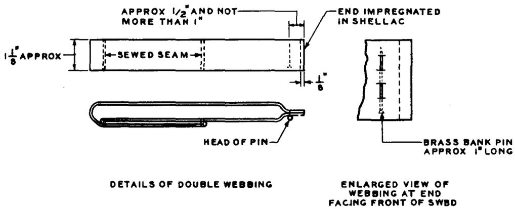
Fig. 6 - Webbing Cables in Switchboards and Desks - Graduated Double Webbing
