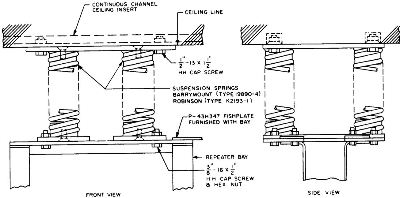
Fig. 5—Fastening Shock Mount System
