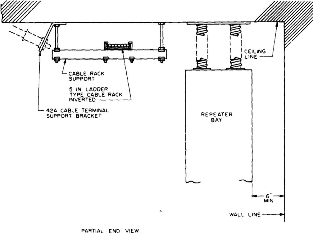
Fig. 3—Typical Cable Rack Arrangement
