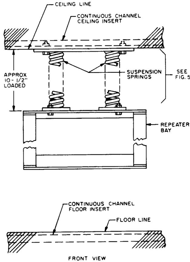
Fig. 4—Typical Shock-Mounted Auxiliary Repeater Bay
