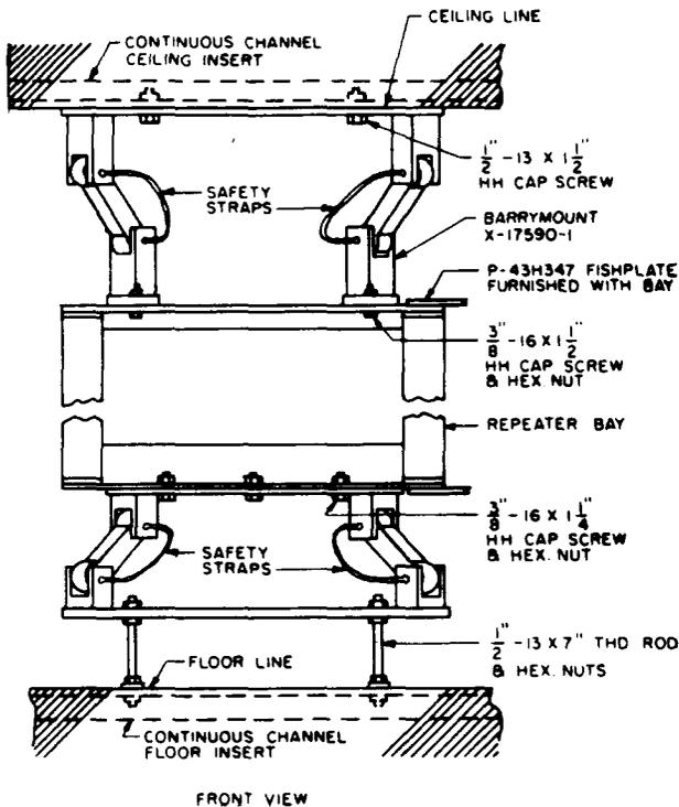
**Fig. 1—Early Type Shock Isolator Installation for Auxiliary Repeater Bays (Mfr Disc.— Replaced by Fig. 4)**
