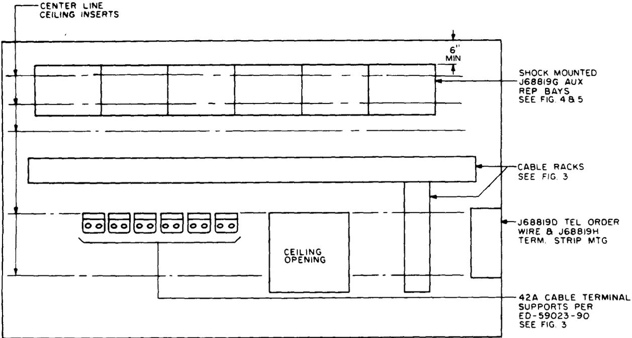
Fig. 2—Typical Layout of an Underground Auxiliary Repeater Station
