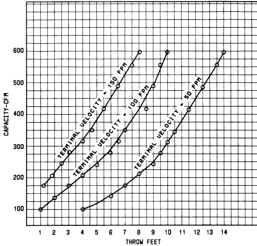
Fig. 5—Cfm Capacity Versus Throw at Terminal Velocities of 150, 100, and 50 fpm
