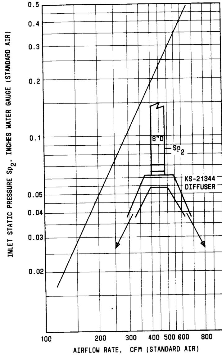
Fig. 4—Pressure Drop Versus cfm Capacity
