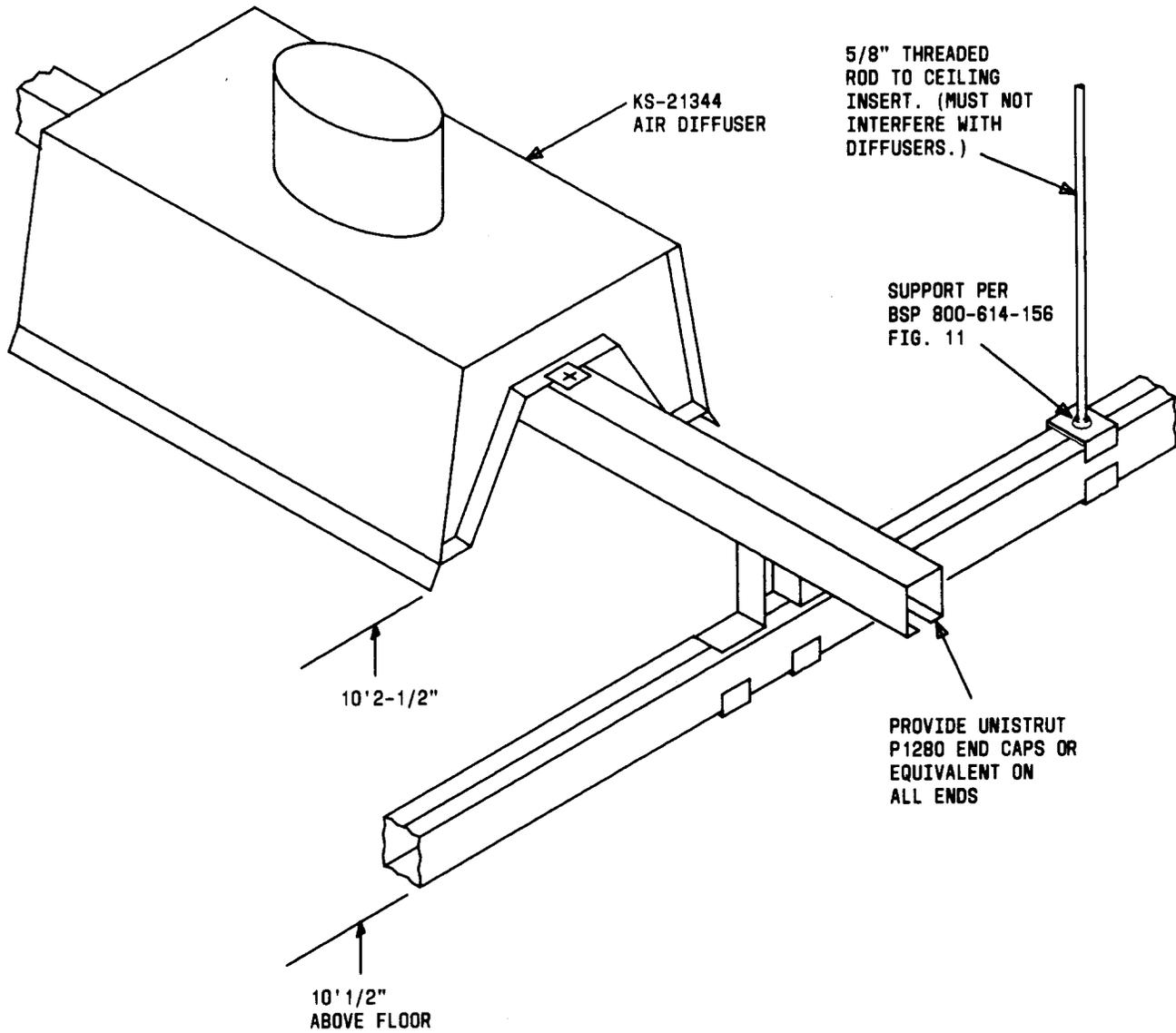
Fig. 2—Framing and Support for KS-21344 Air Diffuser
