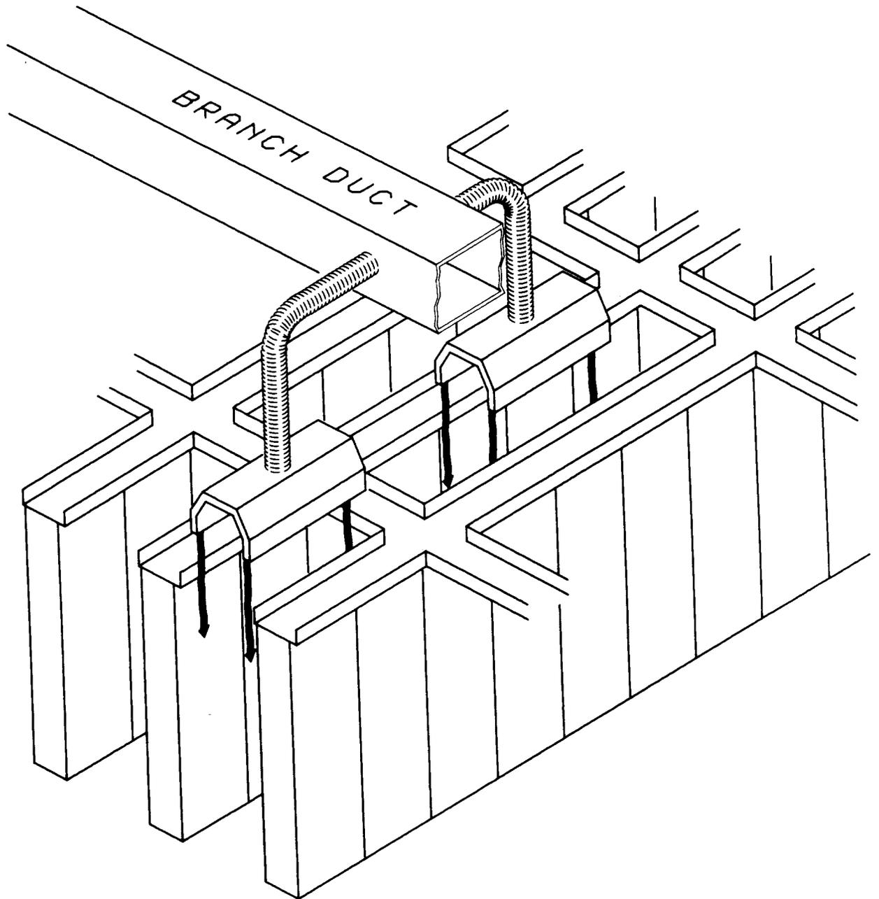
**Fig. 3—Conventional Drop Diffuser Air Supply System**
