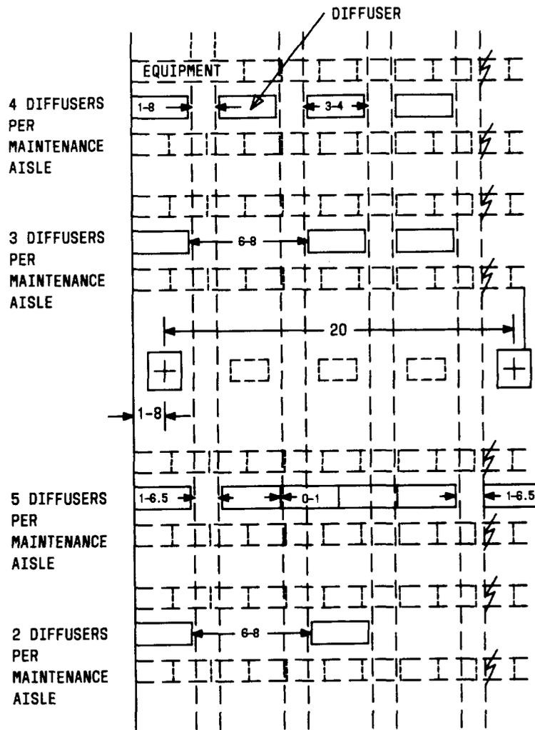
Fig. 9— Various Diffuser Arrangements for Four Cross-Aisle Pathways per Building Bay
