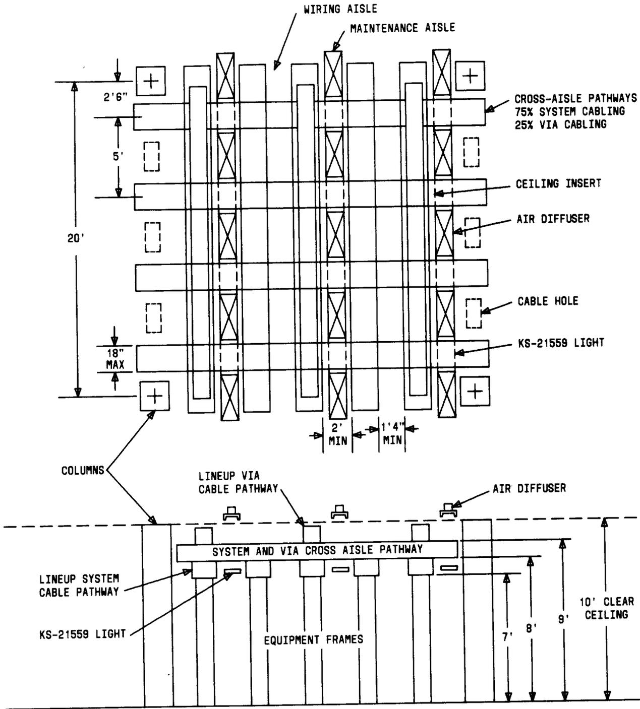
Fig. 8—Cable Pathways Plan for 12-Inch Deep Frame Areas
