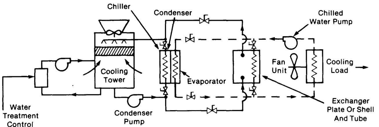
Fig. 11—Cooling Tower and Heat Exchanger
