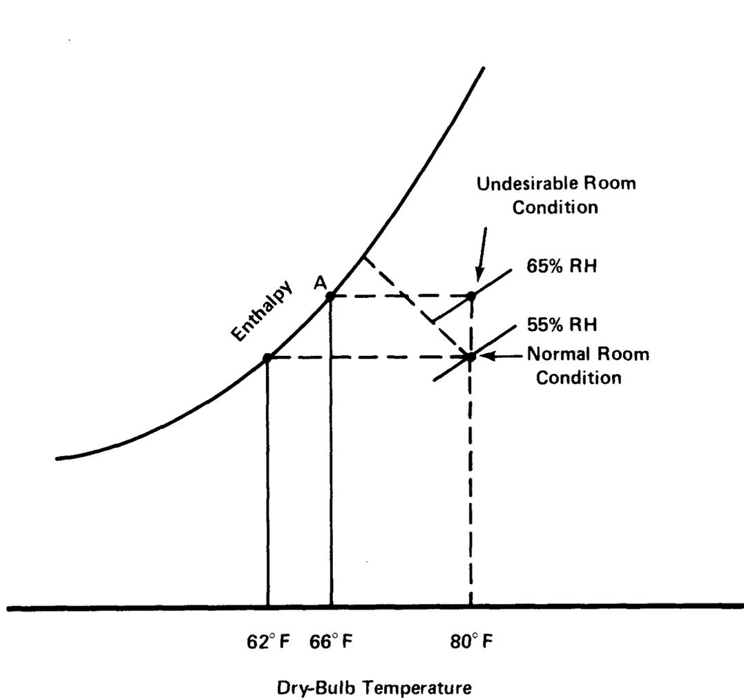
Fig. 7—Air Economizer System—Potential Humidity Problem Associated With Economy Cycle Operation
