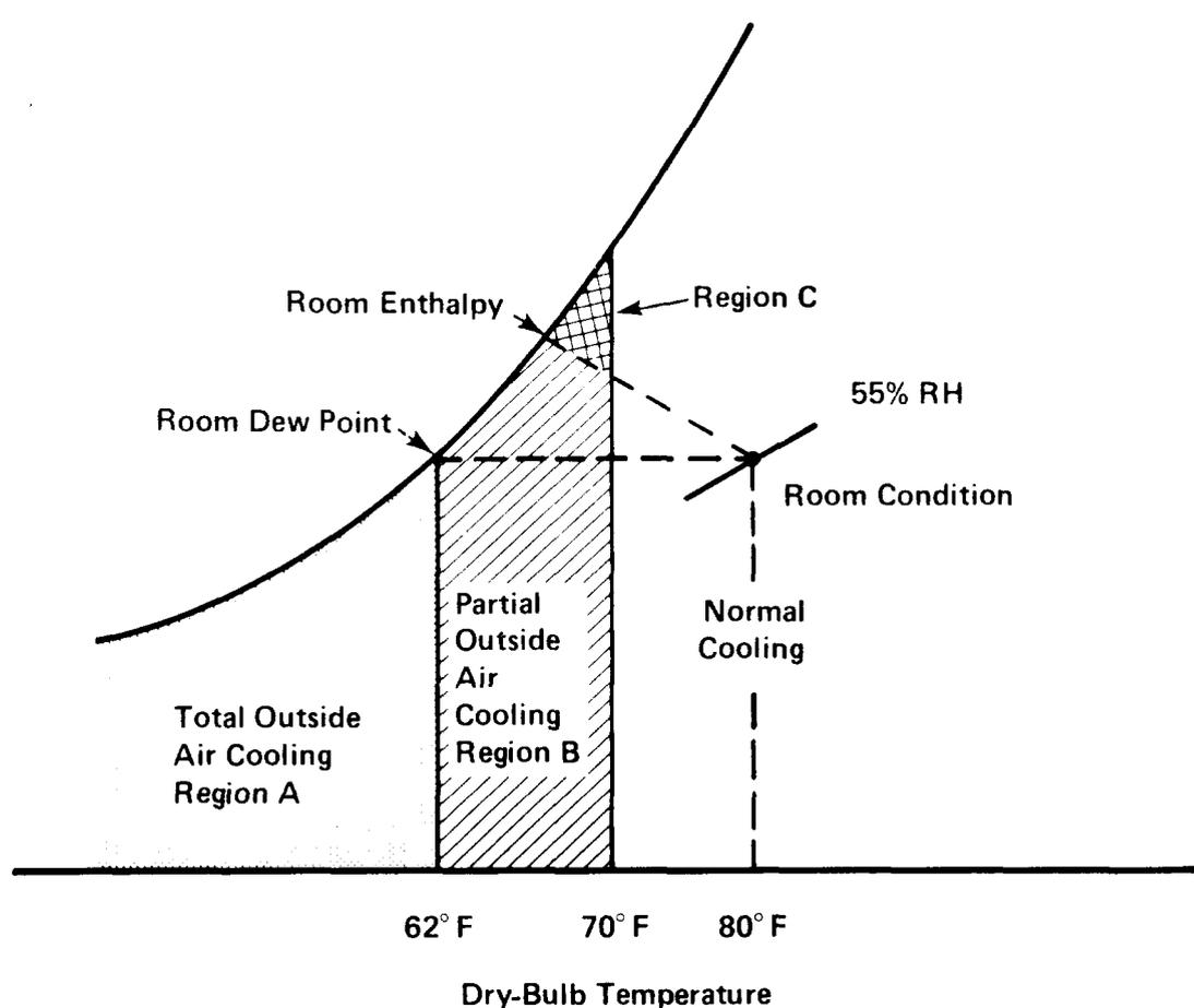
Fig. 3—Air Economizer System—Dry-Bulb Economy Control Operation With 70°F Changeover Point
