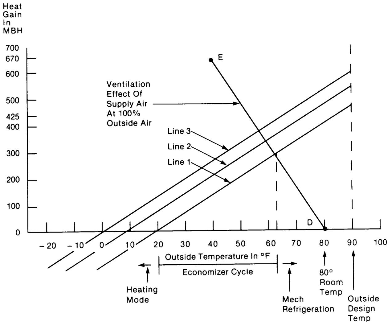
Fig. 13—Ventilation Effect of Supply Air
