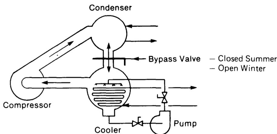
Fig. 9—Pumped Vapor Cycle
