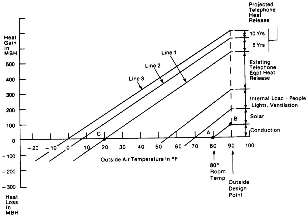
Fig. 12—Energy Load Profile Based on 80°F Room Temperature
