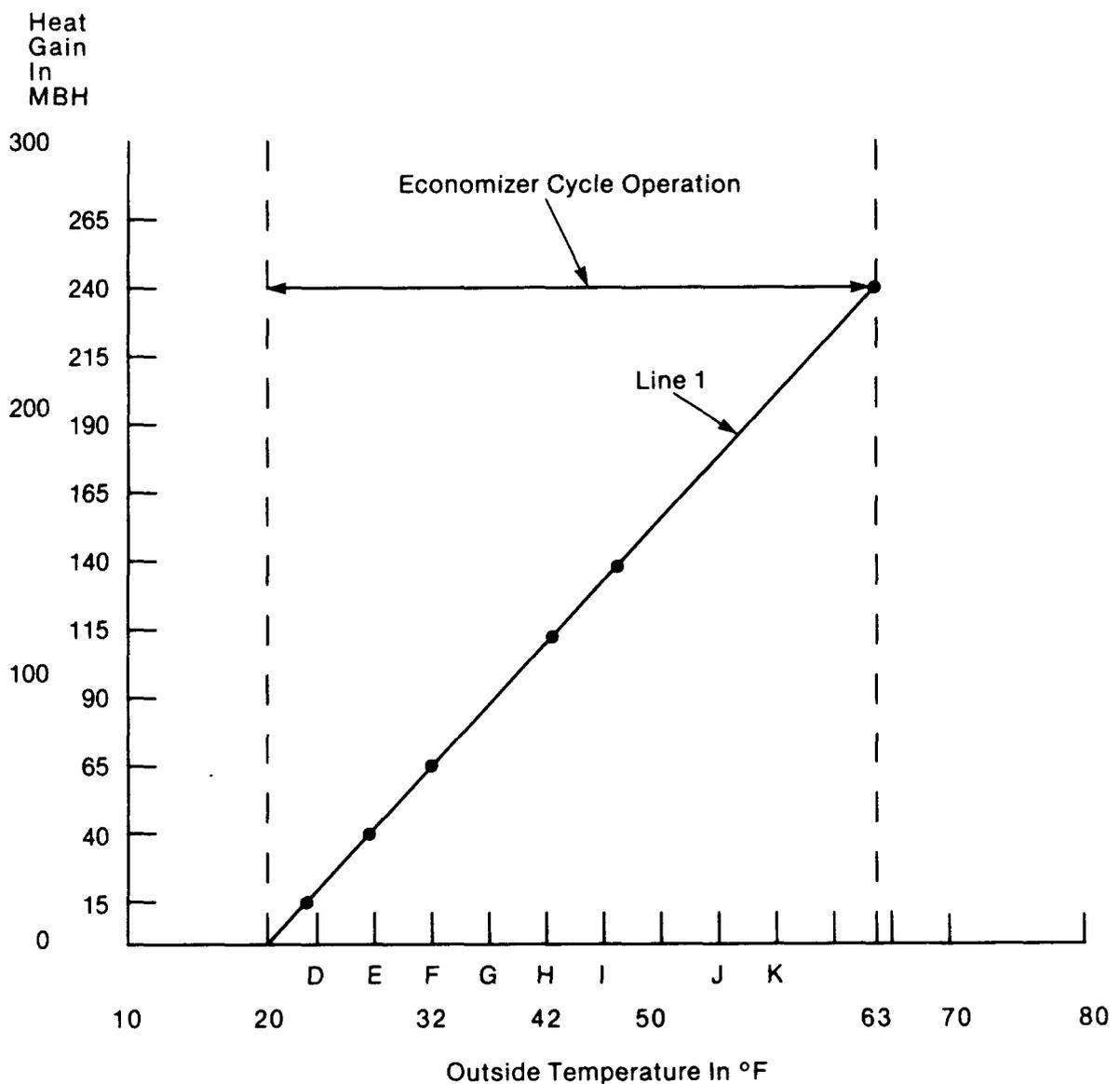
Fig. 14—Economizer Cycle—Energy Profile—MBH Heat Gain Per BIN
