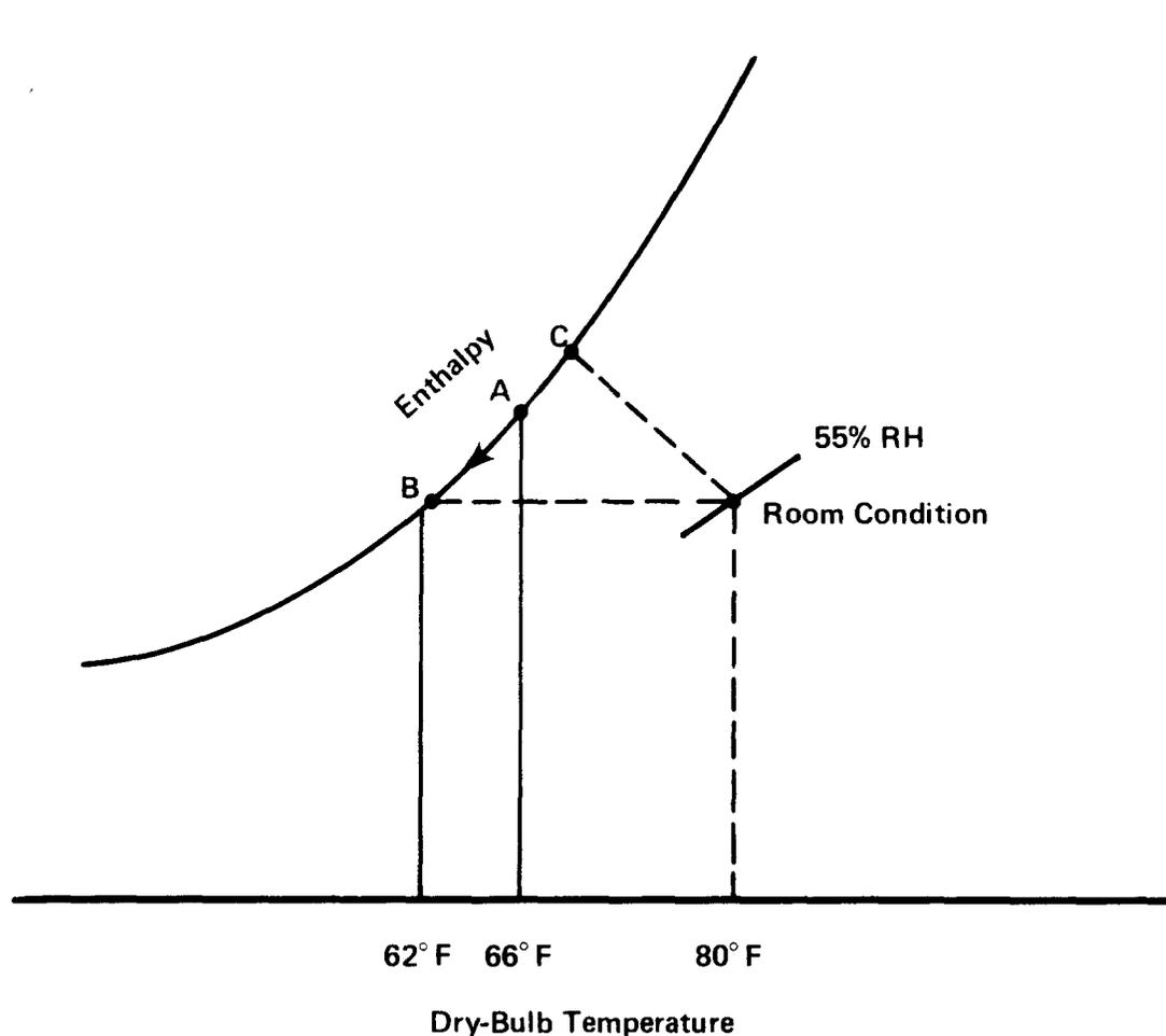
Fig. 6—Air Economizer System—Economy Cycle Operation Under Humid Outside Conditions
