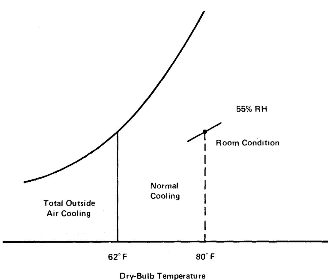
Fig. 2—Air Economizer System—Dry-Bulb Economy Control Operation With 62°F Changeover Point
