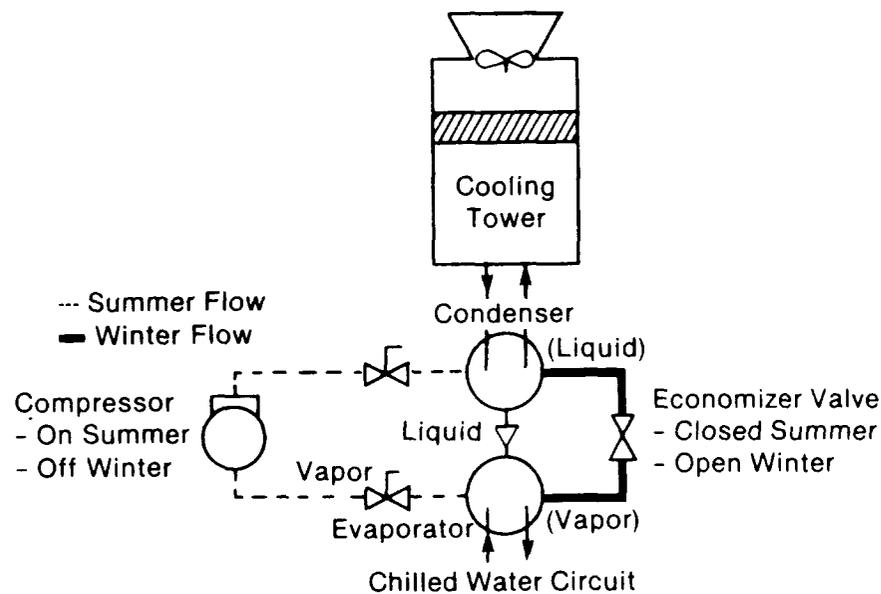
Fig. 8—Chiller Vapor Cycle
