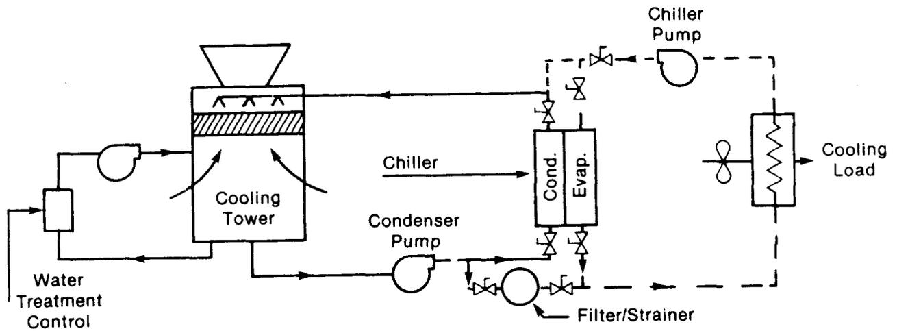
Fig. 10—Filtration or Strainer System
