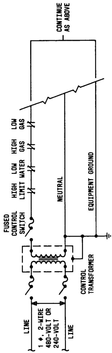
Fig. 1 — Heating Plant Control Circuit
