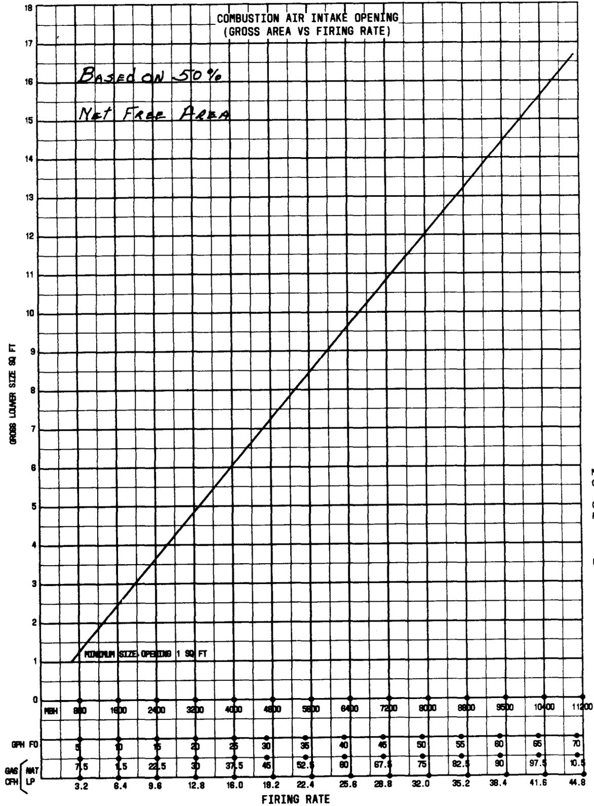
Fig. 24—Combustion Air Intake Opening (Gross Area Versus Firing Rate)
