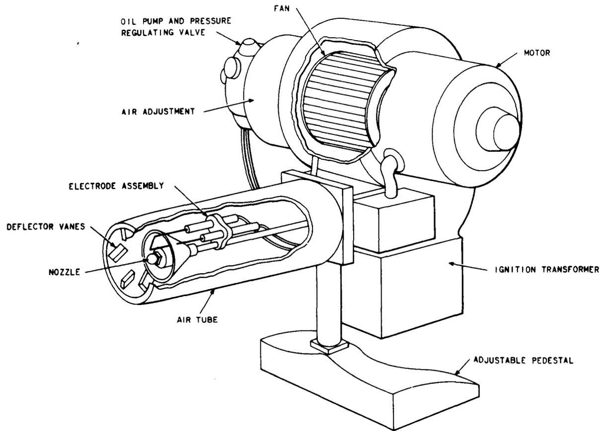
Fig. 19—High-Pressure Atomizing Burner (Reprinted with permission, ASHRAE Guide and Data Book, 1963)
