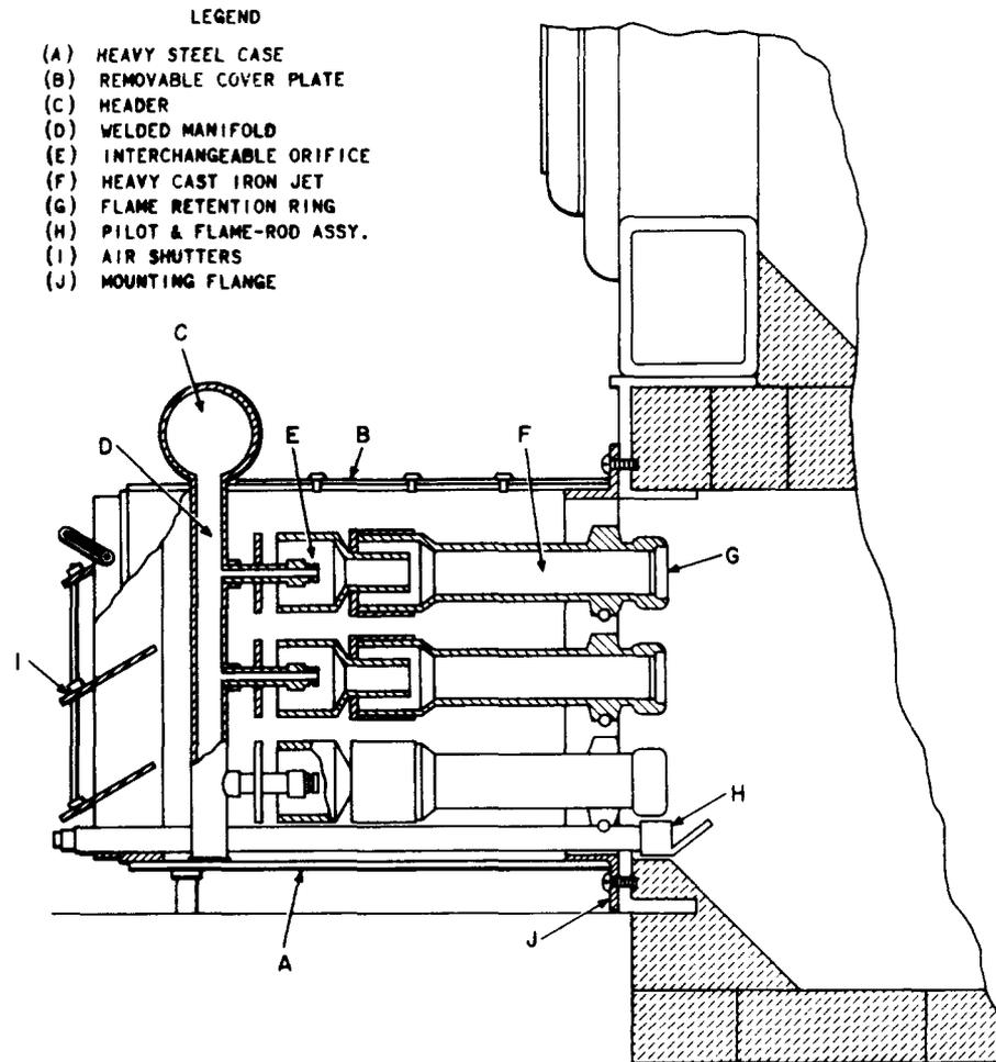
Fig. 22—Inshot Gas Burner—Cross-Sectional View (Reprinted with permission, Ray Burner Co)
