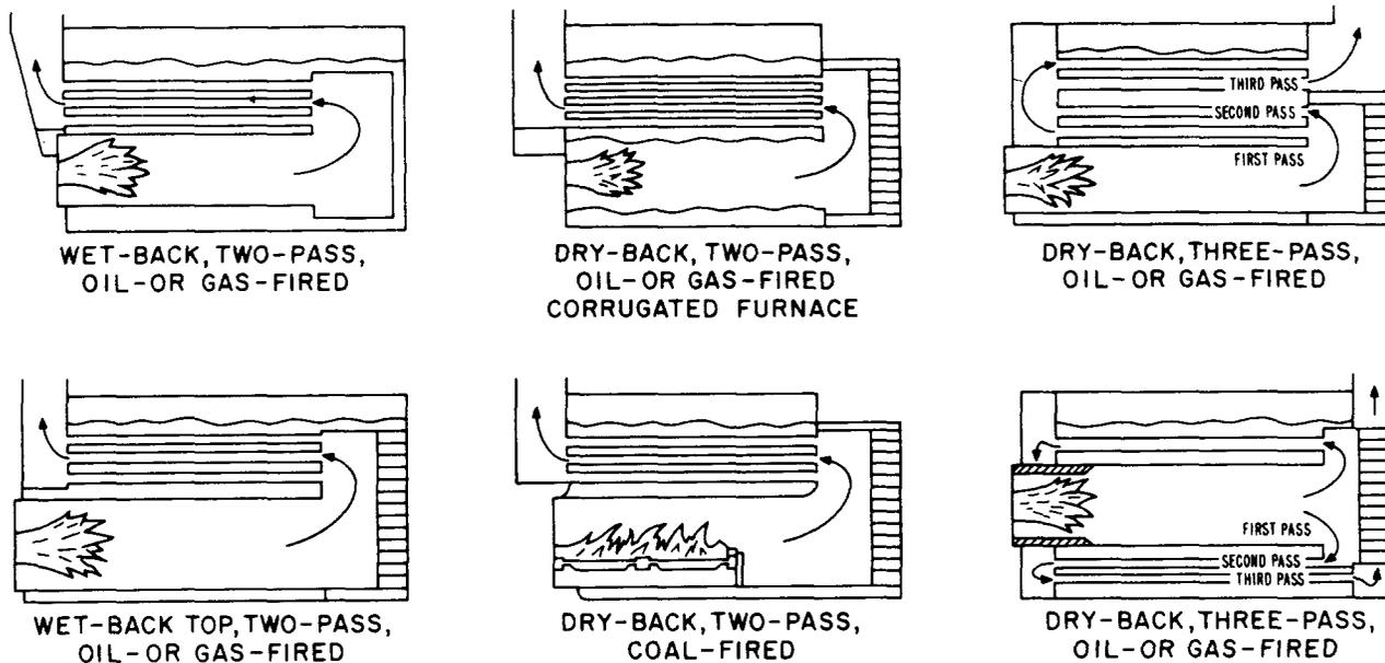
Fig. 9—Gas Flow in Scotch Boiler Types (Reprinted with permission, **BOILERS** by C. D. Shields. Copyright 1961. McGraw-Hill Book Co)
