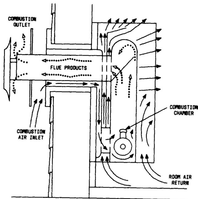
Fig. 15—Direct-Vent Wall Furnace
