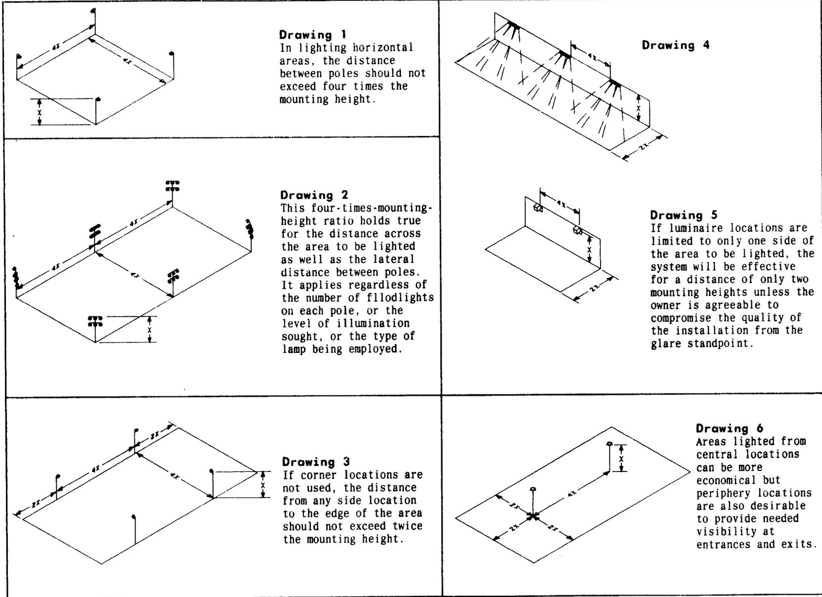
Fig. 1—Site Lighting Layout Considerations for Horizontal Surfaces
