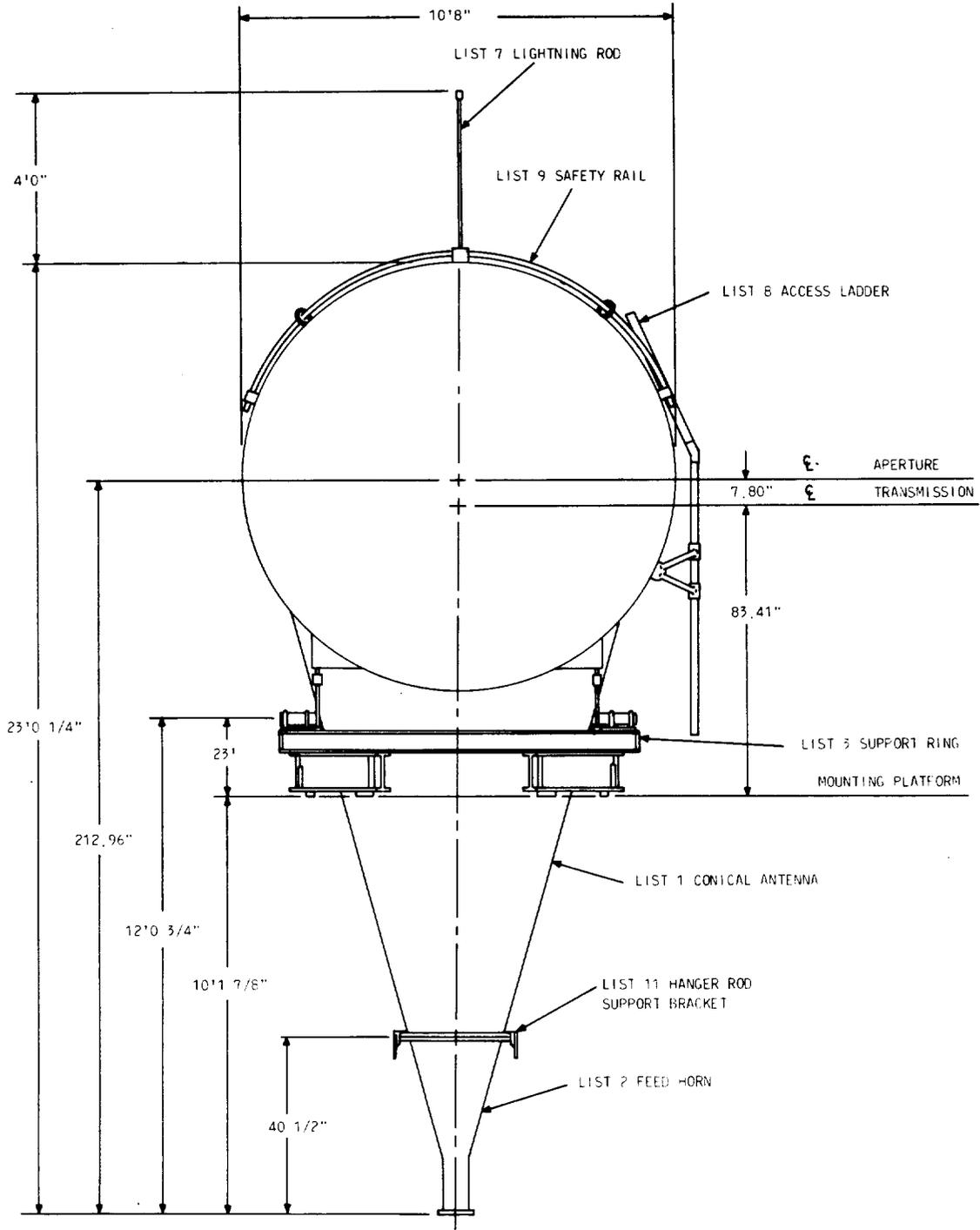
Fig. 1—KS-21972 Conical Antenna (Front View)
