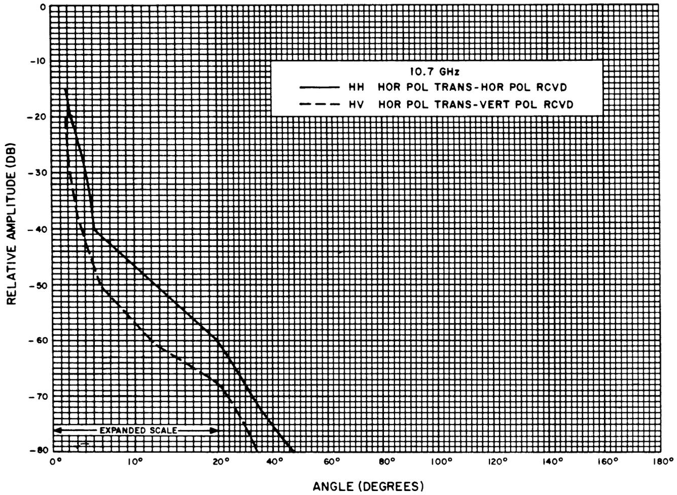
Fig. 8—KS-21972 Conical Antenna, 10.7 GHz, Horizontal Polarization Transmitted
