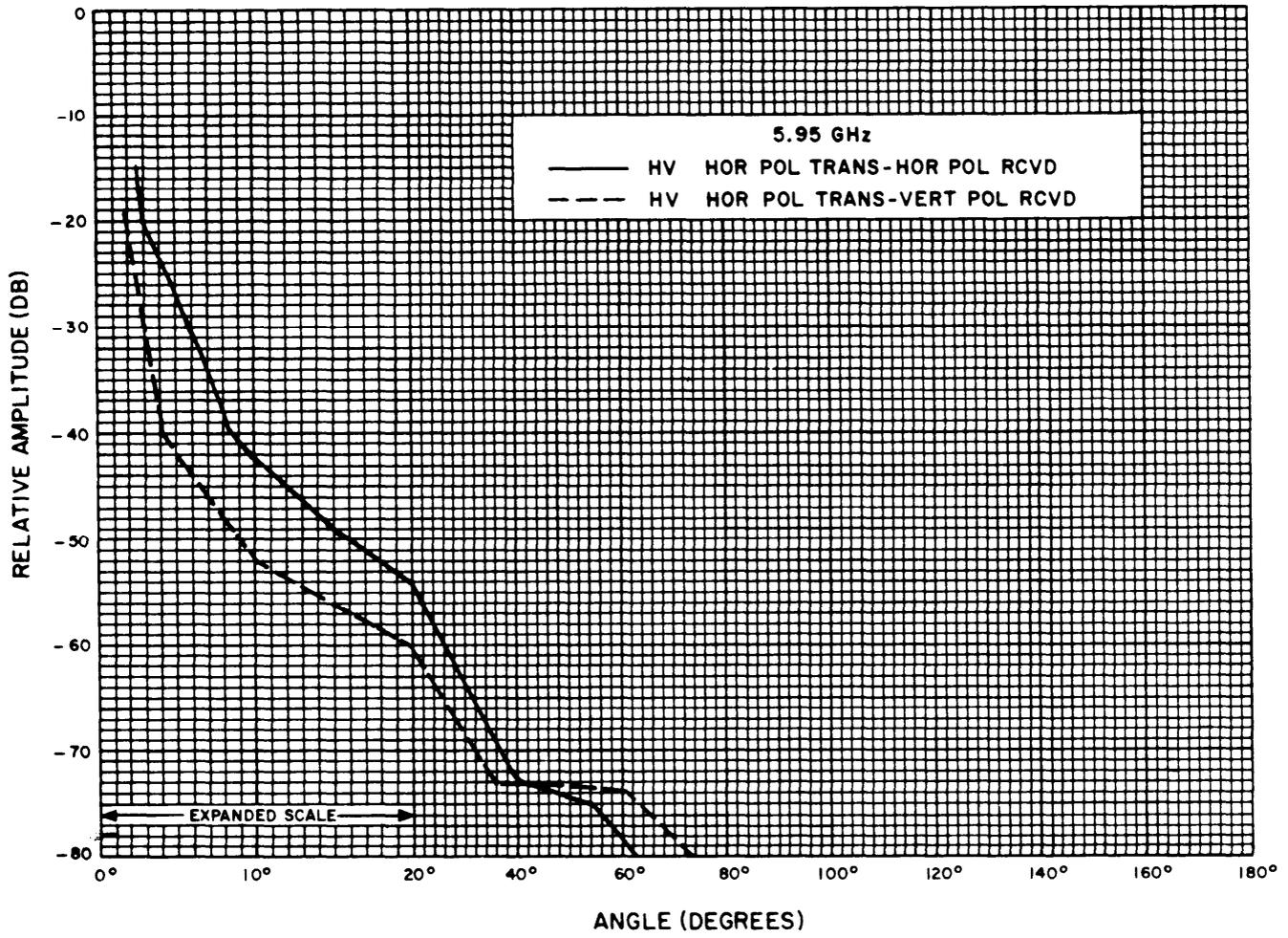
Fig. 6—KS-21972 Conical Antenna, 5.95 GHz, Horizontal Polarization Transmitted
