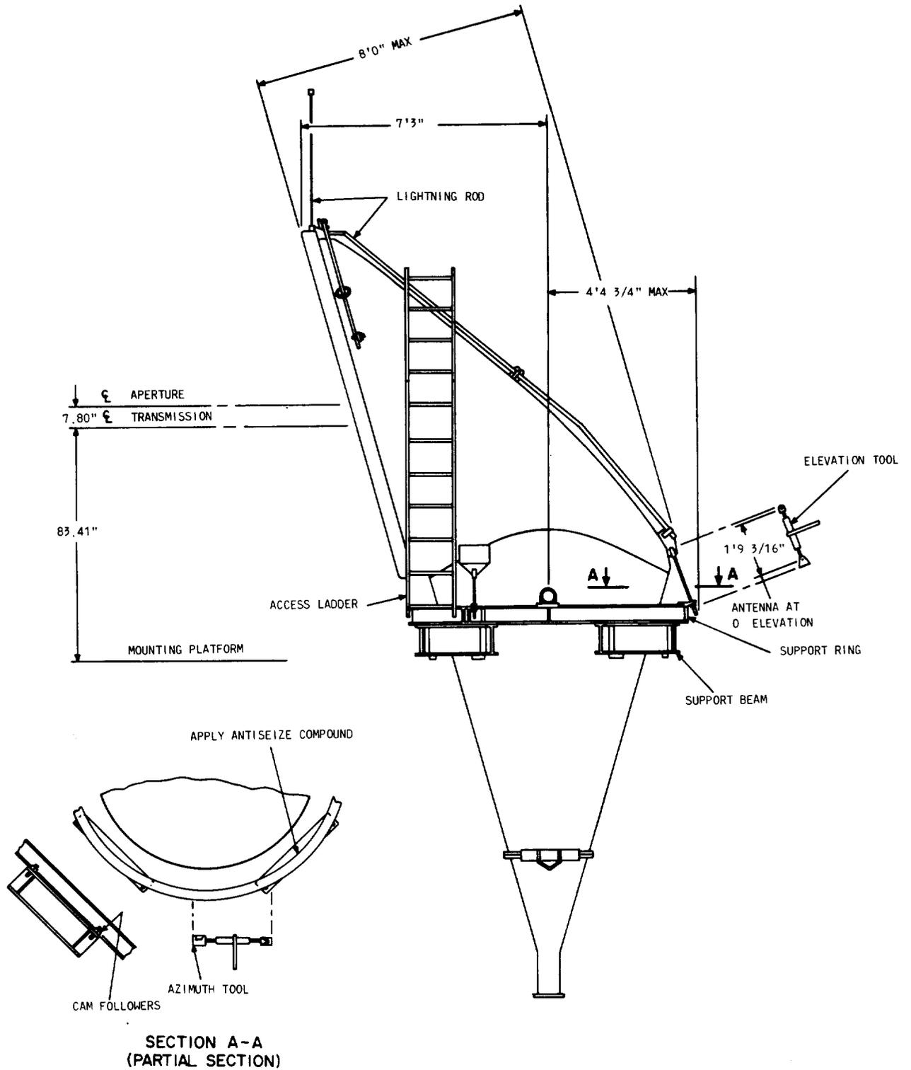
Fig. 2—KS-21972 Conical Antenna (Side View)
