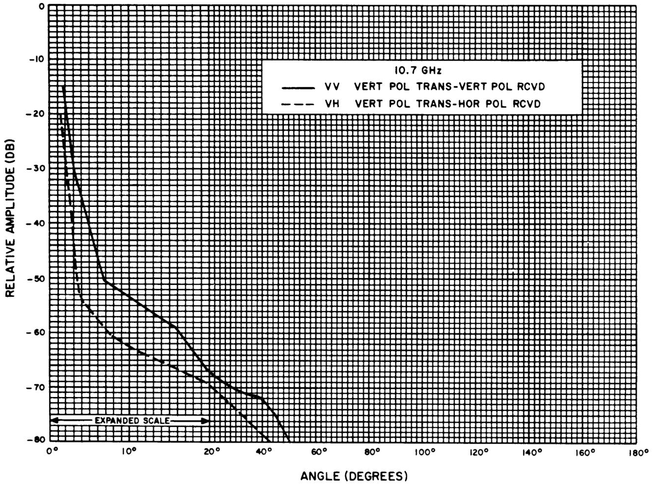
Fig. 7—KS-21972 Conical Antenna, 10.7 GHz, Vertical Polarization Transmitted
