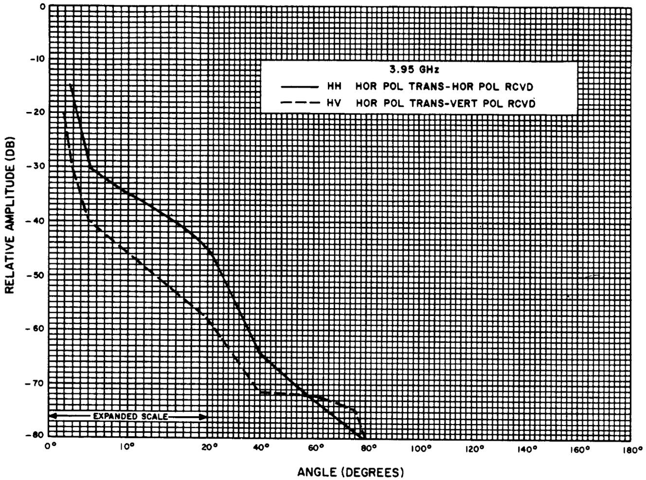
Fig. 4—KS-21972 Conical Antenna, 3.95 GHz, Horizontal Polarization Transmitted
