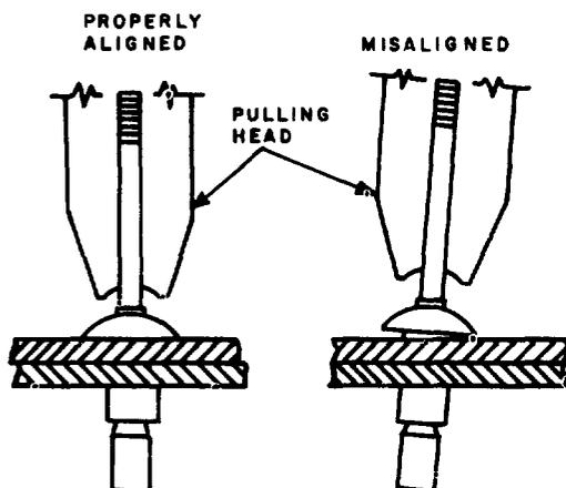
Fig. 2—Pulling Head Placement
