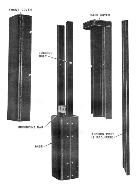
*USE:* To enclose aboveground splices in buried PIC cable and control and access points in dedicated buried plant.
