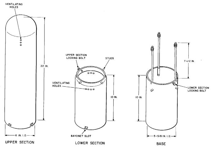
USE: For aboveground splices in PIC cable and for control and access points in dedicated plant with 200 OUT pairs. Can be made gastight or nongastight. Recommended for cables with paper or pulp insulation, at loading points, or at junction splices where rearrangements and changes are anticipated.
