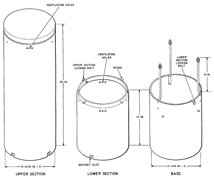
USE: For aboveground splices in PIC cable and for control and access points in dedicated plant with 400 OUT pairs. Can be made gastight or nongastight. Recommended for cables with paper or pulp insulation, at loading points, or at junction splices where rearrangements and changes are anticipated.
