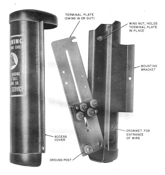
USE: To terminate, splice, and load buried wire.
