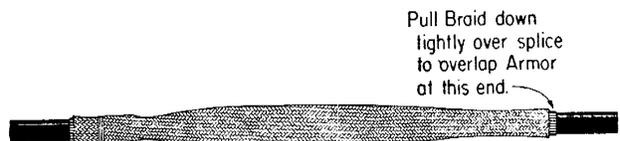
5.03 Using the carding brush, lightly scour the jacket for about 2 inches beyond the armor at each end of the splice. Then, starting about 2 inches beyond the lashed end of the braid, apply two half-lapped wrappings of 3/4-inch DR Tape over the jacket and braid. As the first wrapping progresses, the braid will elongate under the tape. When this wrapping has been carried to about 1-1/2 inches from the free end of the braid, lash the braid as in 5.02 (2). Complete the tape wrapping, as shown.
