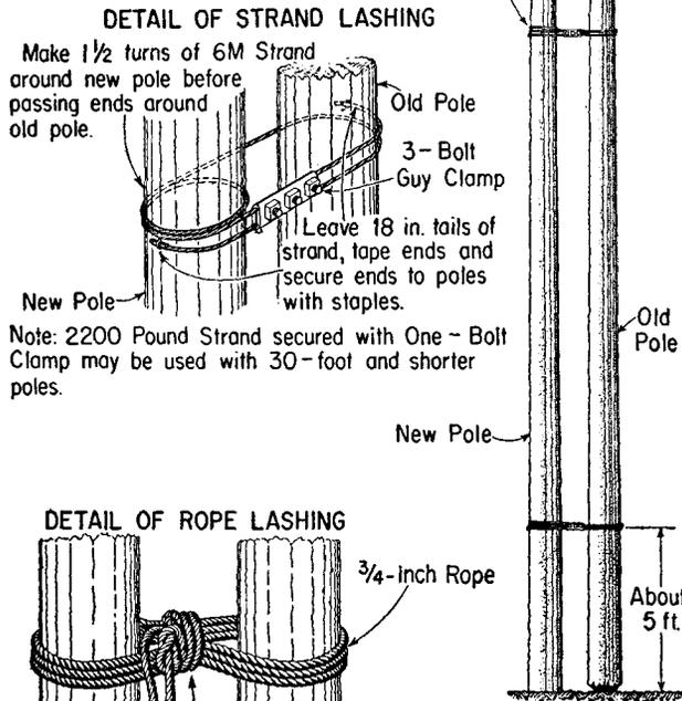
3.03 In order to place the upper lashing, climb the new pole. Do not, under any circumstances, work from the old pole until both upper and lower lashings have been completed. Rope lashings should be used only where the old pole is to be removed within a reasonable period of time (usually a few days) or where there might otherwise be an electrical hazard in passing the sling around the poles.
