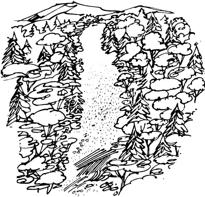
Figure 2. Deflect right-of-way strips.
