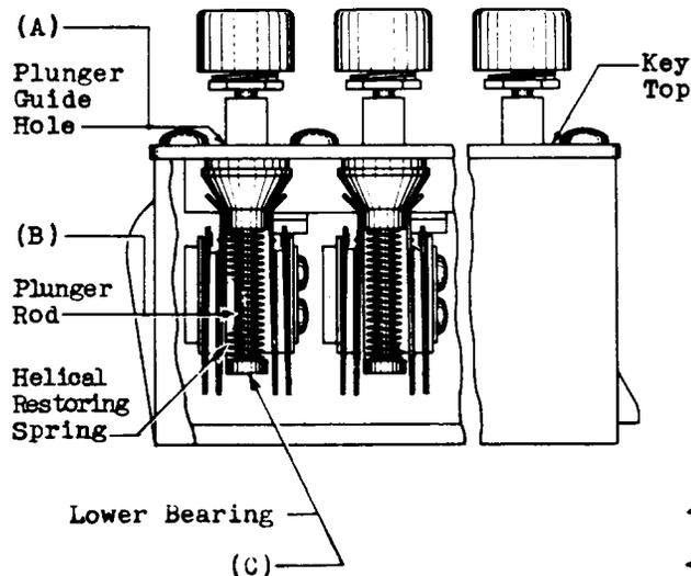
Fig. 1 - Lubrication Points of 499-, 523-, and 524-type Keys
