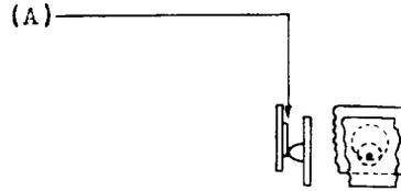
Fig. 3 - Contact Alignment Showing Maximum Permissible Misalignment
