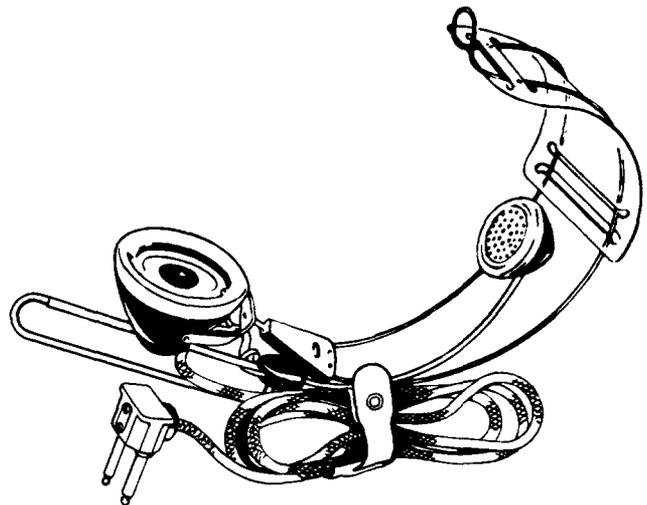
**Fig. 2(B) – Cord Equipped With the No. 396A Plug**
