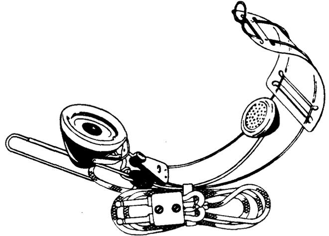
**Fig. 2(A) – Cord Equipped With the 289-Type Plug**
