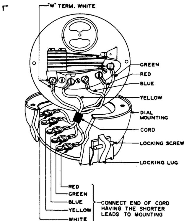
**Fig. 1 – Method of Cording Dial Mountings and Dial, Using D5AD or D5AH Cord With Dial Having a W Terminal As a Part of the Contact Spring Assembly (D5AD Cord Illustrated).**
