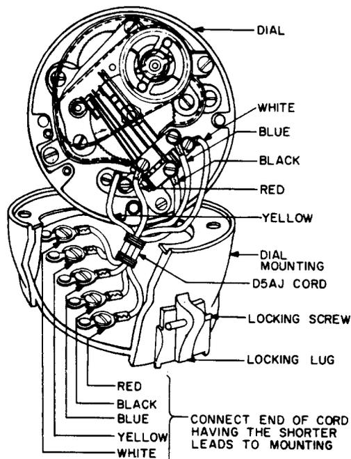
**Fig. 3 - Method of Cording Dial Mountings and Dial, Using D5AJ Cord, With Dials Having All Dial Terminals Part of the Spring Assembly**
