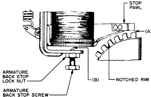
**Fig. 7 – Vertical Position of Stop Unit (203C, D and 208-Type Selectors)**
