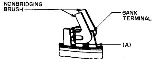
Fig. 29 - Clearance Between Rotor Brushes and Bank Terminals
