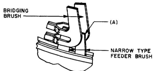
Fig. 30 - Clearance Between Rotor Brushes and Bank Terminals
