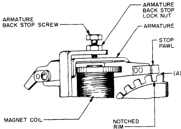
**Fig. 8 - Position of Armature Back Stop (202-Type, 203A, B, E, and 207-Type Selectors)**
