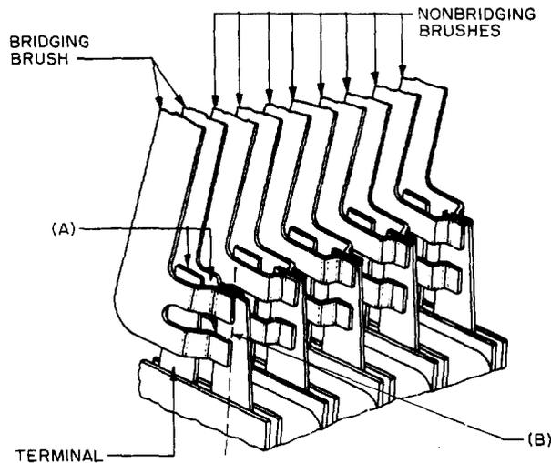
**Fig. 14 – Position of Rotor Brushes**
