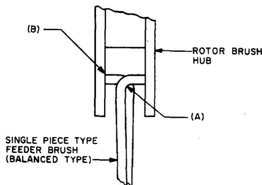
**Fig. 23 – Single-Piece-Type (balanced type) Feeder Brush Tension**
