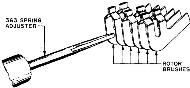
Fig. 34 – Method of Adjusting for Heel Spacing and False Contacting
