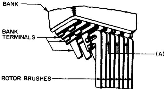
Fig. 27 - Rotor Brush Heel Spacing
