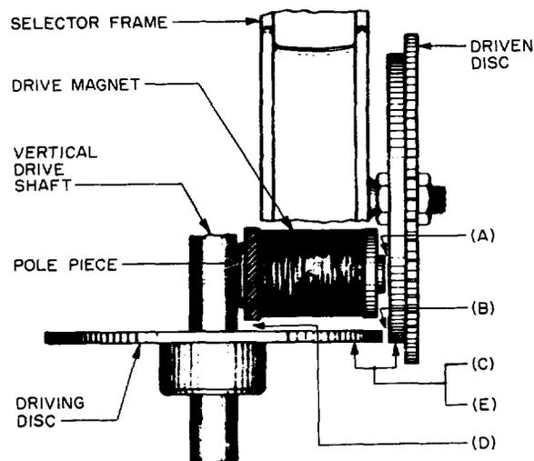
Fig. 5 - Relation Between Driving and Driven Disc
