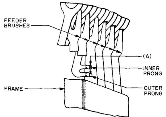
Fig. 25 - Relation Between Rotor Brush and Feeder Brushes
