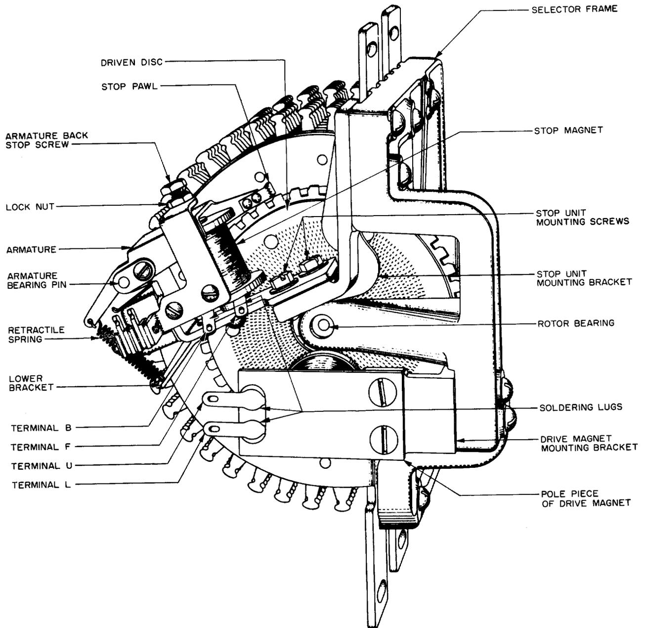
Fig. 2 - Side View of Selector
