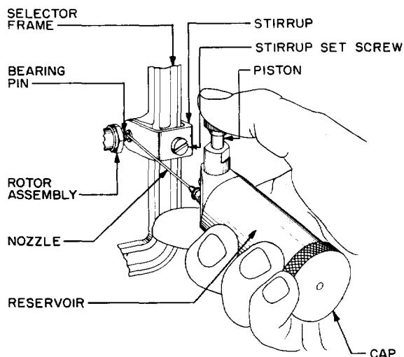
**Fig. 31 – Method of Using the 353C Grease Gun**
