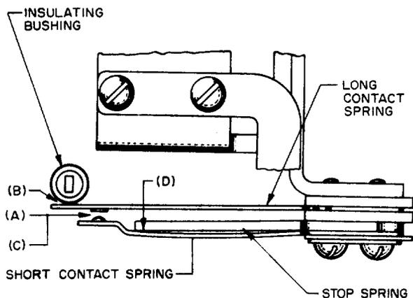
Fig. 12 - Stop Unit Spring Assembly
