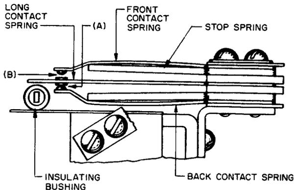
Fig. 11 - Stop Unit Spring Assembly
