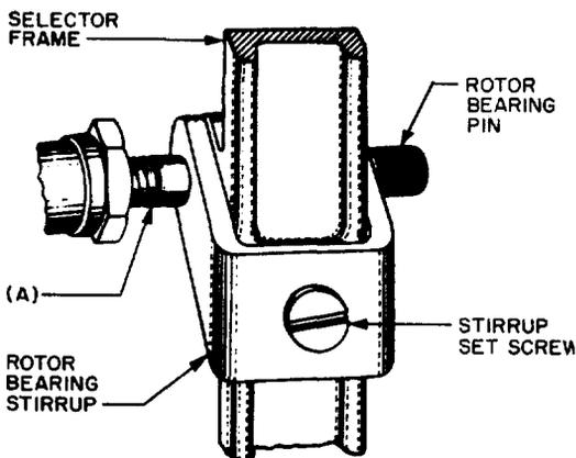
**Fig 3 – Rotor Bearing**
