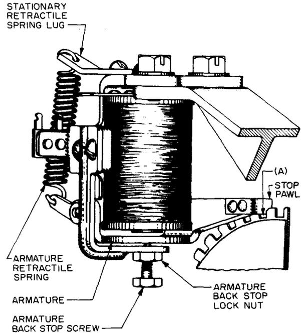
**Fig. 15 – Armature Retractable Spring**
