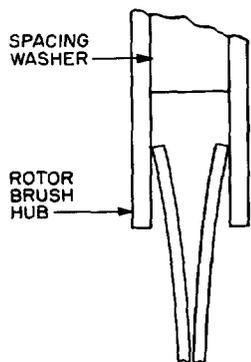
Fig. 20 - Two-Piece-Type Feeder Brush
