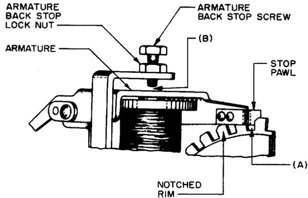
**Fig. 6 – Vertical Position of Stop Unit (202-Type, 203A, B, E and 207-Type Selectors)**
