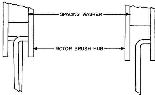
**Fig. 19a - Single-Piece Type Feeder Brush — Balanced Type With Two Formed Tips**
