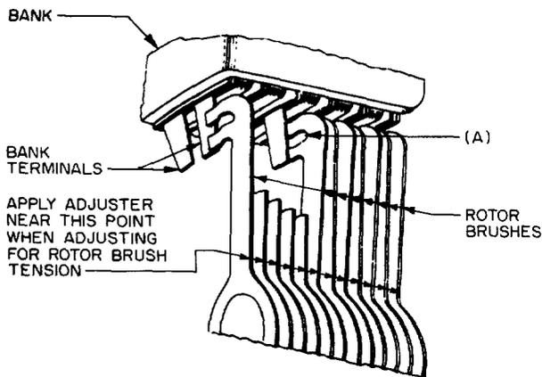
Fig. 24 - Rotor Brush Assembly
