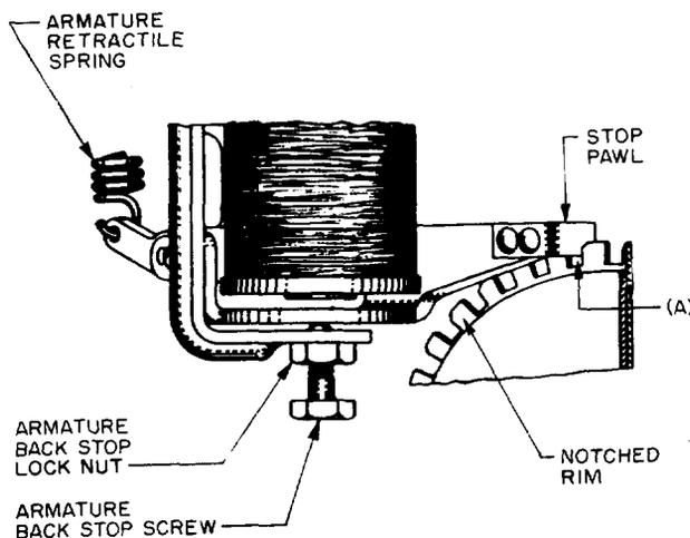
**Fig. 9 - Position of Armature Back Stop (203C, D and 208-Type Selectors)**
