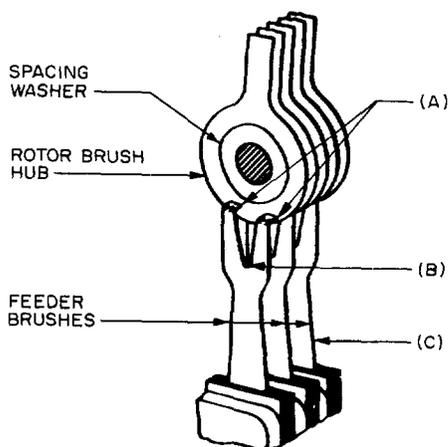
Fig. 21 - Rotor and Feeder Brushes
