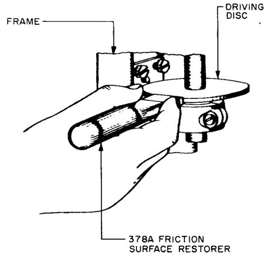
Fig. 32 - Method of Using 378A Friction Surface Restorer
