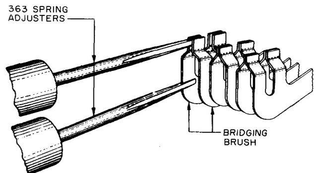
**Fig. 33 – Method of Adjusting Toeing of Bridging Brushes**
