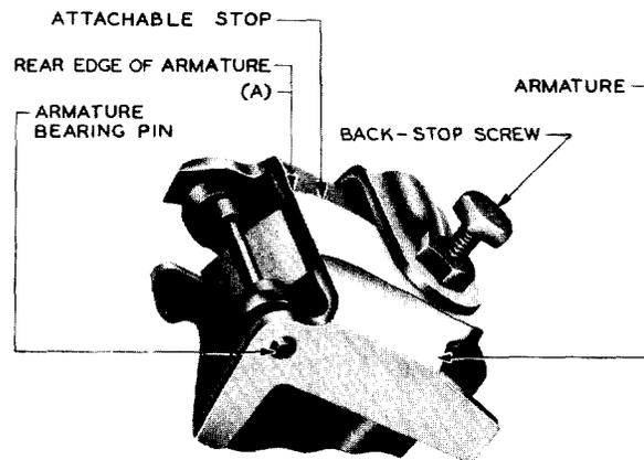
Fig. 35 – P-10A768 Attachable Stop Mounted on Armature of Stop Magnet
