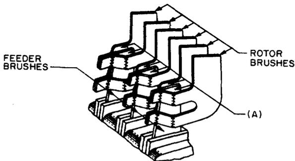
Fig. 28 - Rotor Brush Heel Spacing
