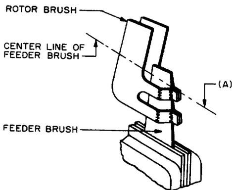
**Fig. 17 - Rotor Brush Alignment**
