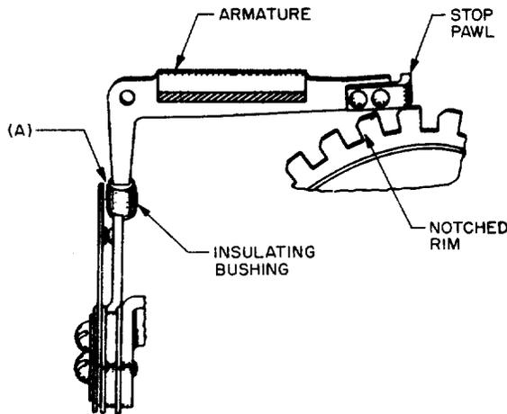
Fig. 13 - Armature Position
