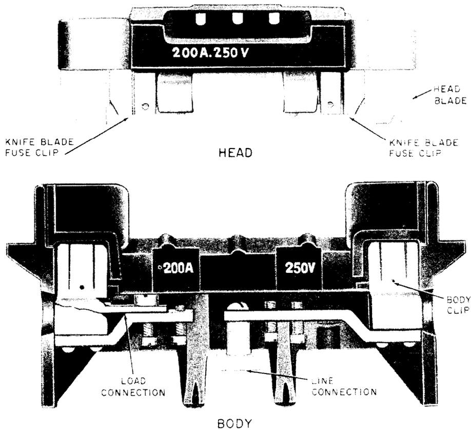
Fig. 2—200-Ampere SAFTOFUSE Unit—Sectional View
