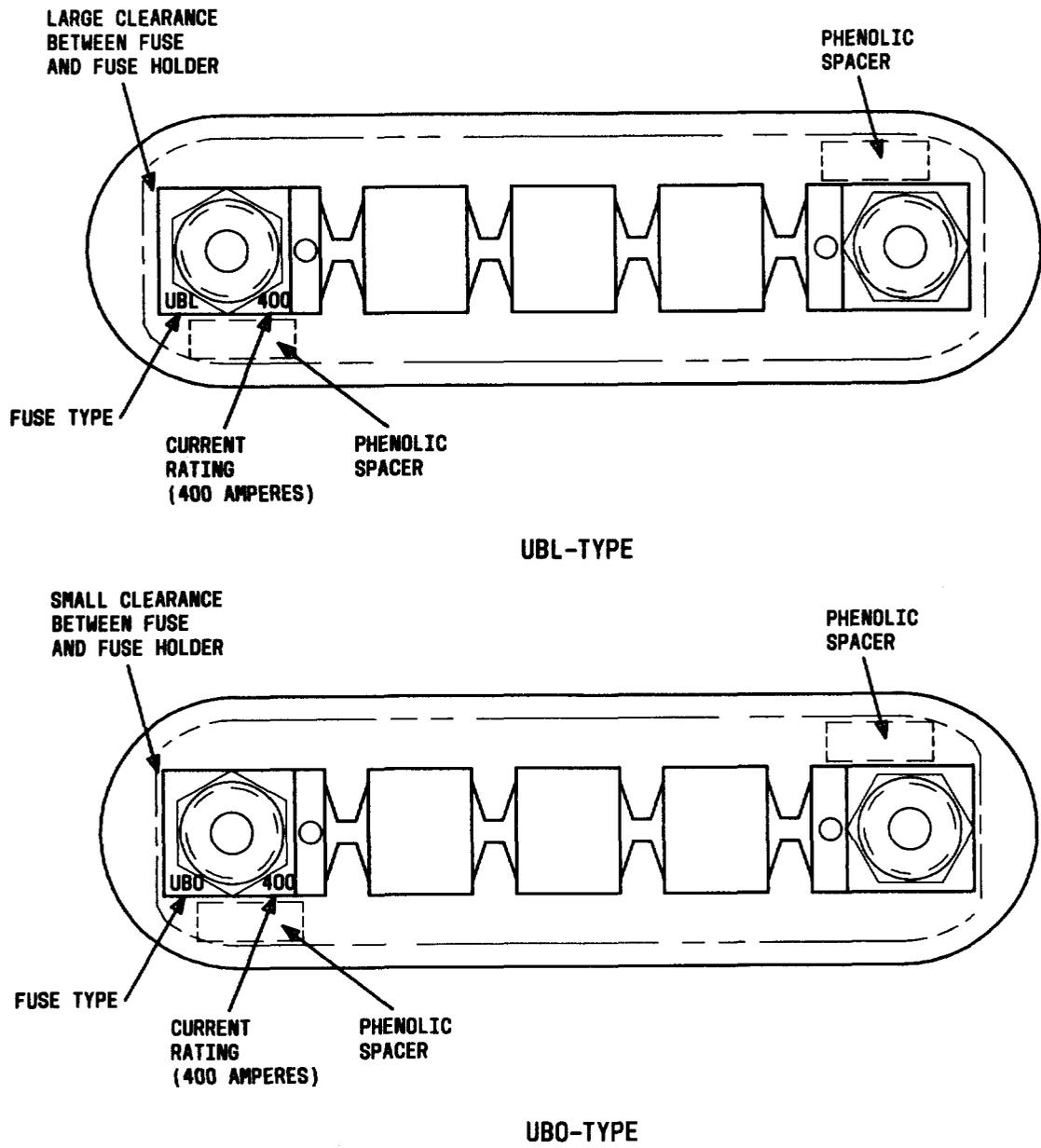
Fig. 4—KS-19392, L12 Through L16 (UBL- and UBO-Type Link Fuse) Blocking Point
