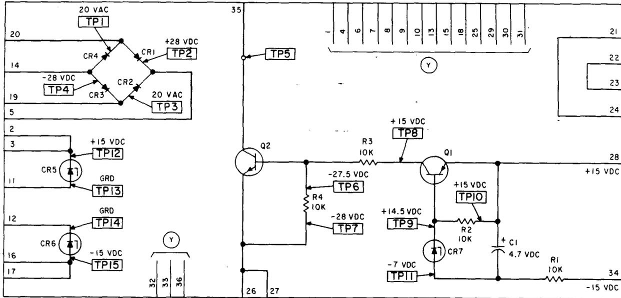
NOTE: VOLTAGES GIVEN ARE TYPICAL WITH RESPECT TO GROUND — RECTIFIER ON, NORMAL OPERATION (Y) KS-20618, L9 ONLY
