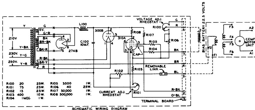
tends to diminish, the grid bias on the regulator amplifier tube increases and reduces the plate current. This increases the voltage drop across the amplifier tube which decreases the negative grid bias on the series tube, decreases its resistance, and raises the output voltage of the rectifier. This increases the output of the generator (par. 1.03) to bring the charging current back to the regulated value. An increase in charging current would have the opposite effect.
