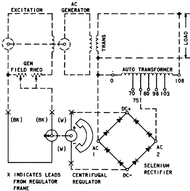
Fig. 7—KS-5376-01 L11 A-C Regulator With Input
