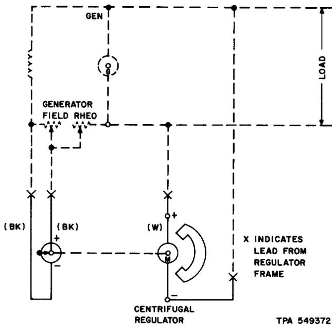
Fig. 6—KS-5293-02 L3 D-C Regulator With Input
