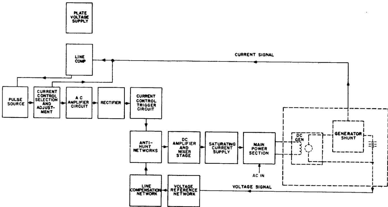
Fig. 3 — Block Diagram — J86250A Voltage Regulator and Exciter
