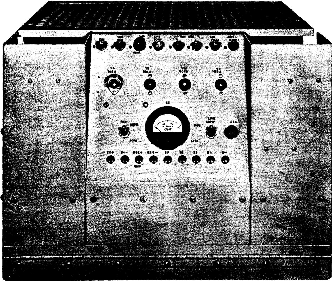
Fig. 1 — J86250A Voltage Regulator and Exciter (early model shown without tubes)
