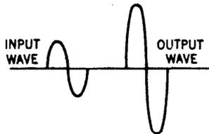
Fig. 5 – Comparison of Input and Output Waveshape (Distortion)
