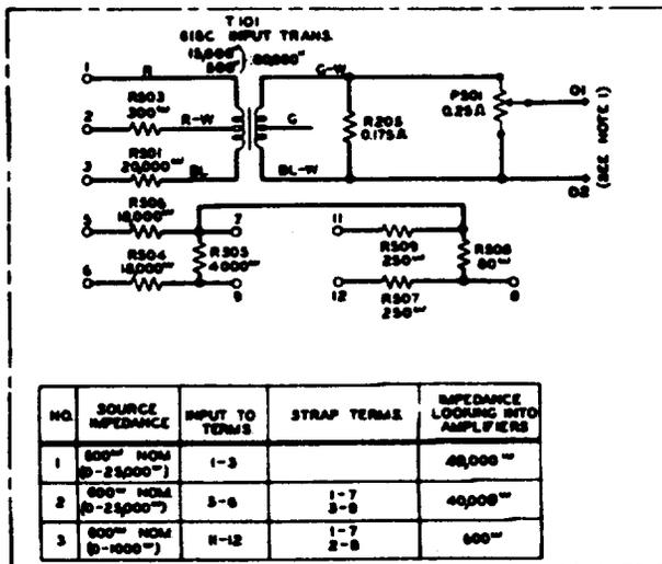
NOTE 1: IN THE 124E AMPLIFIER, 01 AND 02 ARE WIRED TO 21 AND 22 (SHOWN ON SCHEMATIC OF 124B AMPLIFIER) RESPECTIVELY. THESE DESIGNATIONS ARE FOR REFERENCE ONLY AND DO NOT APPEAR ON THE AMPLIFIER.
