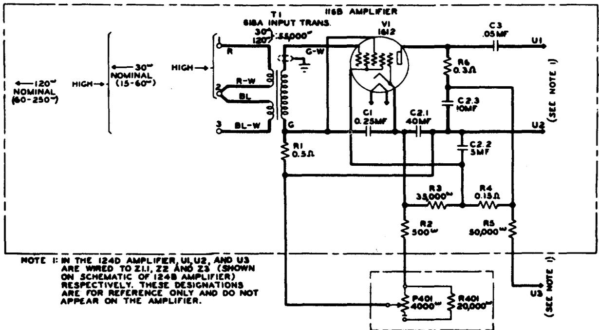
Fig. 6 - 124D Amplifier - Input Arrangement
