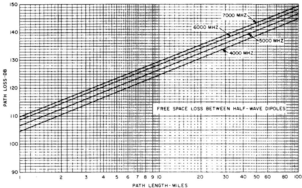
Fig. 4—Free Space Loss Between Half-Wave Dipoles
