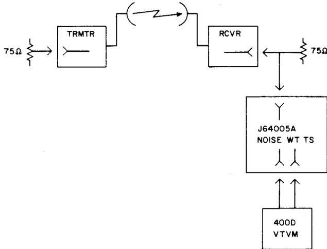
Fig. 12—Test Layout, Random Noise Measurement
