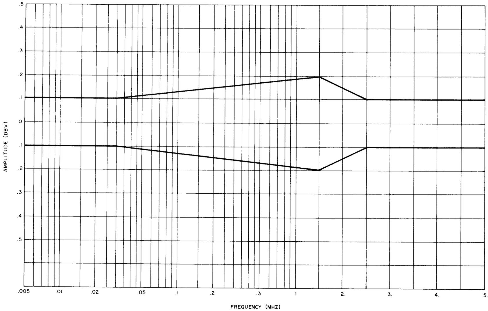
Fig. 8—Amplitude-VS-Frequency Response for Local Loops
