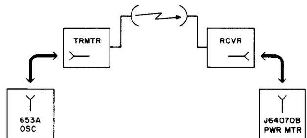
**Fig. 9—Test Layout, Point-To-Point Gain Frequency Measurement**
