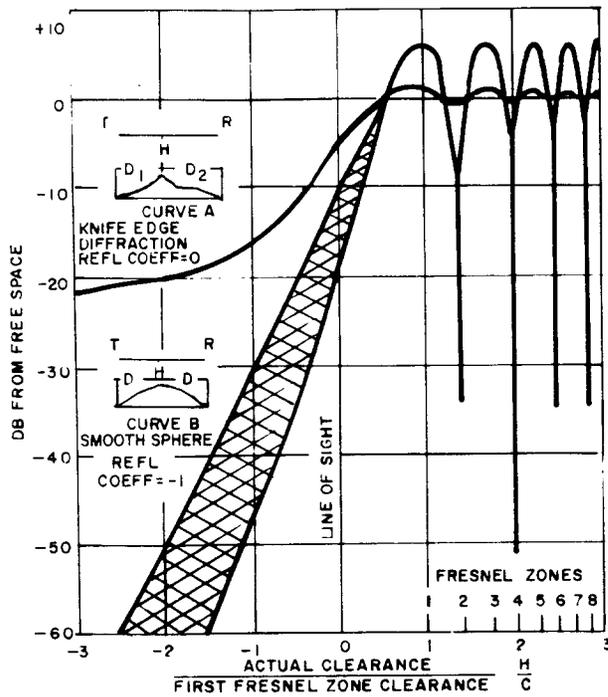
Fig. 7—Effect of Clearance on Radio Transmission
