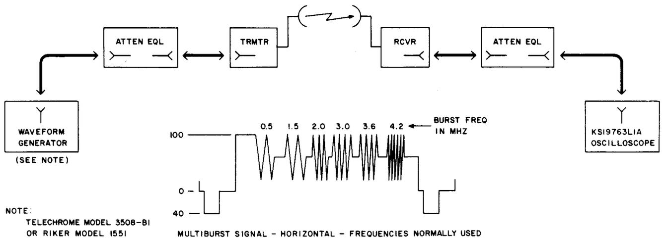
Fig. 13—Test Layout—Multiburst and Window Signal Measurement
