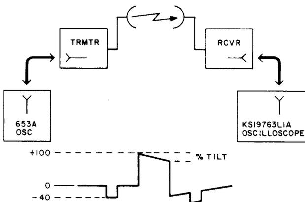
Fig. 11—Test Layout, 60 Hz Square Wave Frequency Response Measurement
