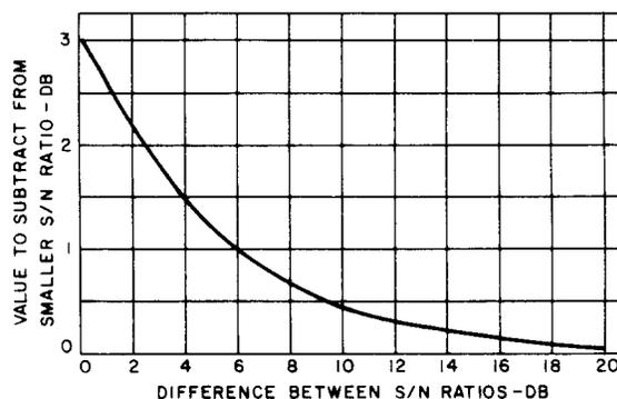
TO COMBINE ANY NUMBER OF S/N RATIOS, SUBTRACT THE LOWEST VALUE OF S/N FROM ONE OF THE VALUES TO BE COMBINED AND READ FROM THE CURVE THE VALUE CORRESPONDING TO THIS DIFFERENCE. SUBTRACT THIS VALUE FROM THE LOWEST S/N. USING THIS NEW S/N, FIND THE DIFFERENCE BETWEEN IT AND ONE OF THE REMAINING S/N VALUES, AND AGAIN SUBTRACT THE APPROPRIATE VALUE OBTAINED FROM THE CURVE. CONTINUE THIS PROCESS UNTIL ALL OF THE S/N VALUES HAVE BEEN COMBINED.
