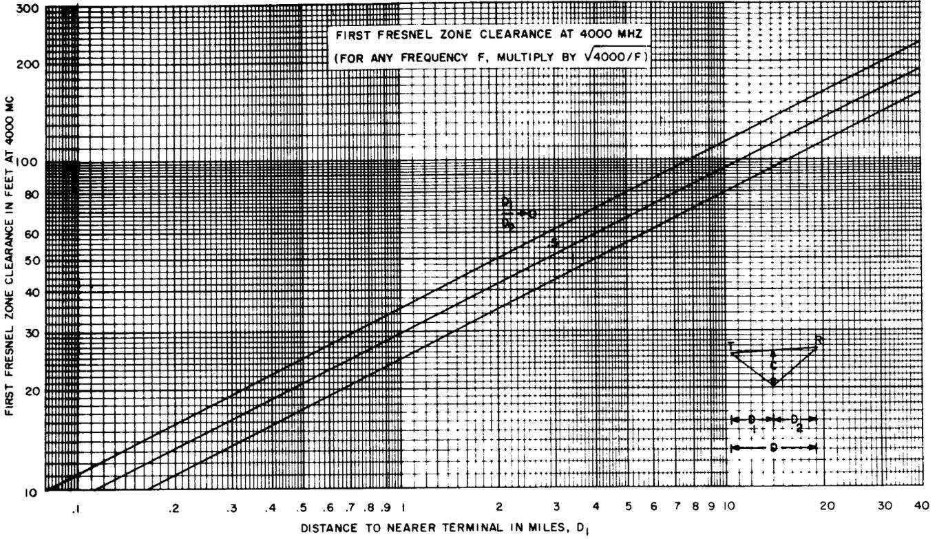
Fig. 6—First Fresnel Zone Clearance at 4000 MHz
