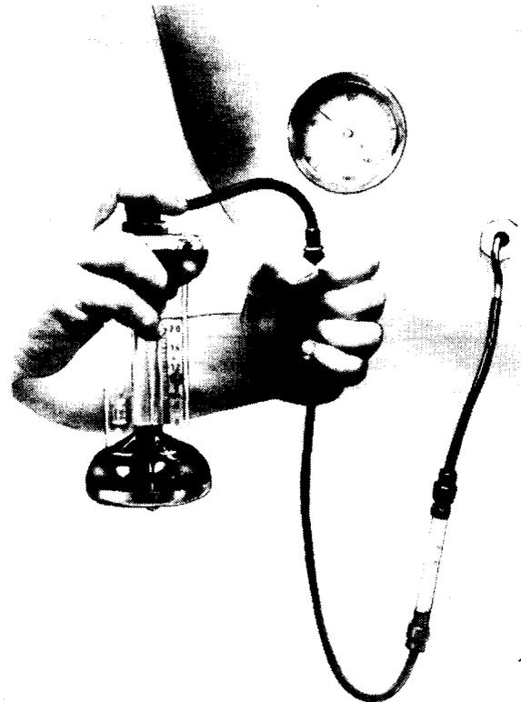
Fig. 6—Taking a Flue Gas Sample
