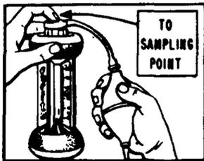
Push rubber connector down-then squeeze bulb 18 times.
