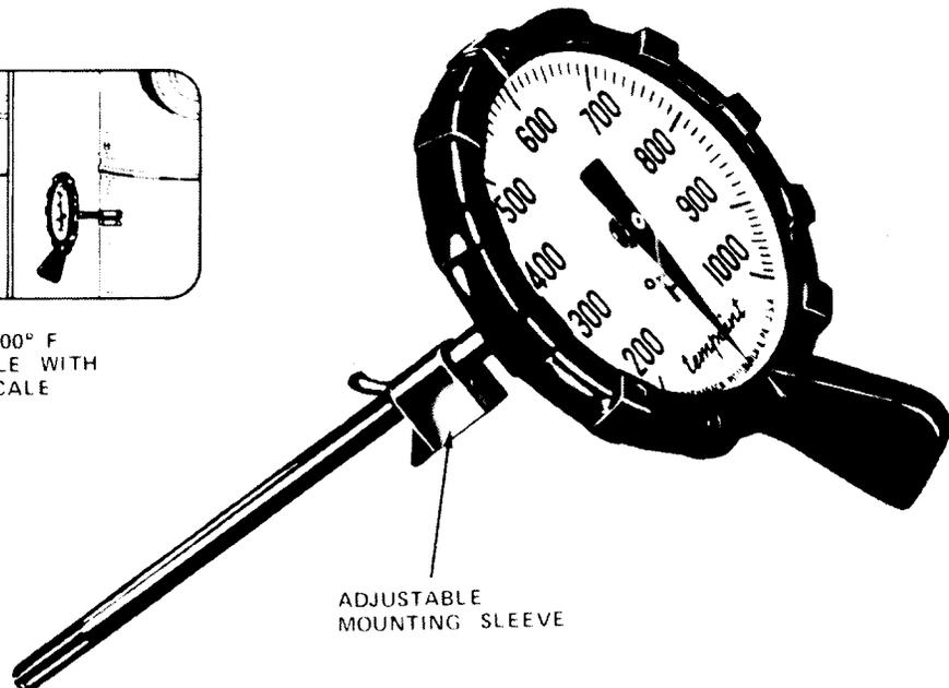
Fig. 3—Testing Stack Temperature
