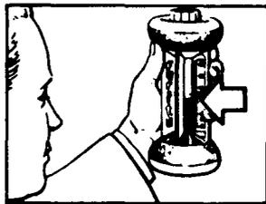
Read fluid level on CO<sub>2</sub> scale
