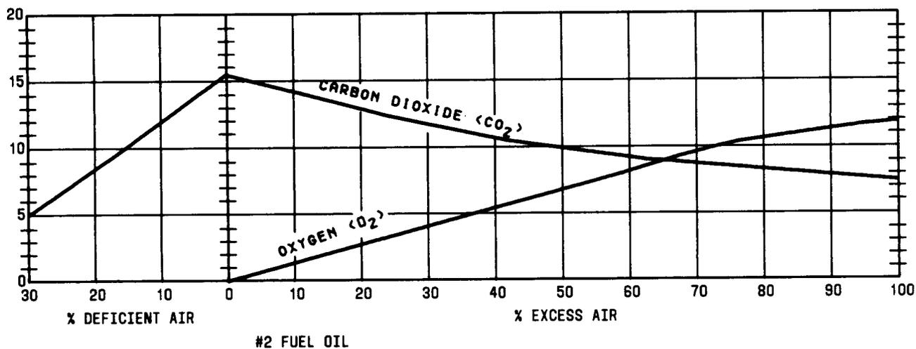
Fig. 9—Percent of Excess Air for Various CO<sub>2</sub> and Oxygen Readings
