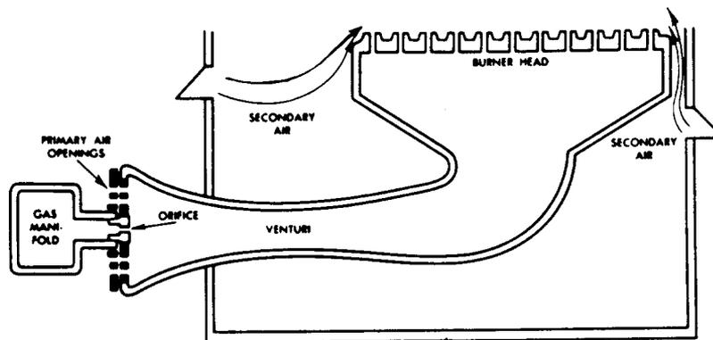
Fig. 14—Typical Atmospheric Burner
