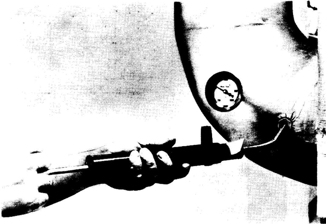
**Fig. 11—Taking a Smoke Sample**
