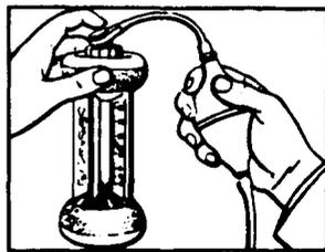
Lift finger from rubber connector-this seals FYRITE
