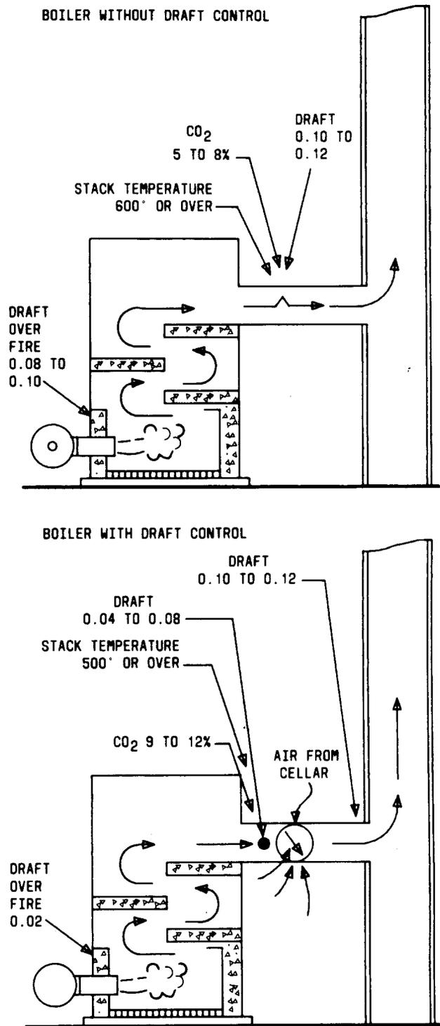
**Fig. 12—Draft Control Can Increase Operating Efficiency**
