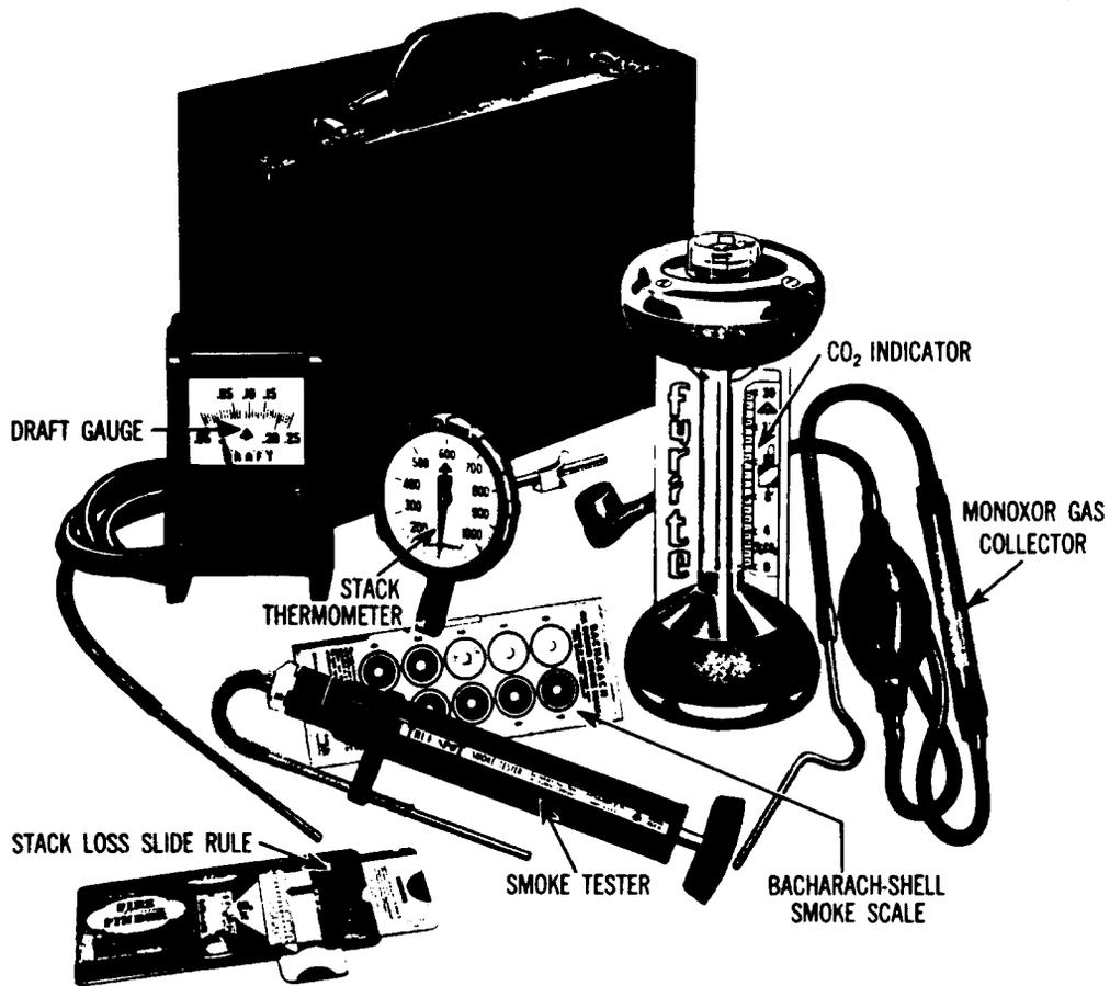
Fig. 1—Combustion Efficiency Testing Kit
