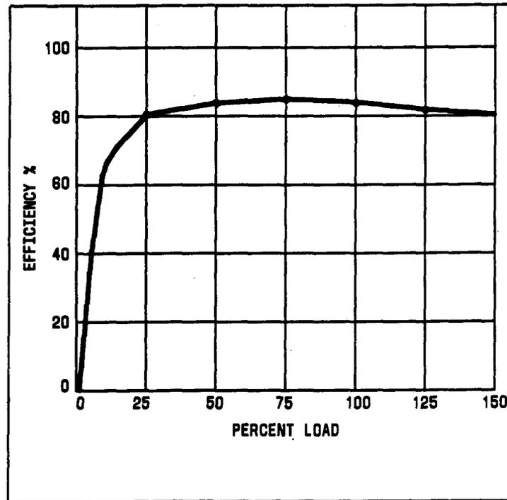
Fig. 1—Efficiency of Typical 3-Phase Motor
