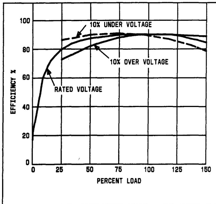
Fig. 2—Efficiency Sensitivity of Typical 3-Phase Motor
