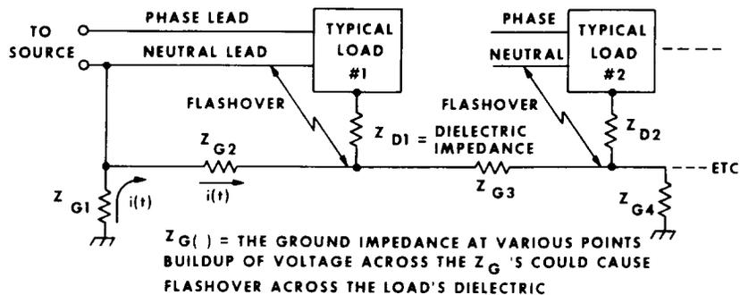
Fig. 4—Ground Impedance Effects
