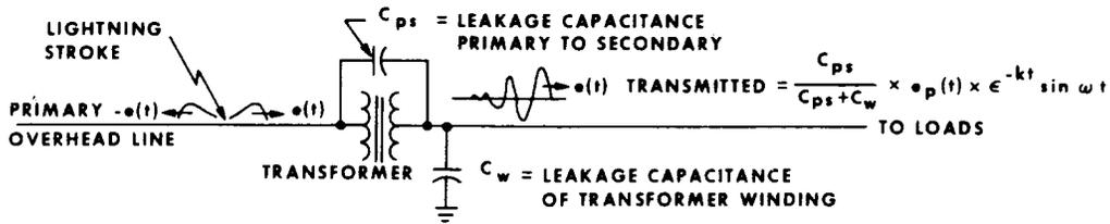
Fig. 2—Capacitive Coupling Effects
