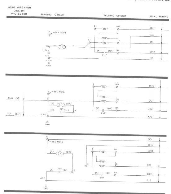
Nate: When an E terminal is not normally provided in subscriber sets, use D-161488 connector to connect local wiring to R ringer lead.
