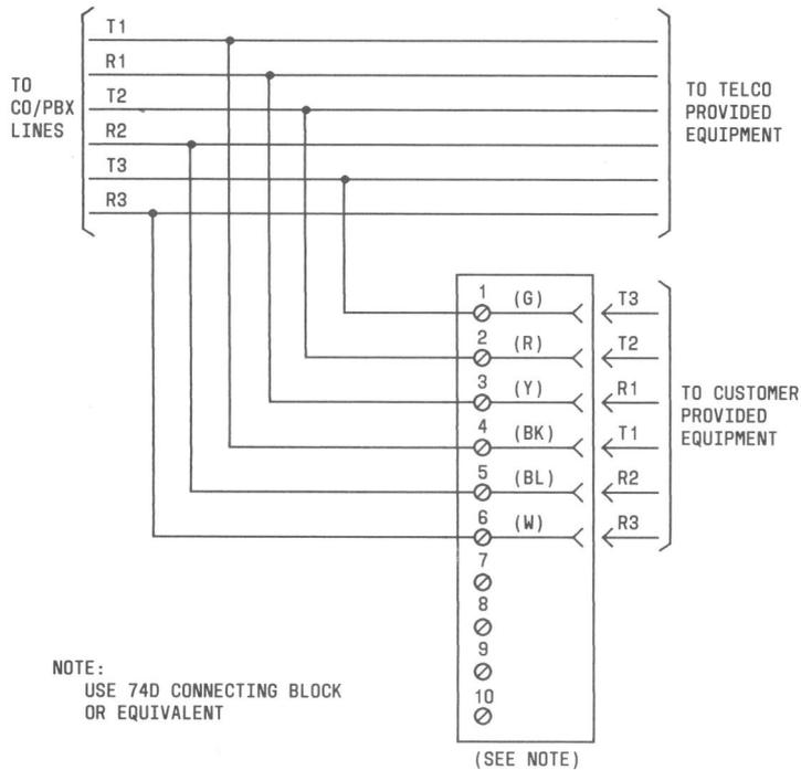
Fig. 2—Connections for USOC RJ25C
