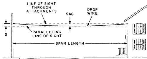
Fig. 1 - Drop Wire Attachments on Same Level
