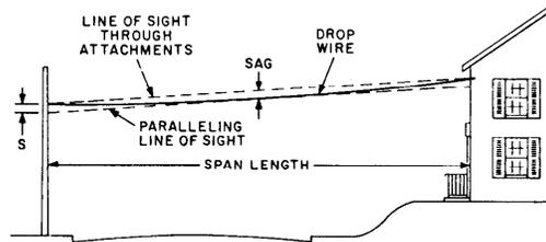
Fig. 2 - Drop Wire Attachments on Different Levels
