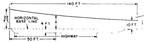
Fig. 6 - Height of pole and House Attachments Are Known
