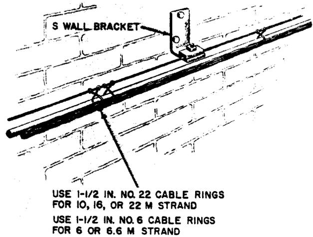
Fig. 7—Wire Run in Cable Rings Paralleling Cable Supported with Strand
