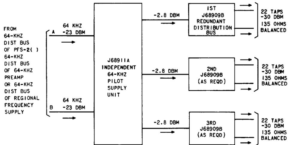
Fig. 2—Independent 64-kHz Supply and Distribution Circuit
