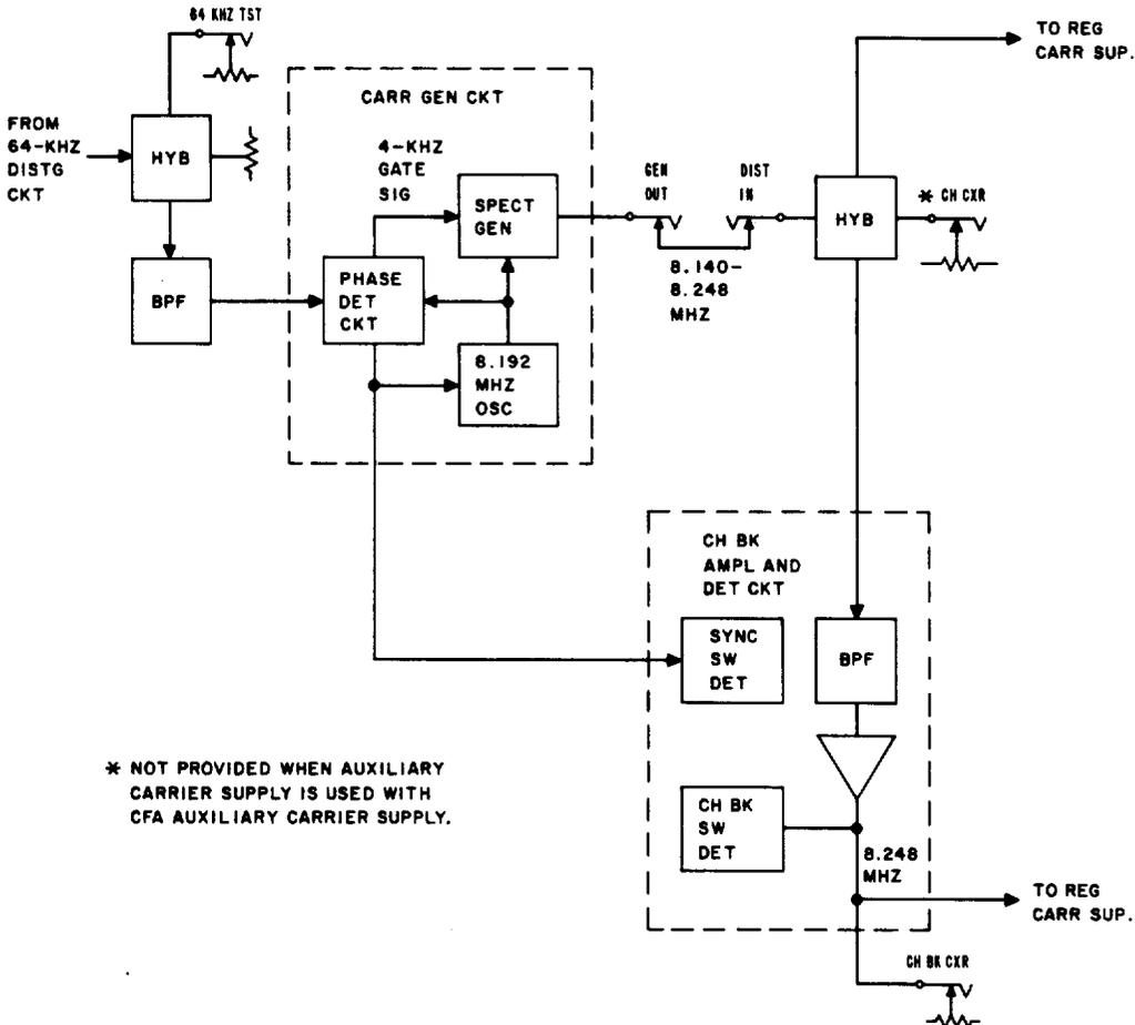
Fig. 4—A6 Auxiliary Carrier Supply
