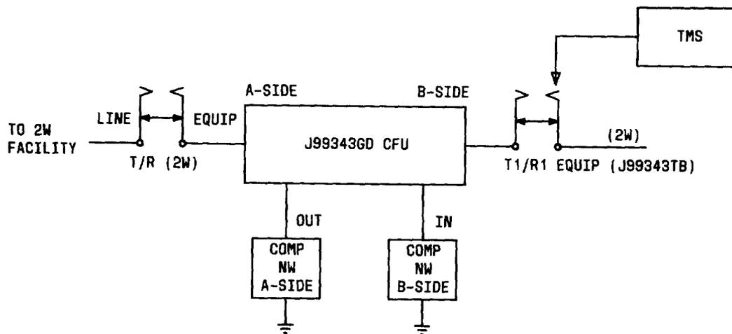
Fig. 3—Typical Test Configuration for Setting A-Side Gauge Switches
