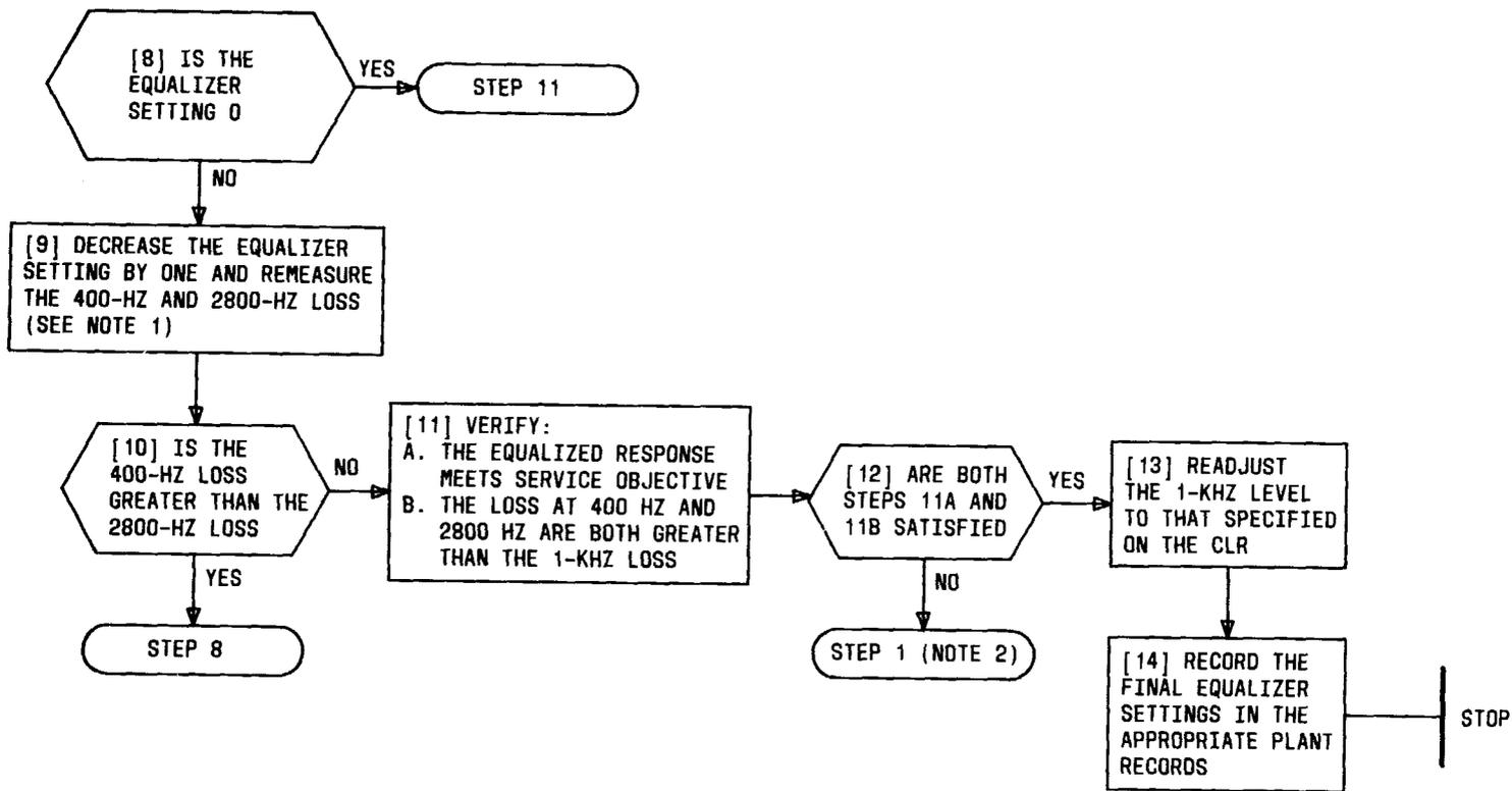
Chart 7—Procedure for Equalizer Touch-Up (Sheet 2 of 2)
