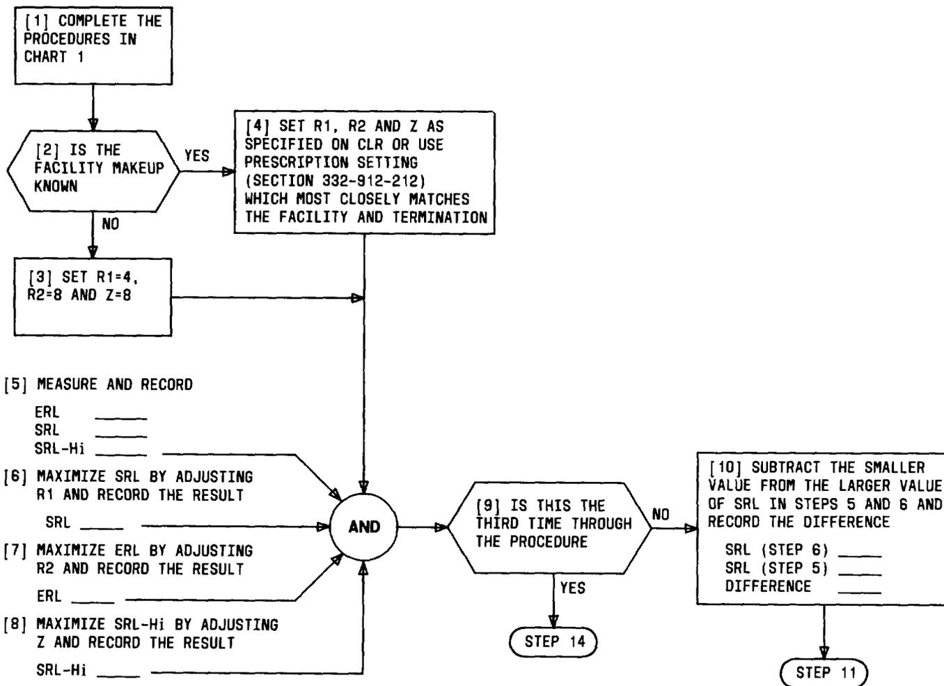
Chart 3—Procedures for Adjustment of the B-Side PBN (Sheet 1 of 2)
