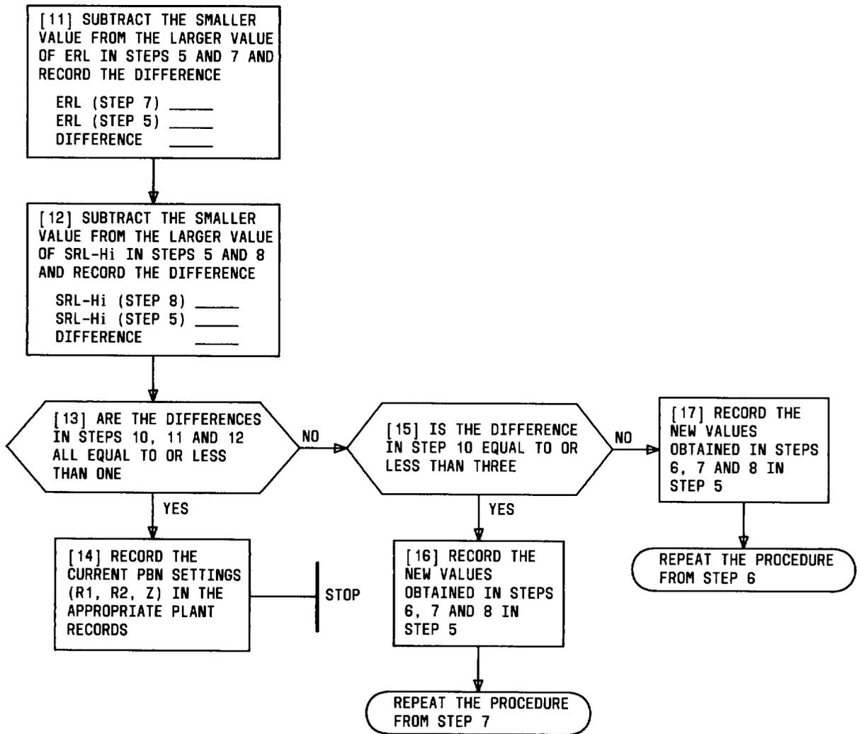
Chart 3—Procedures for Adjustment of the B-Side PBN (Sheet 2 of 2)
