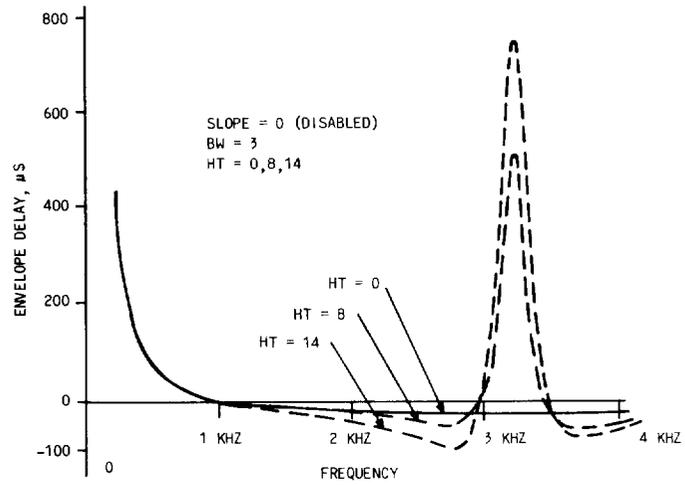
Fig. 14—Relative Envelope Delay Distortion of the SF Signaling/4-4 Wire Repeater, BW = Small Setting, HT Variable
