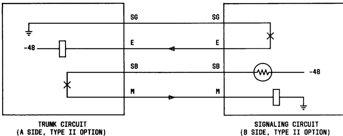
**Fig. 6—Type II E and M Interface**
