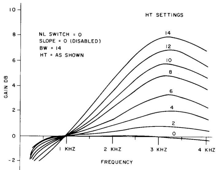
Fig. 11—Gain Frequency Response of the Equalizer Unit, BW = Large Setting, HT Variable
