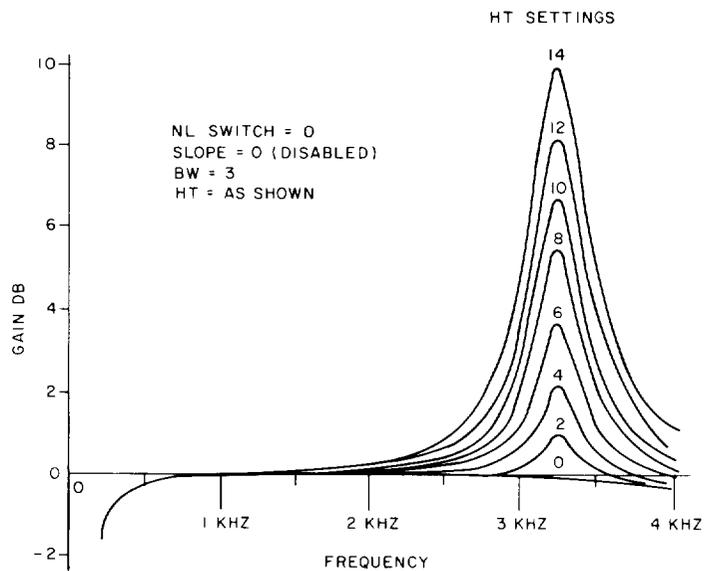
Fig. 10—Gain Frequency Response of the Equalizer Unit, BW = Small Setting, HT Variable
