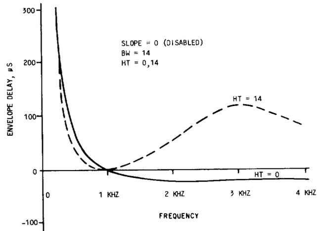
Fig. 15—Relative Envelope Delay Distortion of SF Signaling/4-4 Wire Repeater, BW = Large Setting, HT Variable
