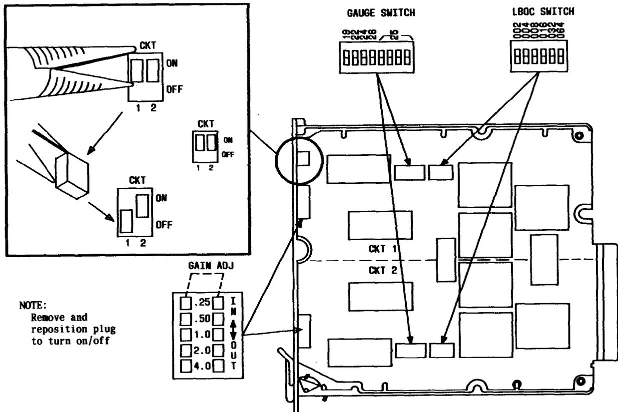
Fig. 3.1—Description of How to Operate the CKT 1,2 (ON/OFF) Plug-Switch of the J99343PL L2 Repeater
