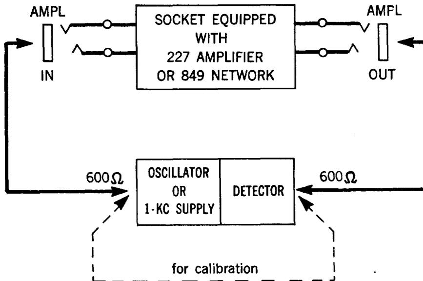
Fig. 7 - Gain or Loss Measurement at Amplifier Socket
