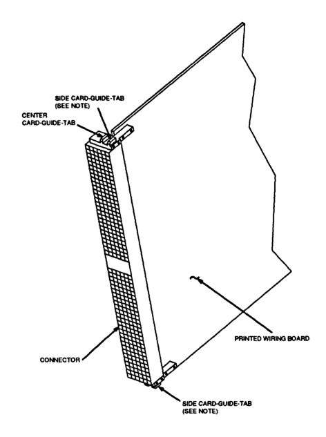
NOTE: Remove the side card guide tabs (both top and bottom) on older versions of circuit packs before inserting into a new apparatus housing equipped with the reduced-cost card guides. The side card guide tabs may be removed by filing the tabs flush with the top of the connector.
